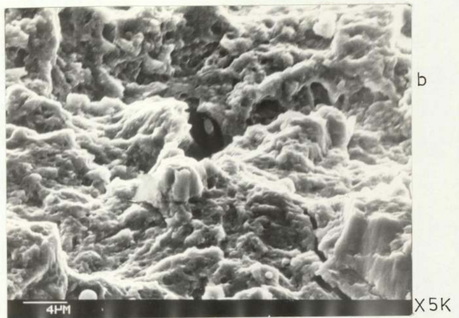
Fig. 76 S.E.M. fractographs of a Co-Mo alloy plated No.5 die steel fatigue testpiece showing void coalescence. (b) is a magnified view of (a) revealing some of the inclusions associated with the dimples.
