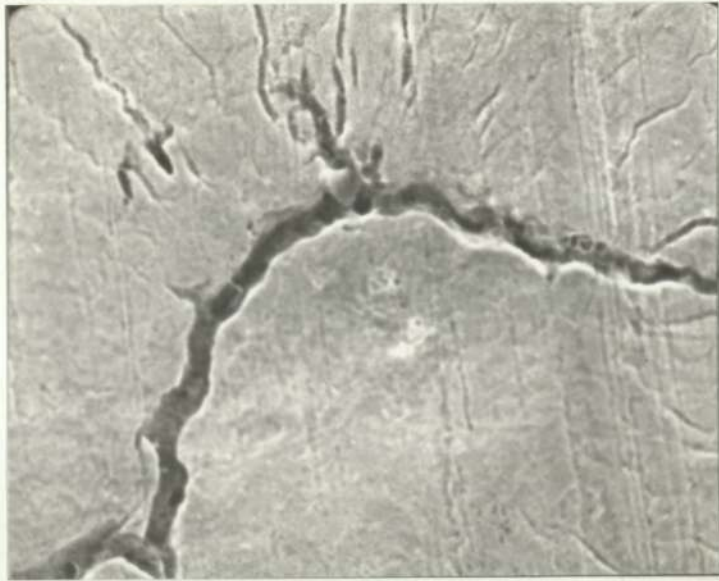
Fig. 19 Worn surface of a hardened and tempered No.5 die after 100 cycles hot forging showing
