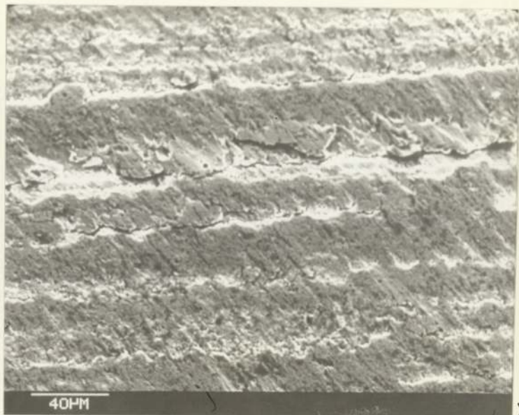
Fig. 44 A view of the surface of a plasma nitrided BH13 die after 100 cycles forging showing the effect of ploughing on a previously flattened layer, surface was descaled.
