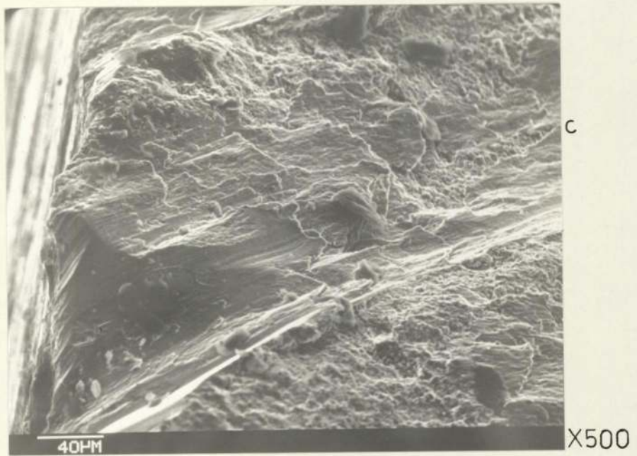
Fig. 64 Three views of the fracture surface of a hard Cr plated No.5 die steel impact testpiece showing - (a) the edge of the testpiece (b) a mixture of cleavage plus tearing (c) an enlargement of one of the tear ridges.
