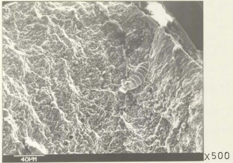
Fig. 82 S.E.M. fractograph of a hard Cr plated No.5 die steel fatigue testpiece showing a tear ridge and brittle failure at the coating-steel interface.
