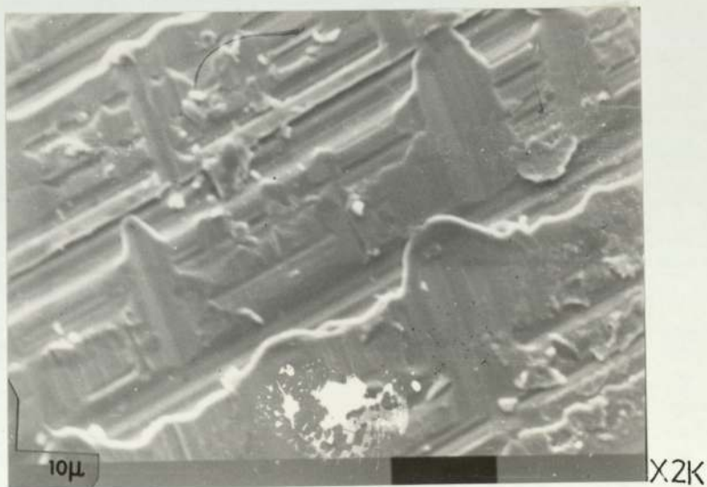
Fig. 14 Ploughing abrasion of a hardened and tempered No.5 die in the as-forged condition after 1 cycle hot forging.
