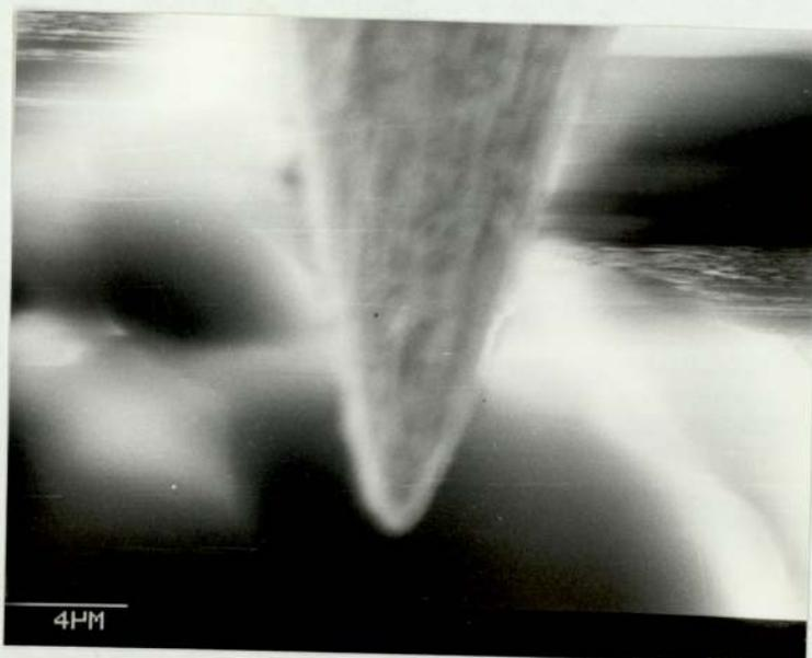
The incorporation of a  $1k\Omega$  resistor in the circuit ensures production of a conical shape of tip of similar angle with a lower current and a higher polishing time than that of series B and series C.
