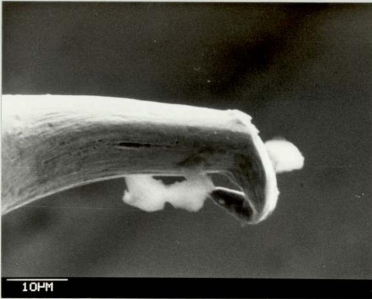
to 0.5 $\mu$ m diameter can be coated with carbon of a few nanometers in thickness. Such carbon coated microindenters can be hardened by heat treatment to diffuse the carbon into the tungsten to give tungsten carbide tips. These tips are harder than tungsten tips. The ductile tungsten supports the tungsten carbide coating and prevents the tips being too brittle to use. The tips are fragile and require very careful handling.
