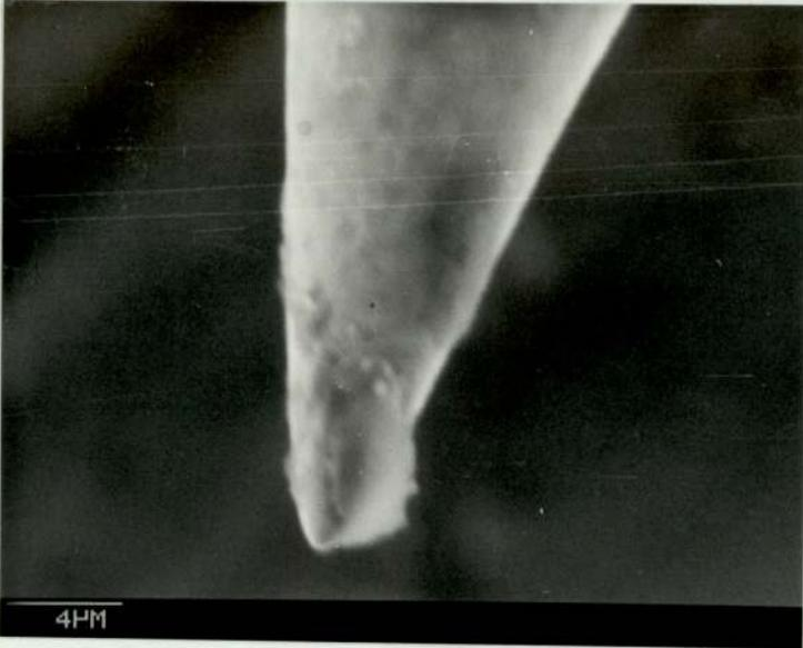
Microindenters polished from the tungsten wire of various thickness.
