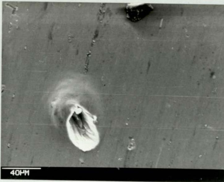
The microindentations with the micromanipulators probe needles at 5 gram indentation load on aluminium.
