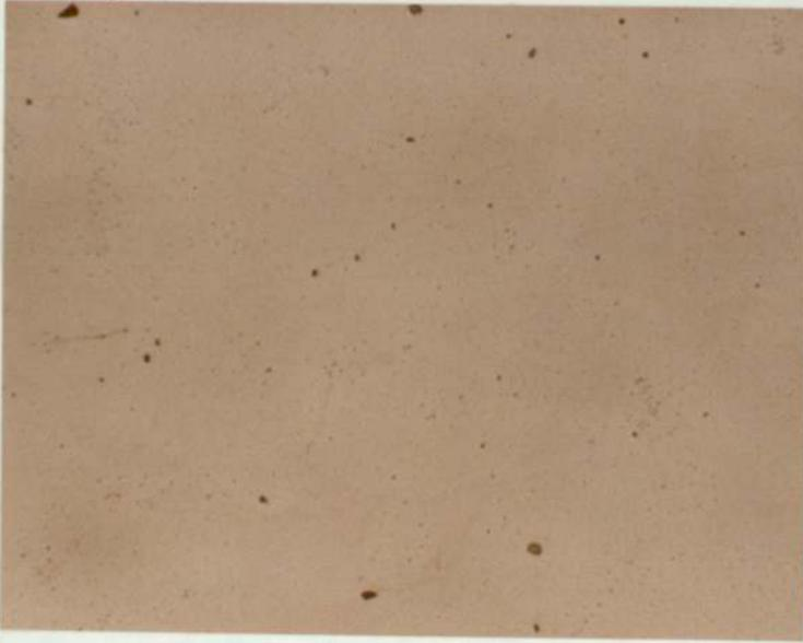
Au coating for 4 minutes of sputtering time on glass cover slips.
