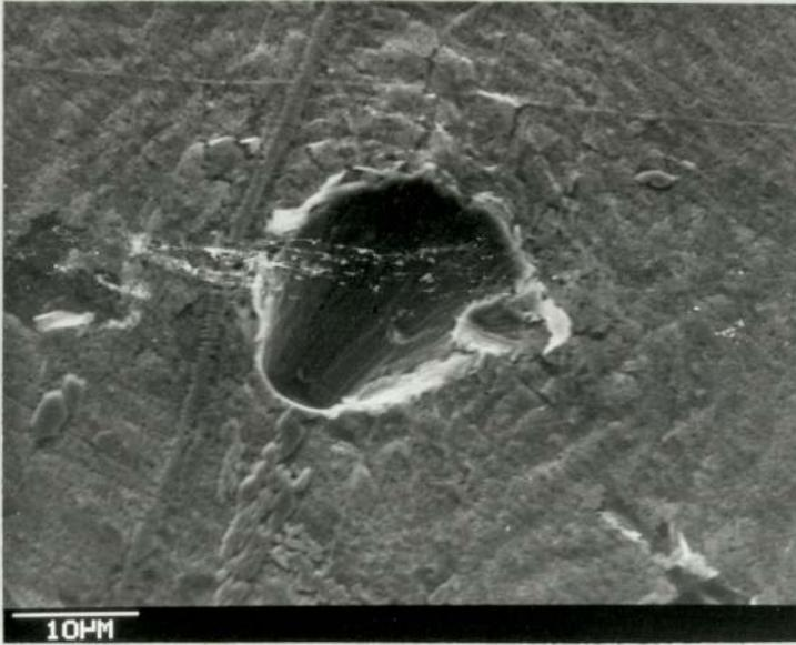
The microindentations made with the micromanipulator's probe needle at 3 gram indentation load on aluminium.
