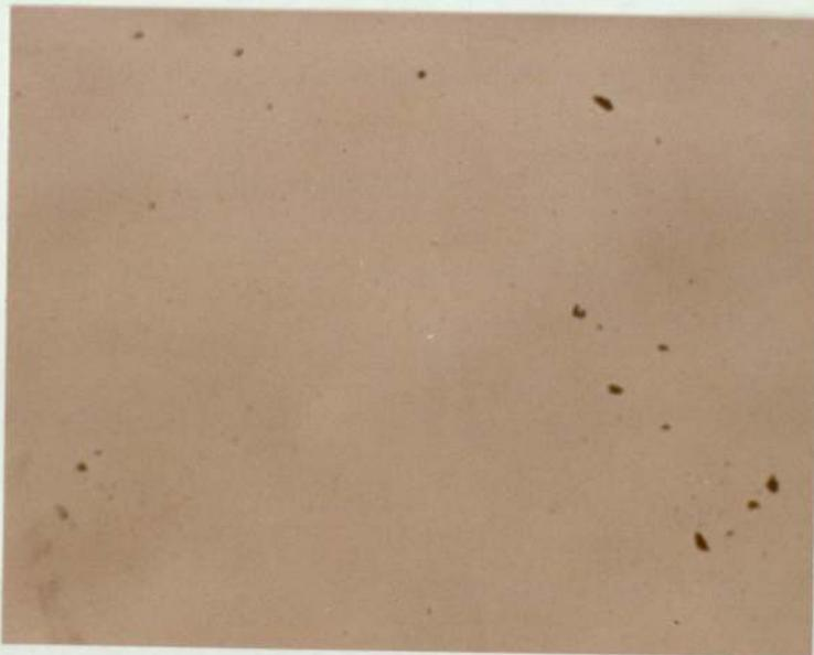
Gold coating for 3 minutes of sputtering time on glass cover slips.
