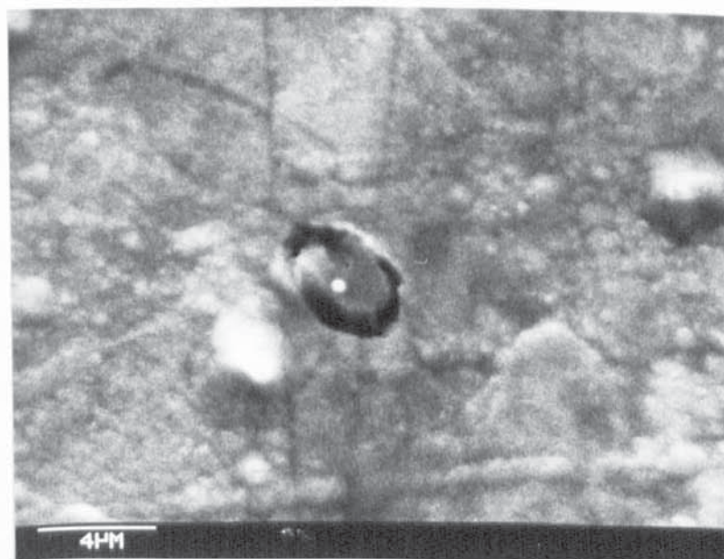
(b) : Ion beam etched surface, tensile specimen No. 3V, \bar{\epsilon}^p = 0.023 . Nucleation occurs at Al-S-Ca-Mn-Fe inclusions.
