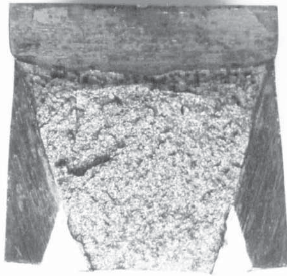
(a) : Side-grooved CVN specimen, -124^{\circ}\text{C}
