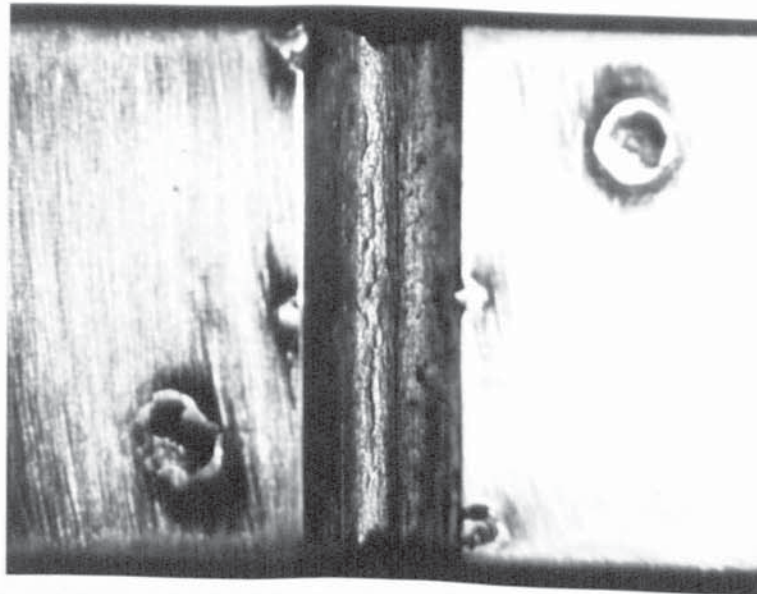
(b) : Side-grooved specimen, -98^{\circ}\text{C}
