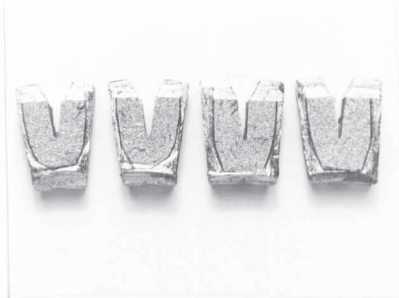
Plate 5.12 : Fracture surfaces in the mid-thickness section of the pre-cracked nonside- and side-grooved specimens; No. B19V (left), No. S19V (right).
