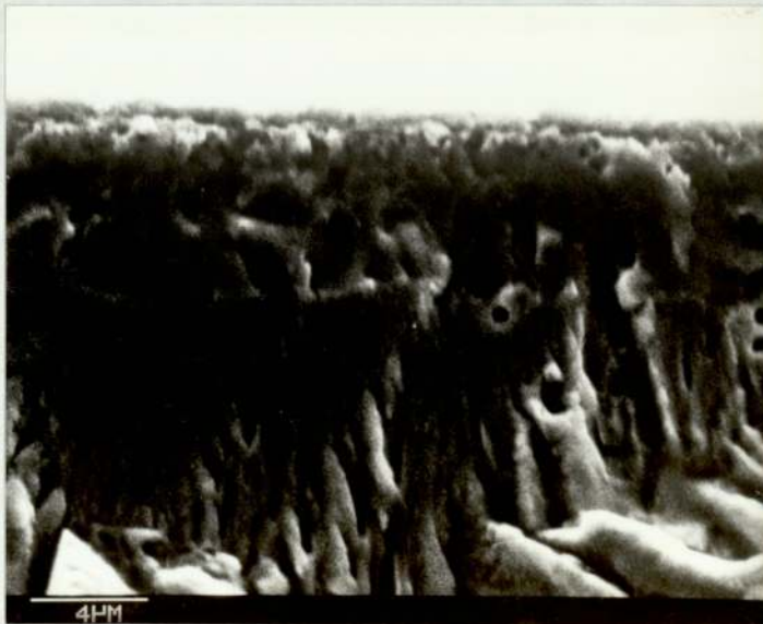
PLATE 63 Fatigue of compound layer at the notch root, nitrocarburised 080M15, root radius 3.17 mm, N_i = 191,000
