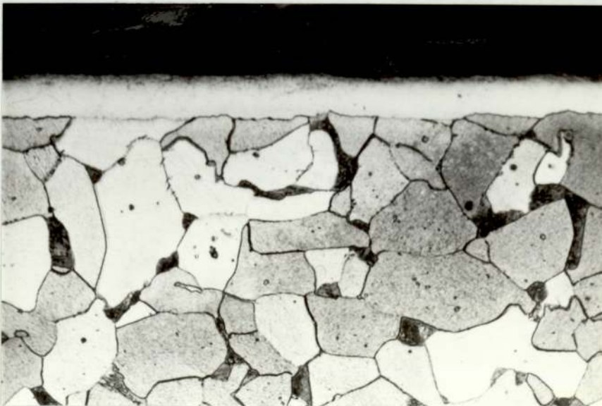
PLATE 22 Microstructure of nitrocarburised 080M15 specimen, midsection, at the notch root, root radius 3.17 mm (magnification x450)
