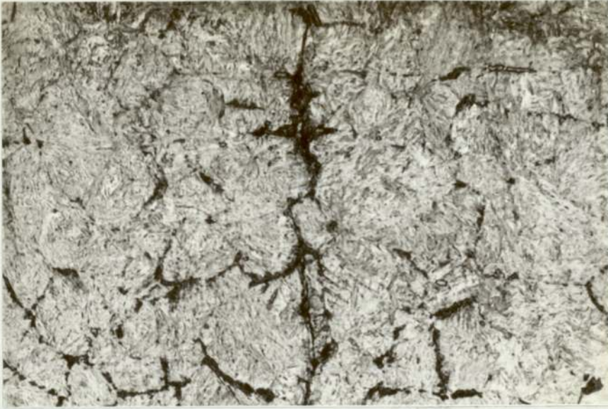
PLATE 19 Microstructure of carbonitrided 080M15, root radius 0.76 mm, (case depth 0.76 mm) (magnification x450)
