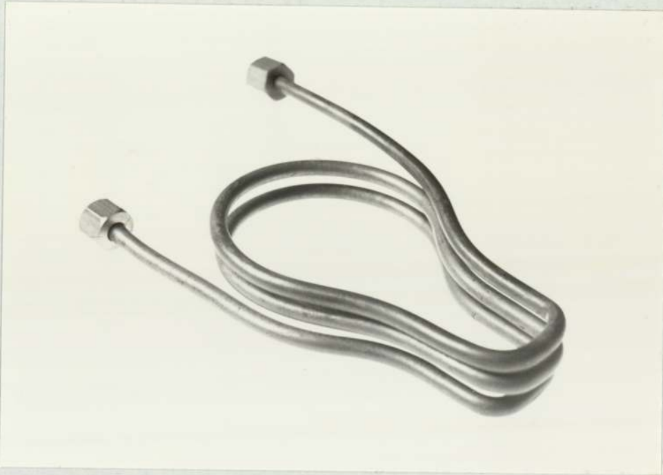
PLATE 1 Copper coil used for induction hardening
