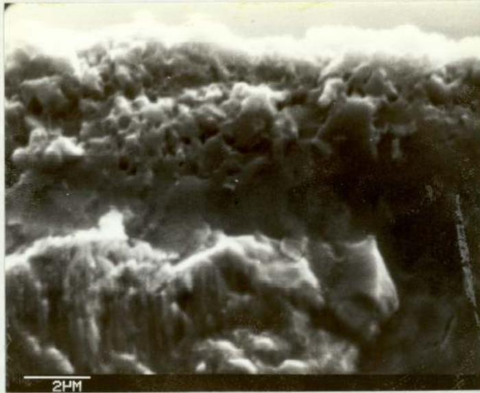
PLATE 58 Fatigue fracture in the compound layer at the notch root, showing microporosity, nitrocarburised 080M15, root radius 0.76 mm, N_i = 610,000
