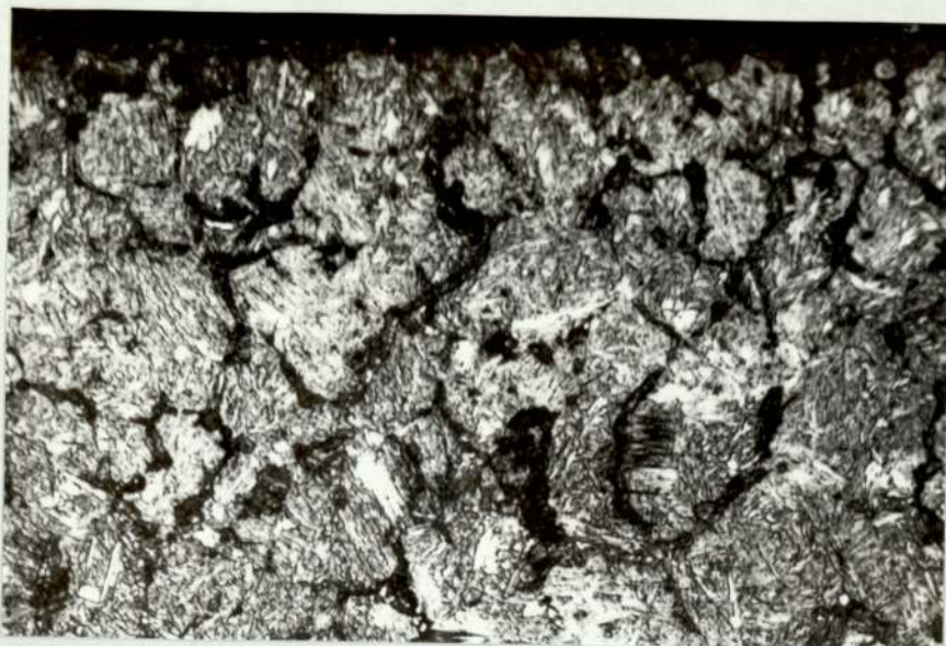
PLATE 10 Microstructure at the notch root, carburised O80M15, root radius 0.76 mm, showing non-martensitic transformation products (case depth 0.38 mm) (magnification x450)
