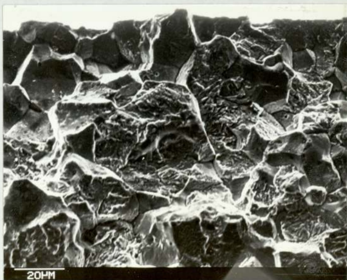
PLATE 49 Fatigue fracture in carbonitrided case at the notch root, case depth 0.38 mm, root radius 3.17 mm, N_i = 211,200
