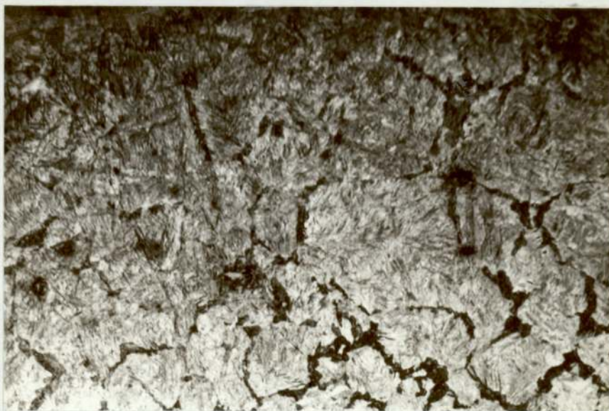
PLATE 13 Microstructure at the notch root, carburised 080M15, root radius 3.17 mm, mid section (case depth 0.76 mm) (magnification x450)
