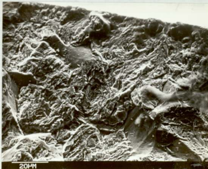
PLATE 43 Fatigue fracture of carburised case at the notch root, case depth 0.38 mm, root radius 1.52 mm, N_i = 118,470
