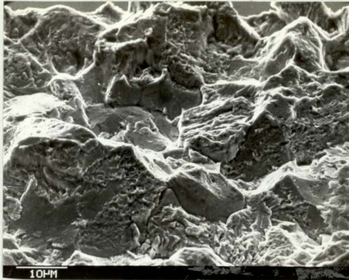
PLATE 46 Fatigue fracture of carburised case at the notch root, case depth 0.76 mm, root radius 1.52 mm, N_i = 305,700
