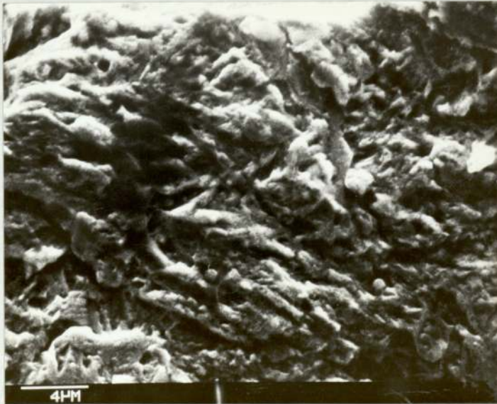
PLATE 35 Fatigue fracture of carburised case at the notch root, case depth 0.76 mm, root radius 0.76 mm, N_i = 229,000
