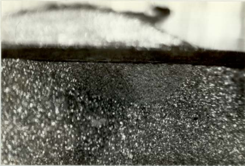
PLATE 4 Fatigue crack shape at initiation in O80A47 specimen (magnification x24)
