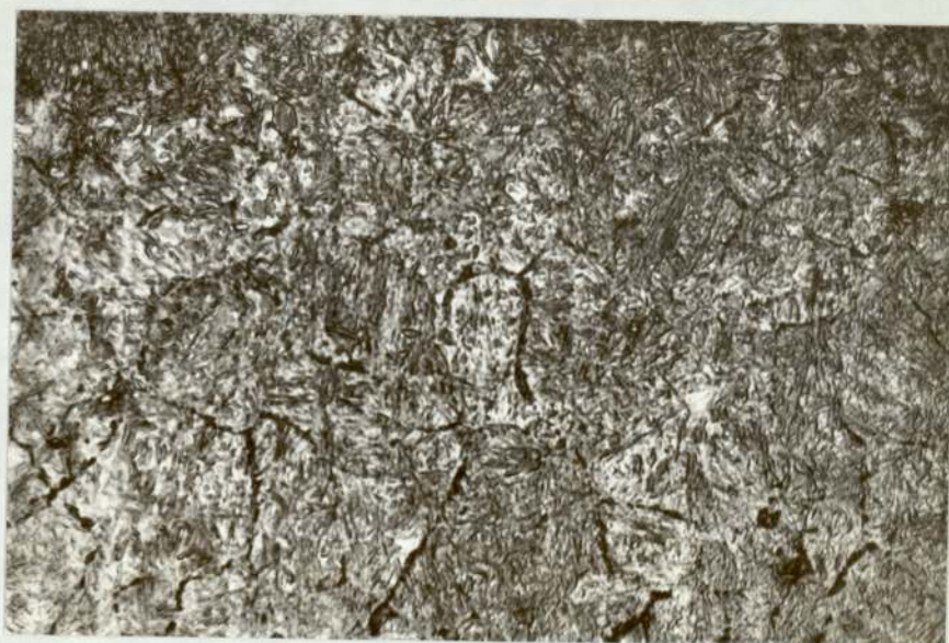
PLATE 11 Microstructure at the notch root, carburised O80M15, root radius 3.17 mm (case depth 0.38 mm) (magnification x450)
