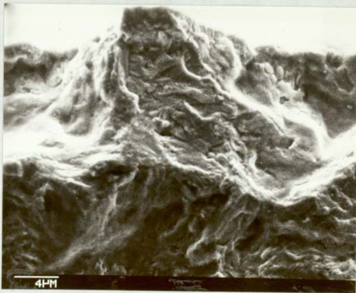
PLATE 33 Fatigue fracture of carburised case at the notch root, case depth 0.76 mm, root radius 0.76 mm, N_i = 241,000
