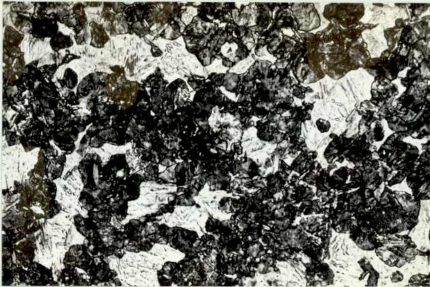
PLATE 28 Microstructure in core of induction hardened O80A47 specimen (magnification x450)
