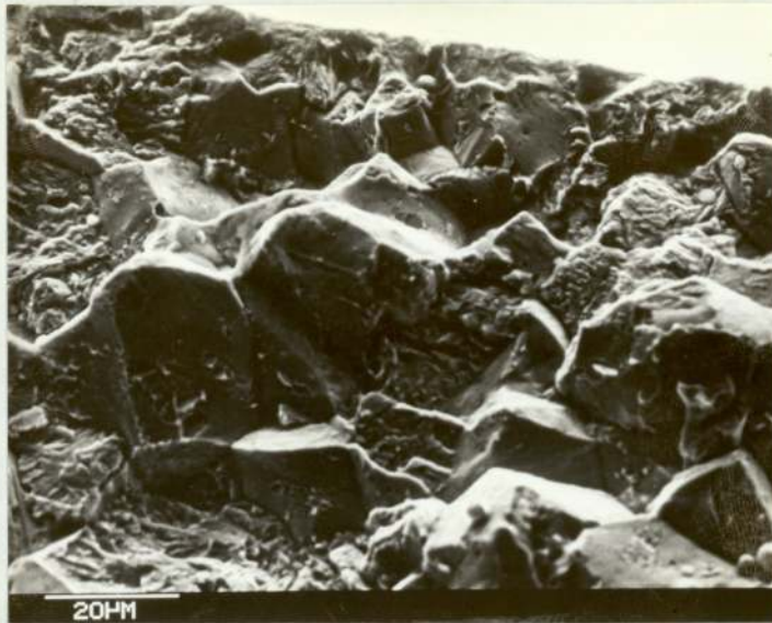
PLATE 42 Fatigue fracture of carburised case at the notch root, case depth 0.38 mm, root radius 1.52 mm, N_i = 62,050
