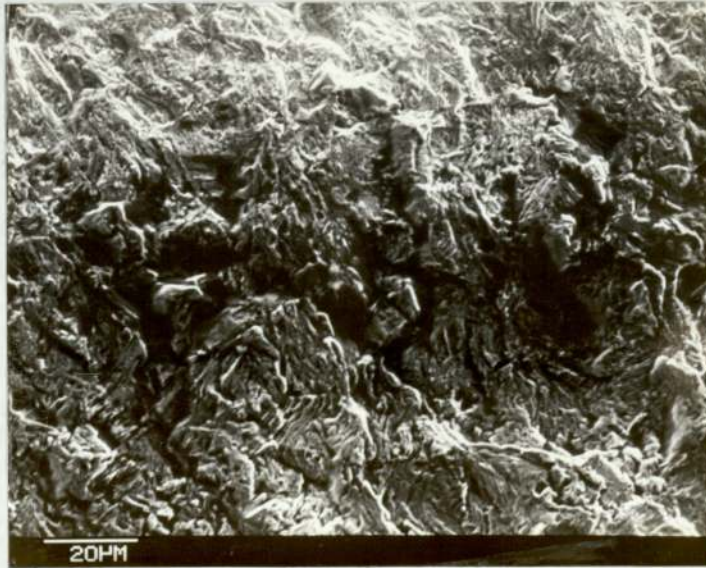
PLATE 41 Fatigue fracture in carbonitrided case below the notch root, showing sub-surface porosity, case depth 0.76 mm, root radius 0.76 mm, N_i = 173,780
