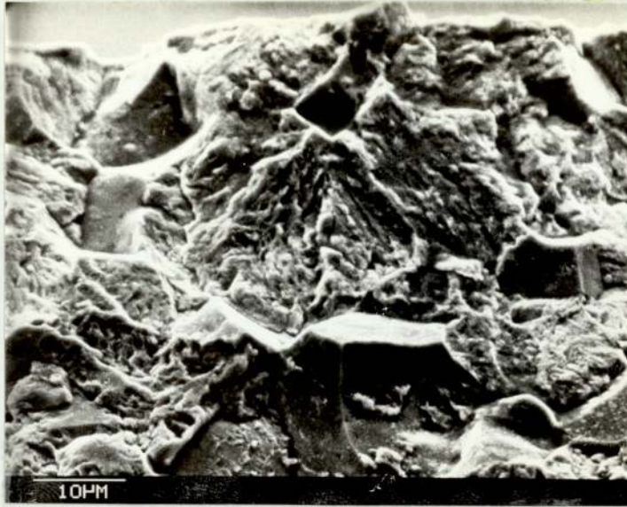
PLATE 50 Fatigue fracture in carbonitrided case at the notch root, case depth 0.76 mm, root radius 1.52 mm, N_i = 185,000
