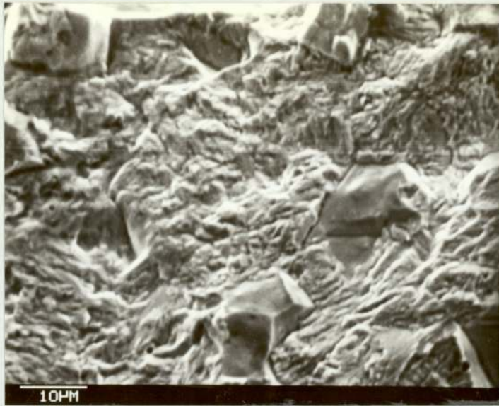
PLATE 38 Fatigue fracture of carbonitrided case at the notch root, case depth 0.76 mm, root radius 0.13 mm, N_i = 168,770
