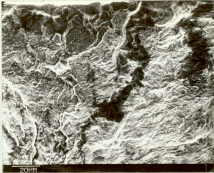
PLATE 40 Fatigue fracture in carbonitrided case below the notch root, showing sub-surface porosity, case depth 0.76 mm, root radius 0.13 mm, N_i = 168,770
