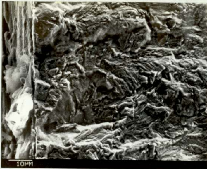
PLATE 30 Fatigue fracture of carburised case below the notch root, case depth 0.38 mm, root radius 0.13 mm N_i = 429,940
