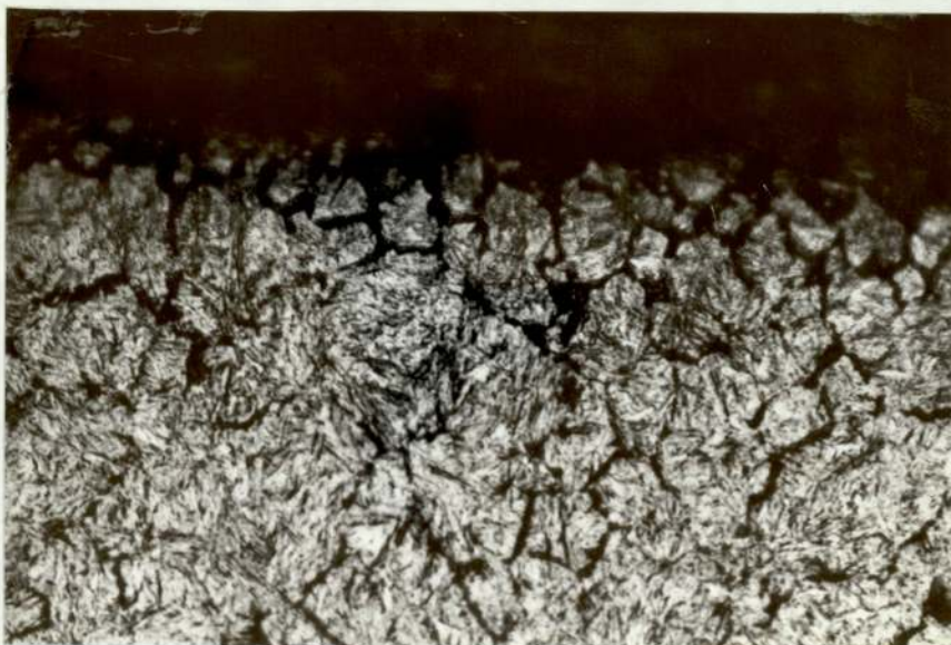
PLATE 16 Microstructure at the notch root, carbonitrided O80M15, root radius 0.13 mm (case depth 0.38 mm) (magnification x450)
