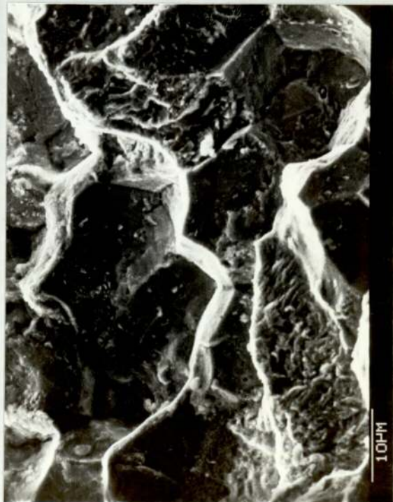
PLATE 74 Fatigue fracture of case in carbonitrided 080M15 at the notch root, showing a cusp grown in transgranular mode surrounded by an area fractured in intergranular mode. Fractography of area at locations A and B is shown at higher magnification in plates marked A and B, root radius 1.52 mm, case depth 0.38 mm, N_i = 158,650
