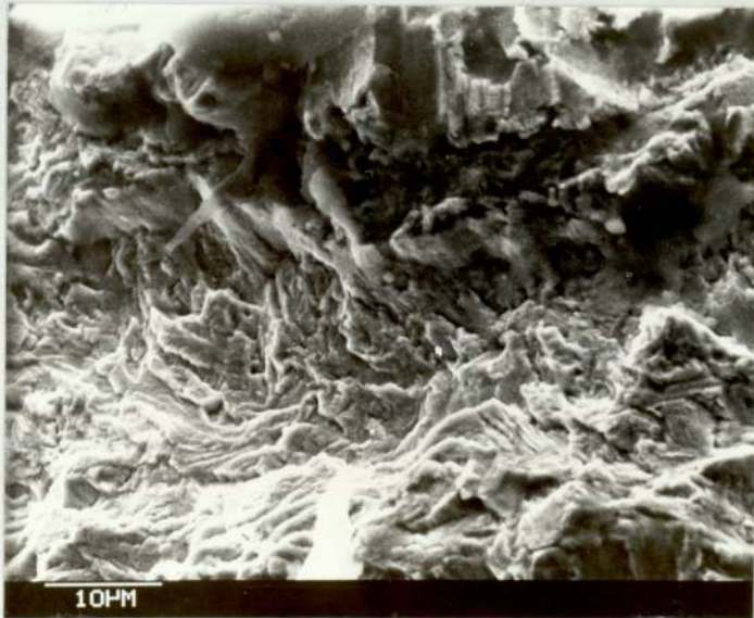
PLATE 67 Fatigue fracture of case in induction hardened O80A47, location: notch root, midsection, root radius 0.76 mm, N_i or N_f = 377,000
