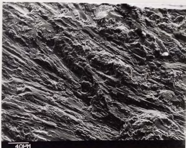
B - Detail of fracture behaviour in fatigue zone Alloy: 2Mo AsCAST
