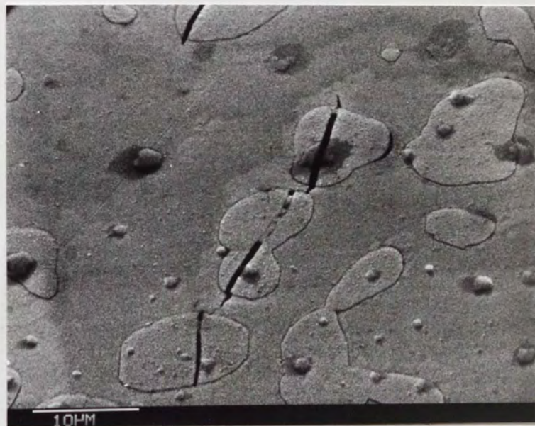
PLATE 39A: Initiation of microcracks at the eutectic carbides in the austenitic alloys
