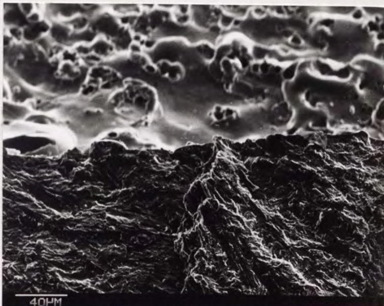
B - General Appearance of fatigue zone. Note: spark machined notch Alloy: 4M2Mo
