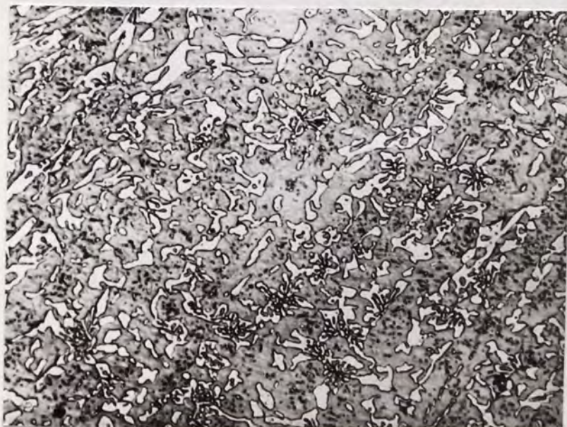
PLATE 19: Effects of heat treatment temperature on the microstructure of 2% Mo containing high-Cr cast iron (Holding periods 12 hours). Note: the variation of eutectic carbide
