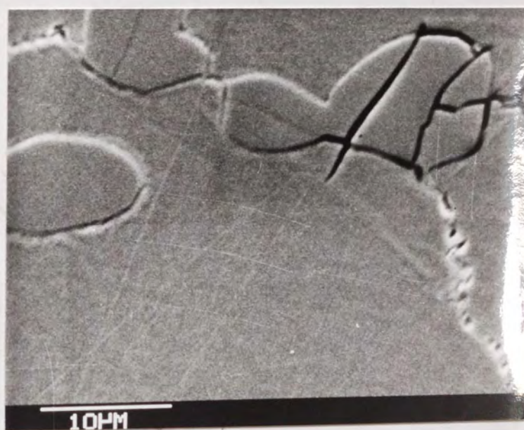
PLATE 39B: Propagation of initiated micro-cracks from the eutectic carbides to surrounding austenitic matrix
