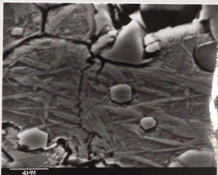
PLATE 22: Stress-assisted martensite formation ahead of the crack tip
