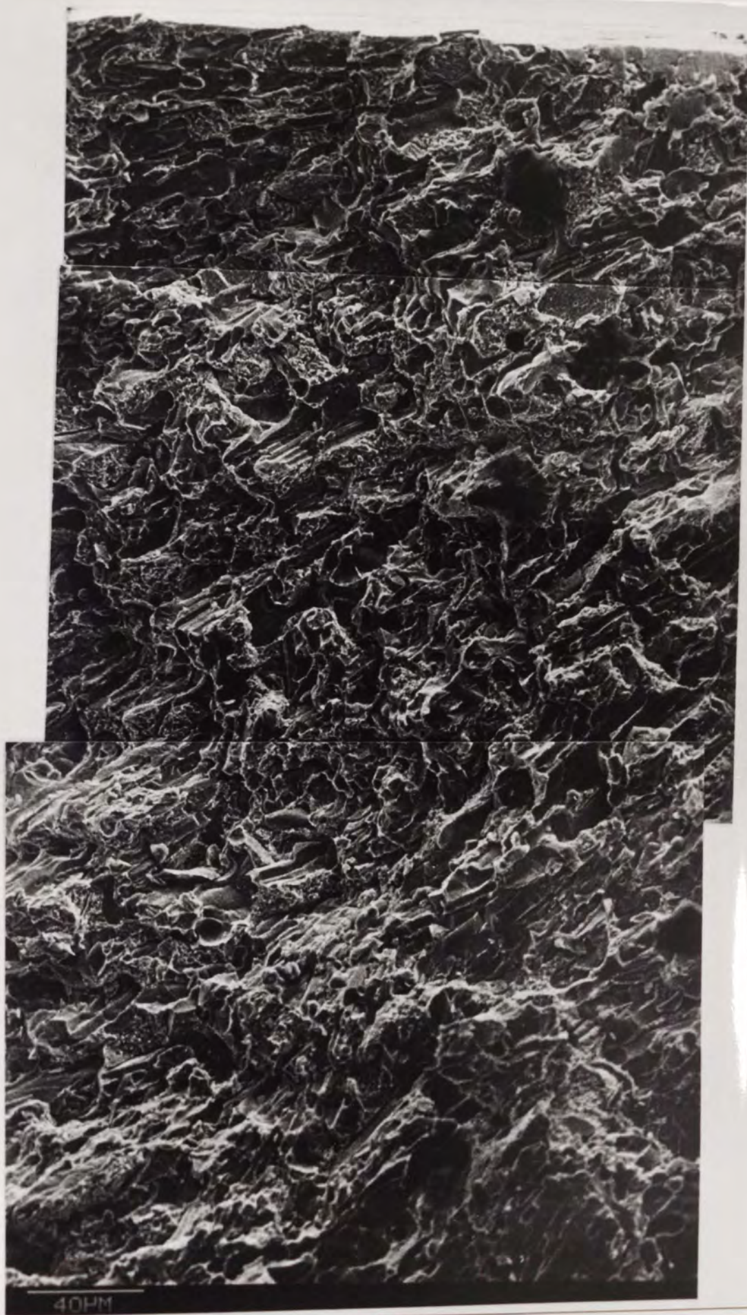
PLATE 32: General appearance of fracture in a martensitic alloy. Note the lower area %age of eutectic carbide on surface compared with austenitic alloys. Alloy: 12M 2Mo
