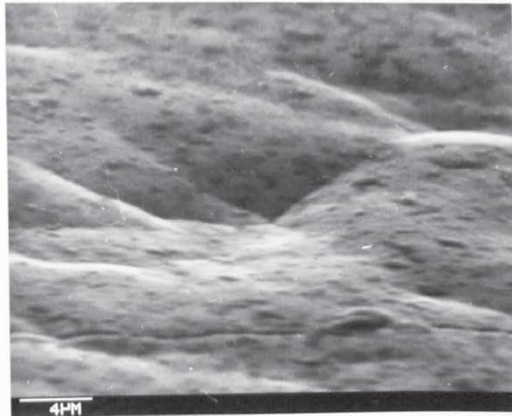
Fig 34a. Cobalt molybdenum deposit on brass substrate x 5K.
