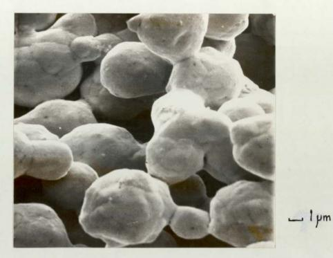
6.45. Scanning electron micrograph of a gold/palladium paste after firing at 1000°C for 10 minutes in a nitrogen 10% hydrogen atmosphere. x 5,400
