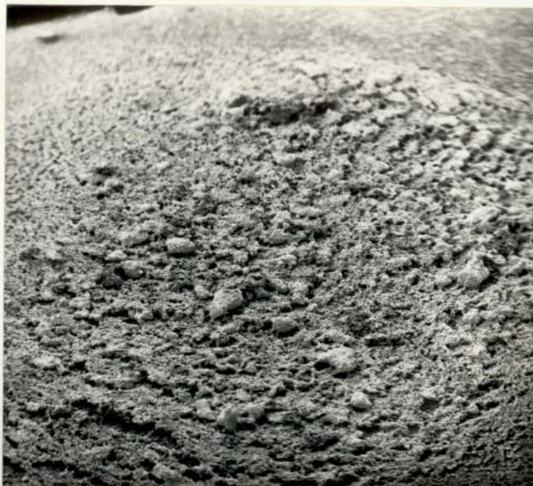
6.8. Scanning electron micrograph of paste dried at 250°C
