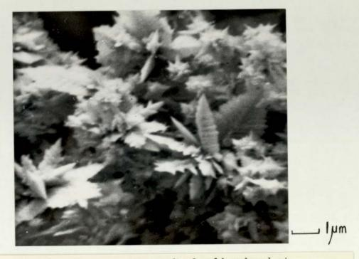
3.24. Scanning electron micrograph of gold reduced at varying temperatures by sulphur dioxide. x 10,000
