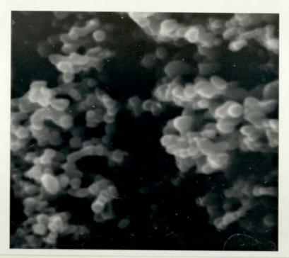
3.71. Scanning electron micrograph of palladium/tin powder from plating on plastics waste. x 10,500
