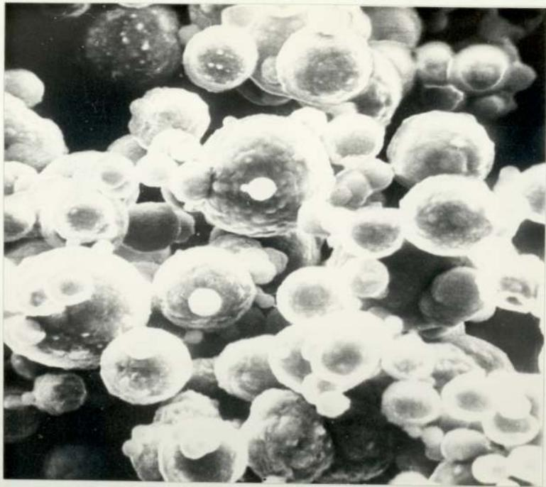
3.73. Scanning electron micrograph of nickel reduced by carbonyl process. x 5,400
