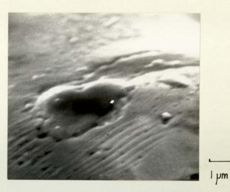
Scanning electron micrograph of the lines seen on a gold/palladium/tin deposit fired at  $1000^\circ\text{C}$  for 10 minutes in argon. x 12,000
