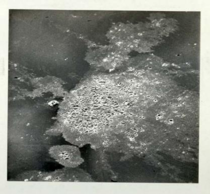
6.2. Scanning electron micrograph of spark damage on polished nickel/iron substrate. x 220
