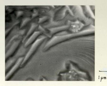
6.93. Scanning electron micrograph of the lines seen on gold/palladium/tin deposit fired at 950°C for 10 minutes in nitrogen. x 10,500
