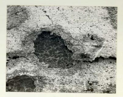
6.73. Scanning electron micrograph of the holes in the gold/ palladium/nickel deposit peeled off a nickel/iron substrate, showing the copper overplate at the base of the holes. x 110
