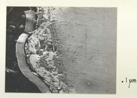
6.79. Scanning electron micrograph of a pure gold which has been fired at  $850^{\circ}$ C for 25 hours in argon. x 600.
