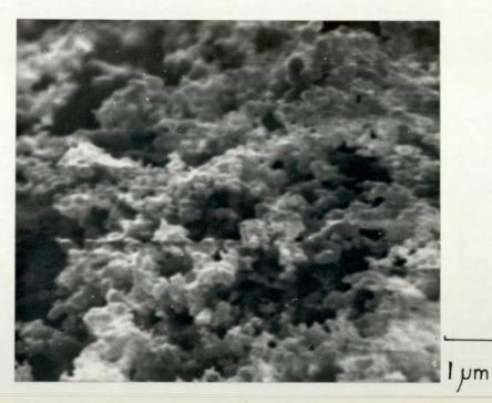
3.52. Scanning electron micrograph of gold reduced by Faraday's solution. x 22,000
