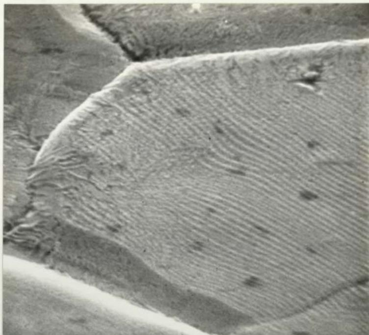
6.32. Scanning electron micrograph of gold fired for 10 minutes at 1000°C. x 1,000
