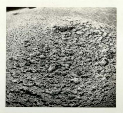
6.8. Scanning electron micrograph of paste dried at 250°C x 24
