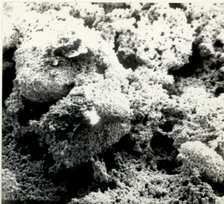
6.39. Scanning electron micrograph of a gold/palladium paste after firing at 900°C for 10 minutes. x 150.
