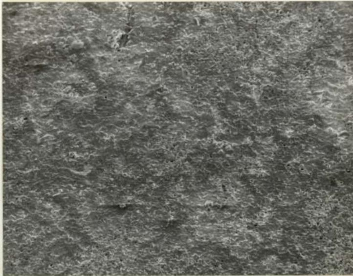
6.71. Scanning electron micrograph of the underside of a pure gold deposit peeled off a nickel/iron substrate. x 100
