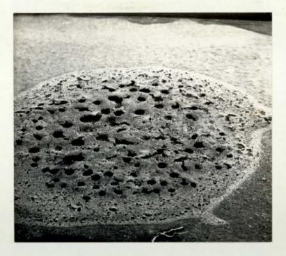
6.57. Scanning electron micrograph of gold/palladium/nickel paste after firing at 950°C for 10 minutes. x 21.
