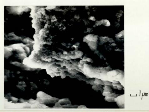
3.64. Scanning electron micrograph of palladium/nickel powder reduced from mixed solution of chlorides by sodium thiosulphate. x 5,400
