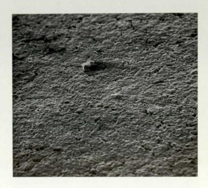
6.6. Scanning electron micrograph of paste mixed with a three roll mill. x 280
