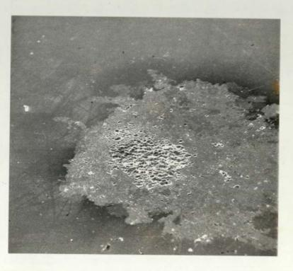
6.3. Scanning electron micrograph of spark damage on polished nickel/iron substrate. x 240
