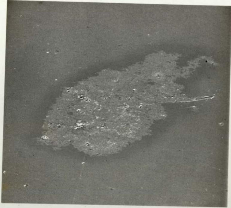
6.4. Scanning electron micrograph of spark damage on polished nickel/iron substrate. x 250
