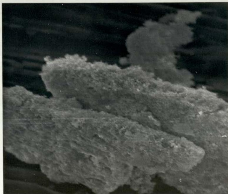
3.17. Scanning electron micrograph of gold reduced at 100°C by sodium hydroxide. x 1,900
