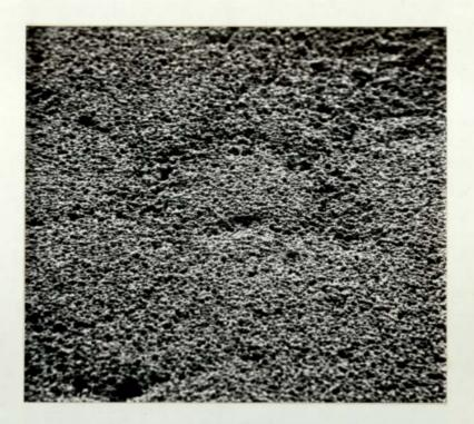
6.5. Scanning electron micrograph of paste mixed with a palette knife. x 230
