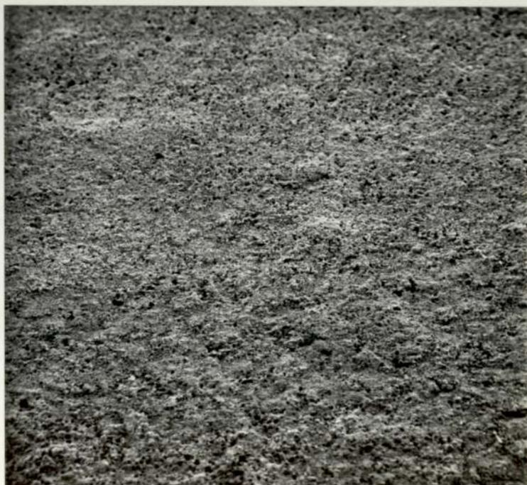
6.58. Scanning electron micrograph of a gold/nickel paste after firing at  $950^{\circ}\text{C}$  for 10 minutes, showing the surface finish. x 110
