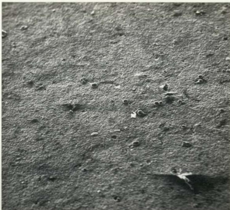
6.37. Scanning electron micrograph showing the surface finish of a fired gold paste containing no glass. x 30.
