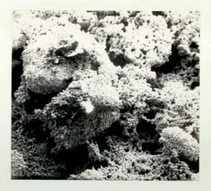
6.39. Scanning electron micrograph of a gold/palladium paste after firing at  $900^{\circ}$ C for 10 minutes. x 150.
