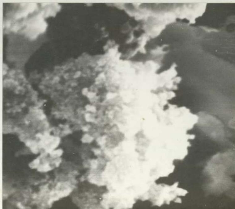
3.5. Scanning electron micrograph of gold reduced by gaseous hydrogen. x 10,000
