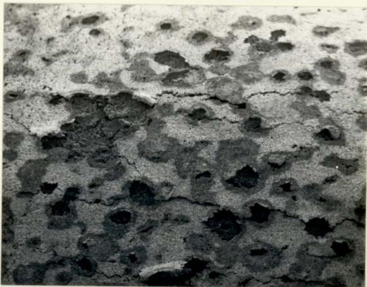
6.72. Scanning electron micrograph of the underside of a gold/palladium/nickel deposit peeled off a nickel/iron substrate. x 21.
