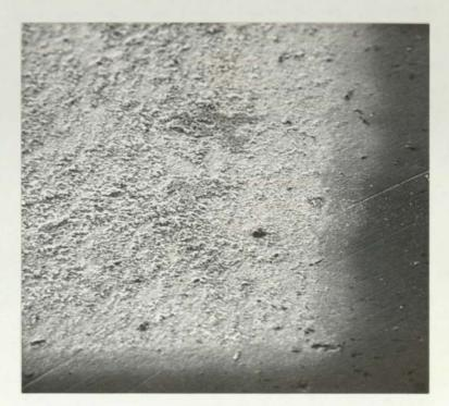
6.38. Scanning electron micrograph showing the surface finish of a fired gold paste containing glass frit. x 23.
