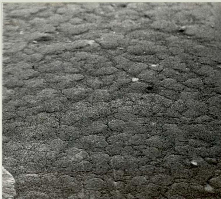
6.9. Scanning electron micrograph of paste dried at 150°C.
