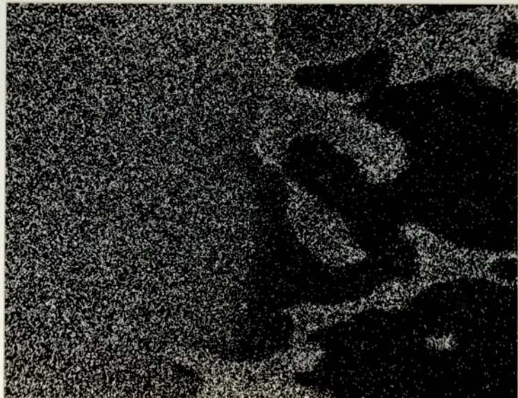
6.78. Distribution of nickel in fig. 6.75. (Nickel  $K\alpha$  line)
