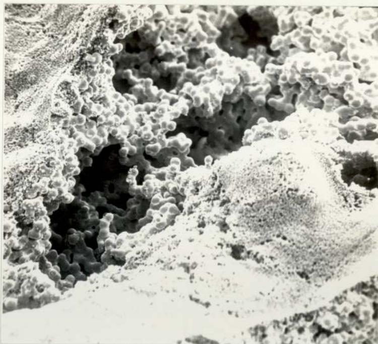
6.46. Scanning electron micrograph of a gold/palladium/tin paste fired at 900°C for 10 minutes. x 375.
