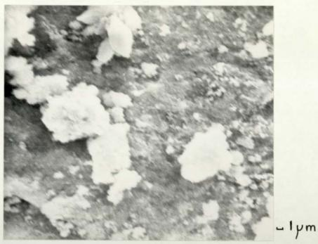
3.7. Scanning electron micrograph of gold reduced by hydrogen sulphide. x 2,100
