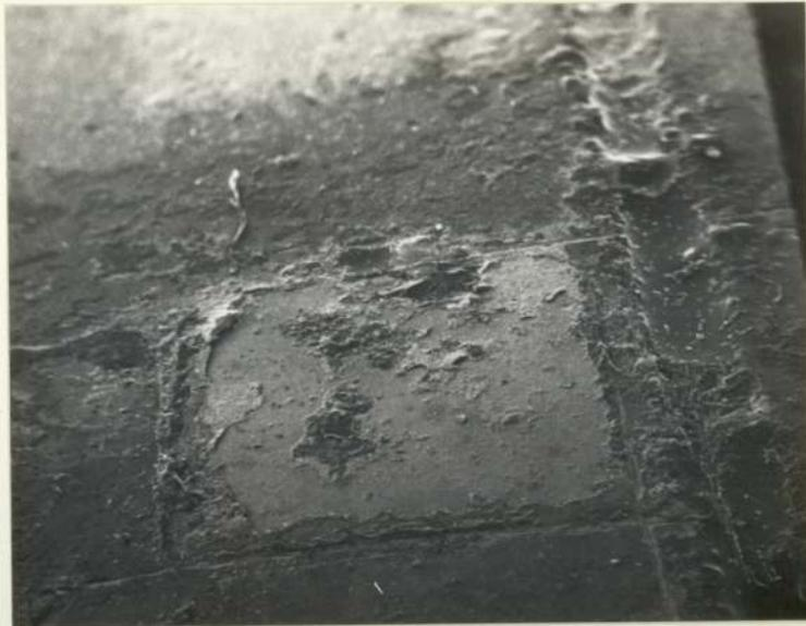
6.69. Scanning electron micrograph of the substrate after adhesion testing using a soldered wire. x 28.
