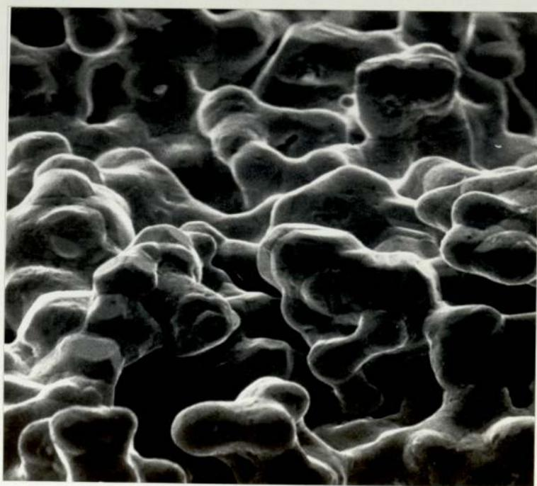
6.44. Scanning electron micrograph of a gold/palladium paste after firing at 1000°C for 10 minutes. x 2,400
