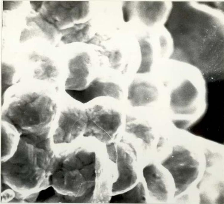
6.41. Scanning electron micrograph of a gold/palladium paste after firing at 900°C for 10 minutes. x 3,700
