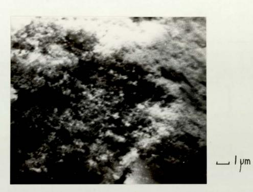
3.66. Scanning electron micrograph of nickel reduced by nascent hydrogen from sodium hydride. x 6,400
