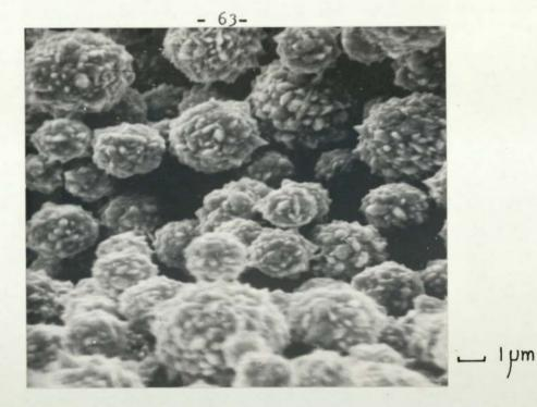
3.25. Scanning electron micrograph of gold reduced at pH 0 by sodium sulphite. x 6,500
