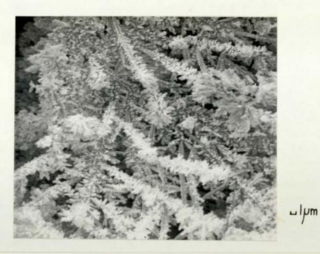
3.56. Scanning electron micrograph of gold found on the cathode after electrolysis. x 2,200
