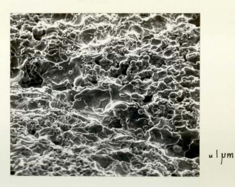
6.86. Scanning electron micrograph of the spark damage on an
