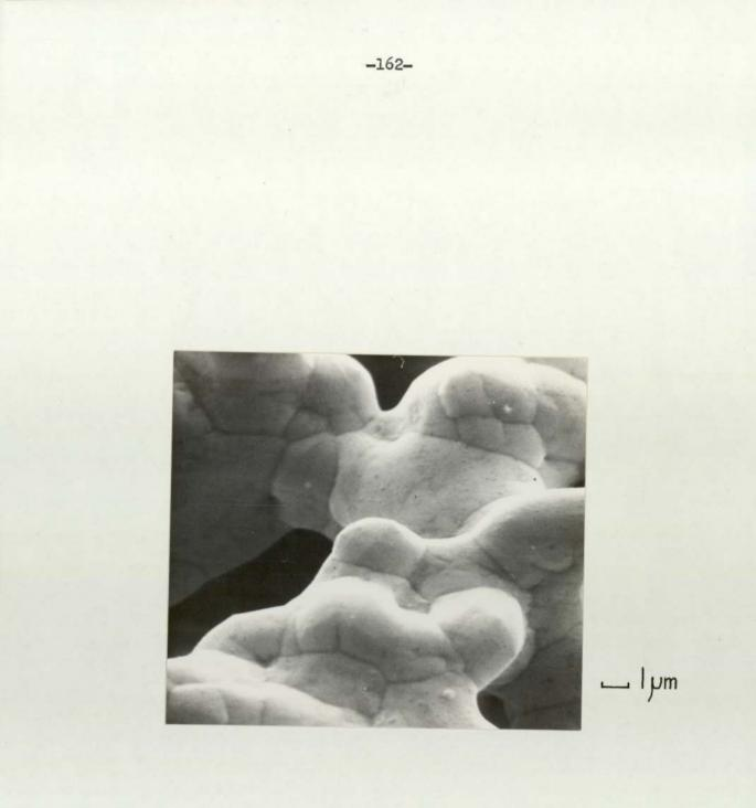
6.28. Scanning electron micrograph of gold fired in argon at 900°C for 60 minutes. x 6,500
