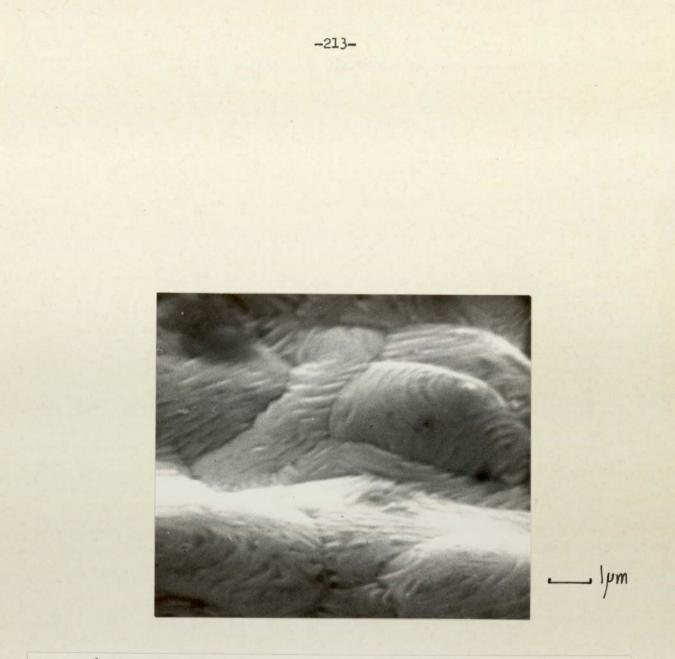
6.94. Scanning electron micrograph of the lines seen on a pure gold deposit fired at 950°C for 10 minutes in argon. x 11,000
