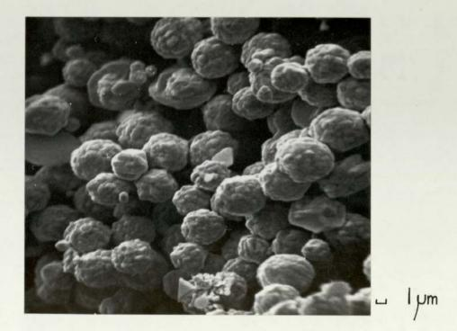
3.31. Scanning electron micrograph of gold reduced at pH 2 with a gold chloride : sodium sulphite ratio of 0.5 x 2,900
