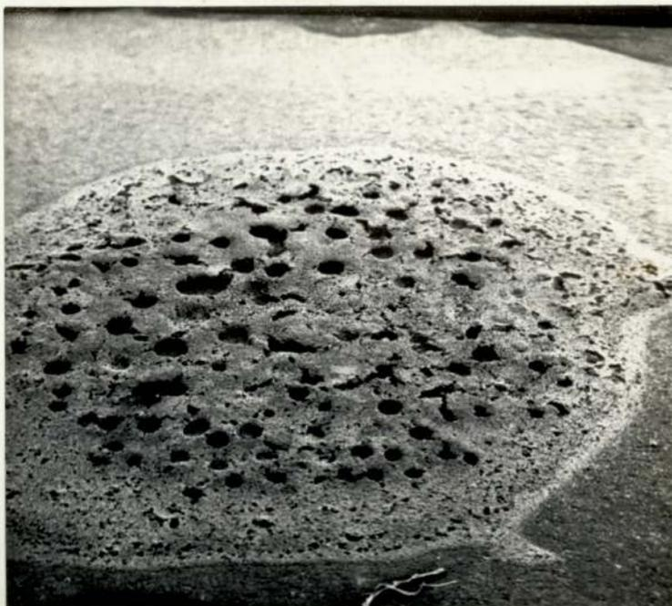
6.57. Scanning electron micrograph of gold/palladium/nickel paste after firing at  $950^{\circ}\text{C}$  for 10 minutes. x 21.
