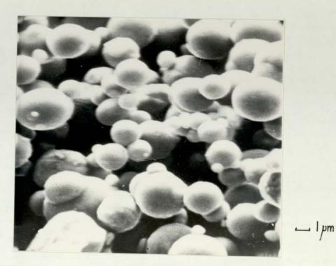
3.74. Scanning electron micrograph of iron reduced by carbonyl process. x 5,400
