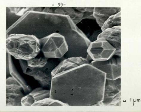
3.18. Scanning electron micrograph of gold reduced by acetone at room temperature. x 2,000
