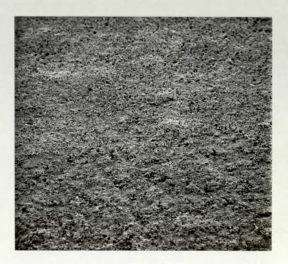
6.58. Scanning electron micrograph of a gold/nickel paste after firing at 950°C for 10 minutes, showing the surface finish. x 110
