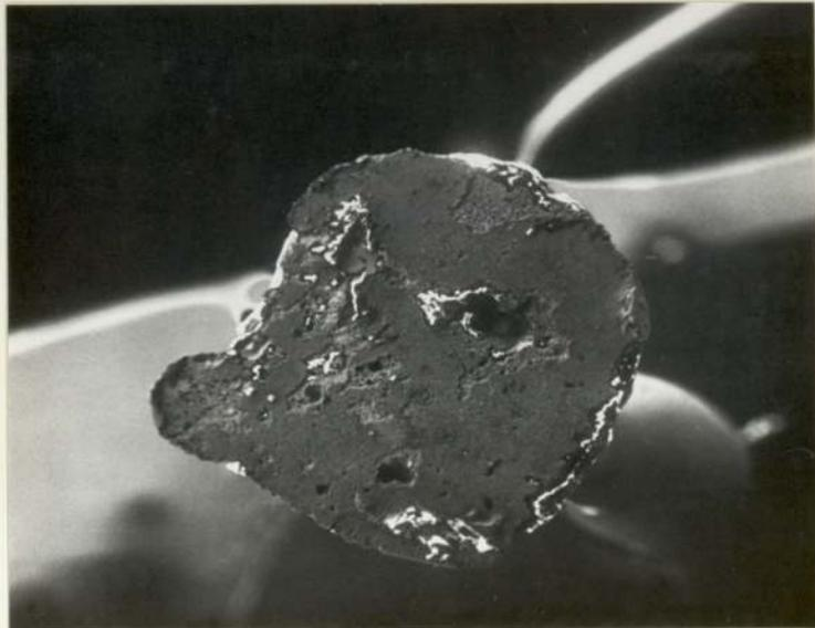
6.70. Scanning electron micrograph of the underside of the soldered area pulled off the substrate shown in fig. 6.69. x 32.
