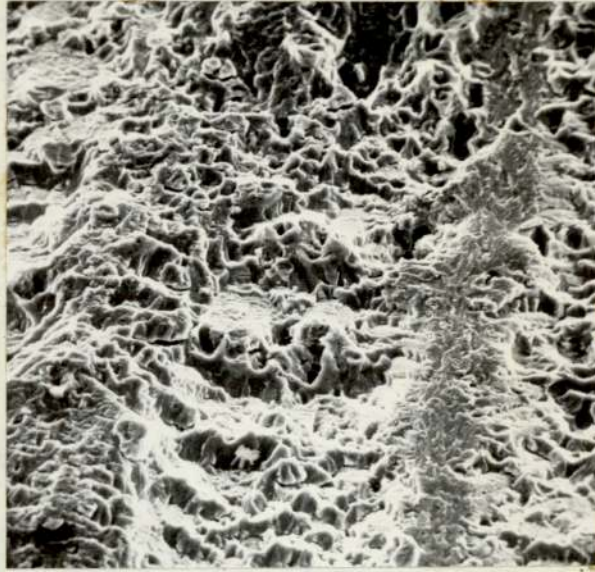
Figure 6.30 X 375 Microvoid coalescence in soft HAZ (2114069) at high \Delta K ( 20\text{MN}/\text{m}^{3/2} ) in 3\frac{1}{2}\% NaCl, R=0.48 .
