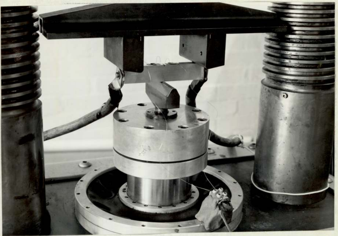
Figure 4.10 Photograph showing current and potential measuring leads on fatigue specimen loaded in bend rig.
