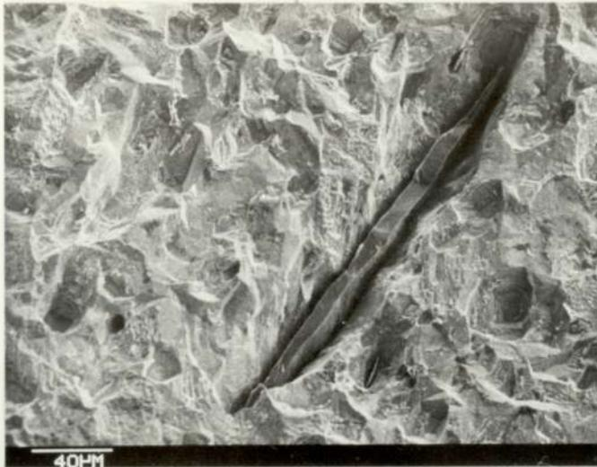
PLATE 80 : INCLUSIONS SECTIONED SUCH THAT IT EXHIBITS ITS TRUE  $\vee$  IN THE POLISHED PLANE.
