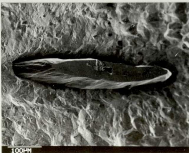
PLATE 82 : INCLUSIONS SECTIONED SUCH THAT IT EXHIBITS A GREATER  $\vee$  THAN ITS TRUE VALUE IN THE POLISHED PLANE.
