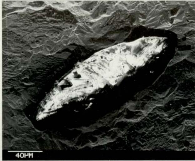
PLATE 25 : DEFORMED Mn-SILICATE INCLUSION.
