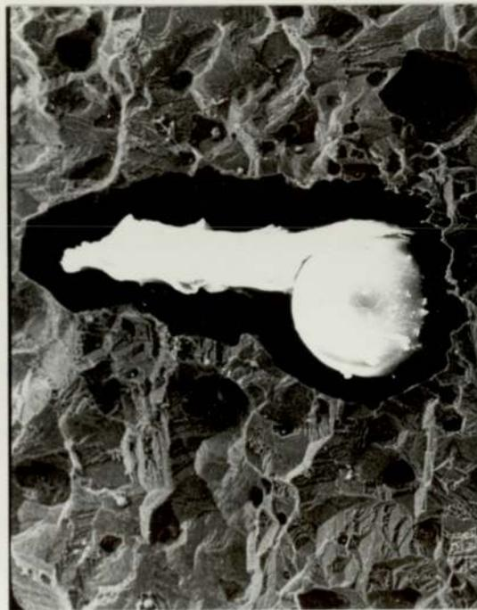
PLATE 41 : THE COMPOSITION OF THE DEFORMED SECTION OF THE INCLUSION IS 45%SiO<sub>2</sub>, 43%MnO, 10%Al<sub>2</sub>O<sub>3</sub>, 1%FeO, 1%S, .WHILST THE COMPOSITION OF THE UNDEFORMED SECTION IS 57%SiO<sub>2</sub>, 31%MnO, 7%Al<sub>2</sub>O<sub>3</sub>, 3%FeO, 2 S. TAKEN FROM MELT A12(0.1%S) ROLLED AT 800°C,  $\epsilon_m = 0.69$ . x1000
