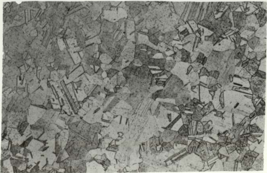
FIG 67 7A53 Aged 500°C for 10^3 s \times 304
