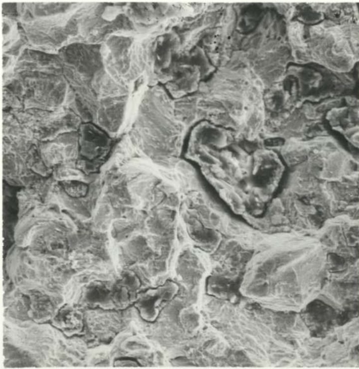
FIG 144 OB Sea Water -100\text{ mV} \dot{\epsilon} 1 \times 10^{-7}/\text{s} x240
