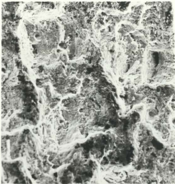
FIG 174 1C54 Sea Water Rest Potential \epsilon^{\circ} 1 \times 10^{-6}/s x360
