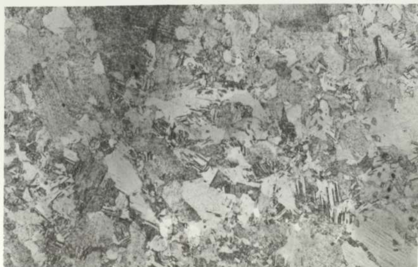
FIG 82 7C56 Aged 500°C for 10^6 s x304
