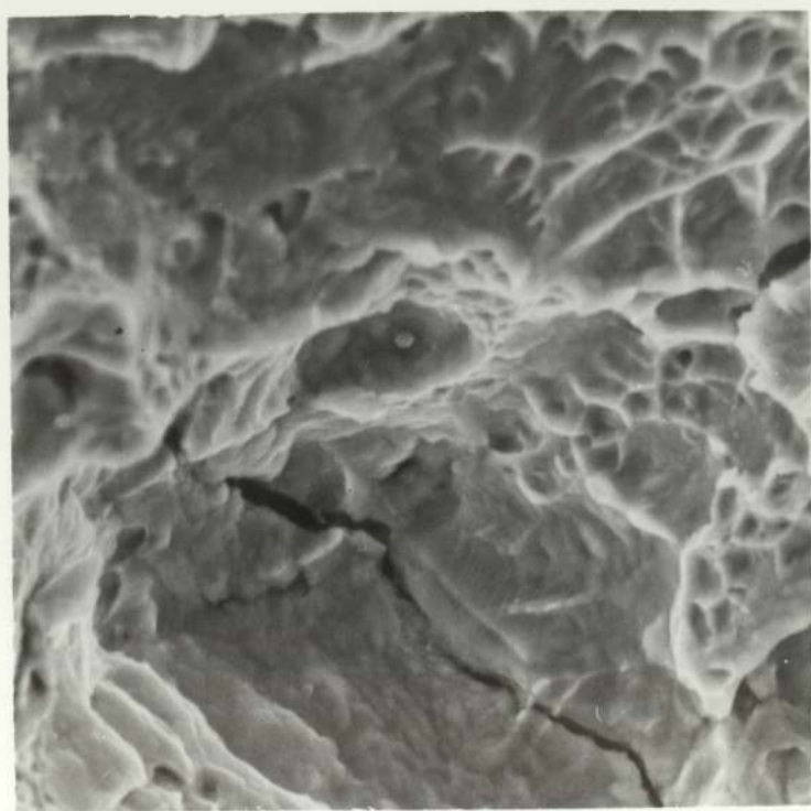
FIG 151 OB NaOH +500 mV pH 12.3 \dot{\epsilon} 1 \times 10^{-6}/s x1200
