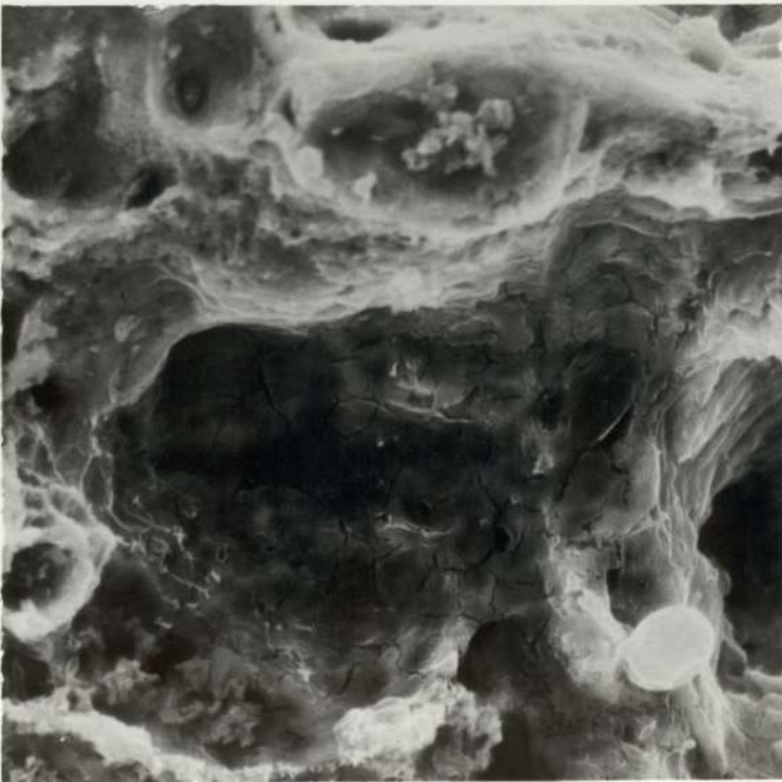
FIG 139 OB Sea Water Rest Potential \dot{\epsilon} 1 \times 10^{-6}/s x1000
