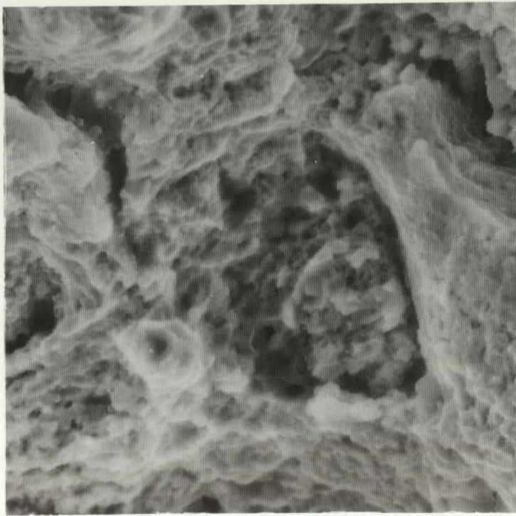
FIG 157 1B Sea Water Rest Potential \xi 1 \times 10^{-6}/s x1000
