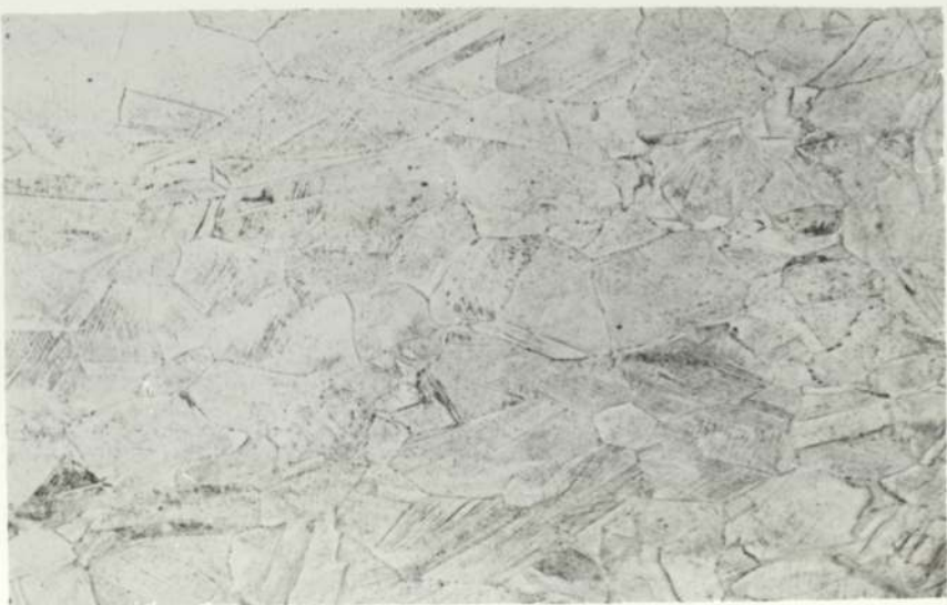
FIG 33 1C 1% Co Solution Treated + 25% Cold Work x304
