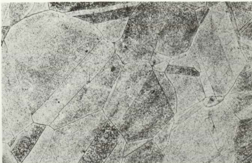
FIG 72 7B52 Aged 500°C for 10 2 s x304
