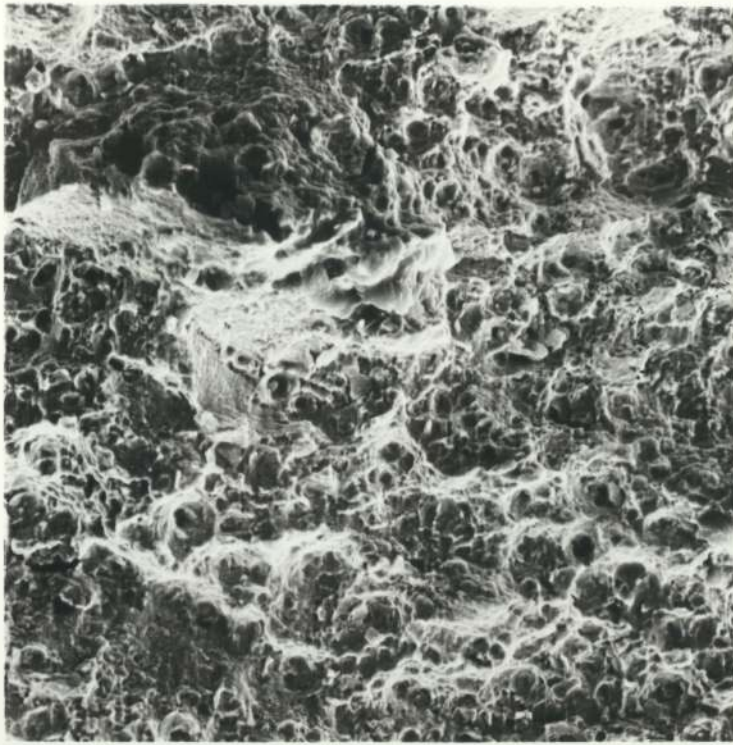
FIG 176 1C56 Sea Water Rest Potential \xi 1 \times 10^{-6}/s x330
