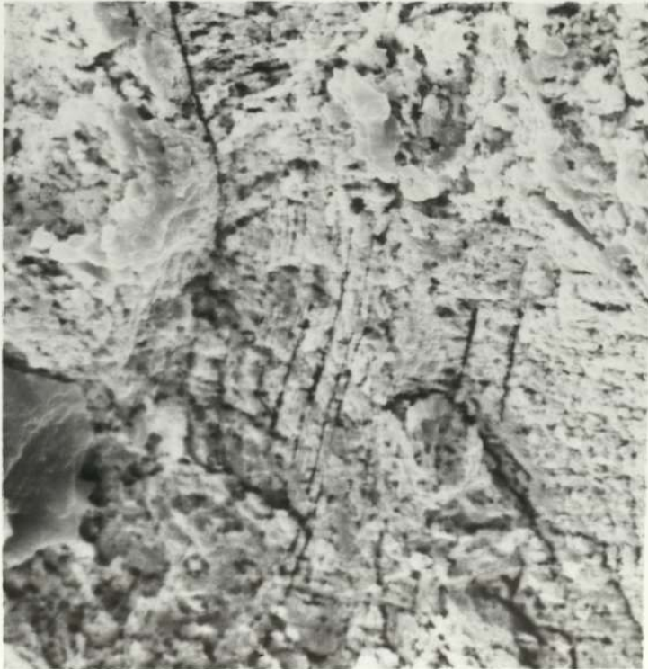
FIG 171 1A56 Sea Water Rest Potential \epsilon^{\circ} 1 \times 10^{-6}/s x1000
