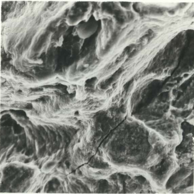
FIG 146 OB Sea Water + L Cystine Rest Potential \bar{\epsilon} \times 10^{-7}/s x650
