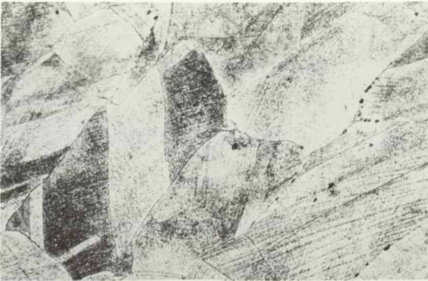
FIG 78 7C52 Aged 500°C for 10 2 s x304
