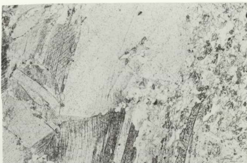
FIG 81 7C55 Aged 500°C for 10^5 s x304
