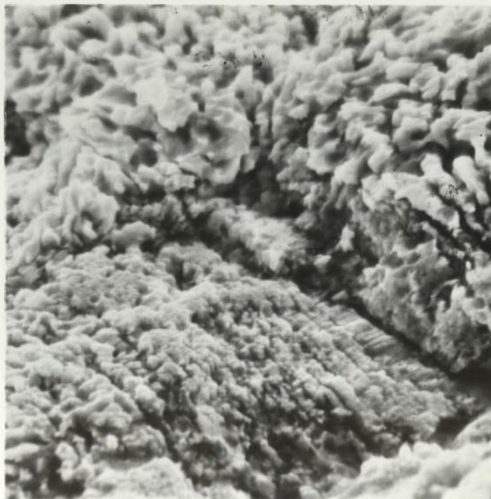
FIG 175 1C54 Sea Water Rest Potential \epsilon^{\circ} 1 \times 10^{-6}/s x2000
