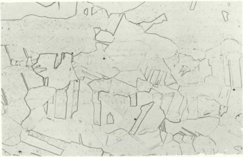
FIG 31 1A 1% Co Solution Treated x304
