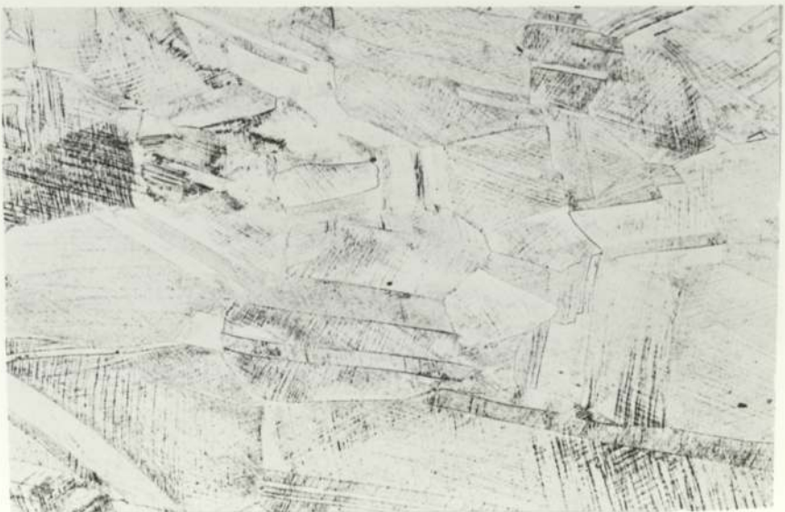
FIG 27 5C 0.5% Co Solution Treated + 25% Cold Work x304
