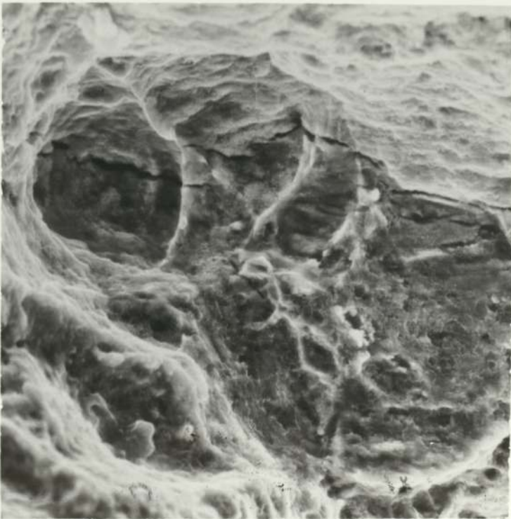
FIG 147 OB Sea Water + L Cystine Rest Potential \bar{\epsilon} \times 10^{-7}/s x900
