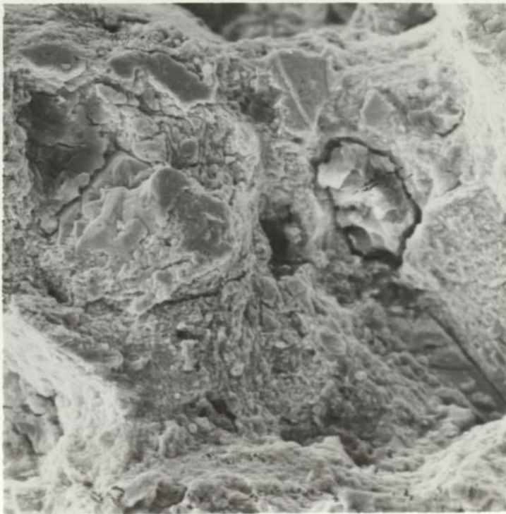
FIG 145 OB Sea Water -100\text{ mV} \dot{\epsilon} 1 \times 10^{-7}/\text{s} x390
