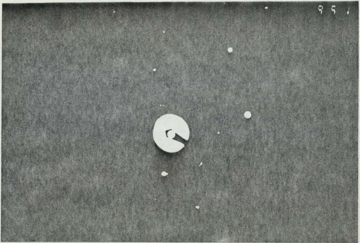
FIG 99 7A55 Selected Area Diffraction Pattern of Fig 98
