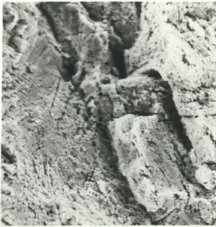
FIG 170 1A56 Sea Water Rest Potential \epsilon^{\circ} 1 \times 10^{-6}/s x1000
