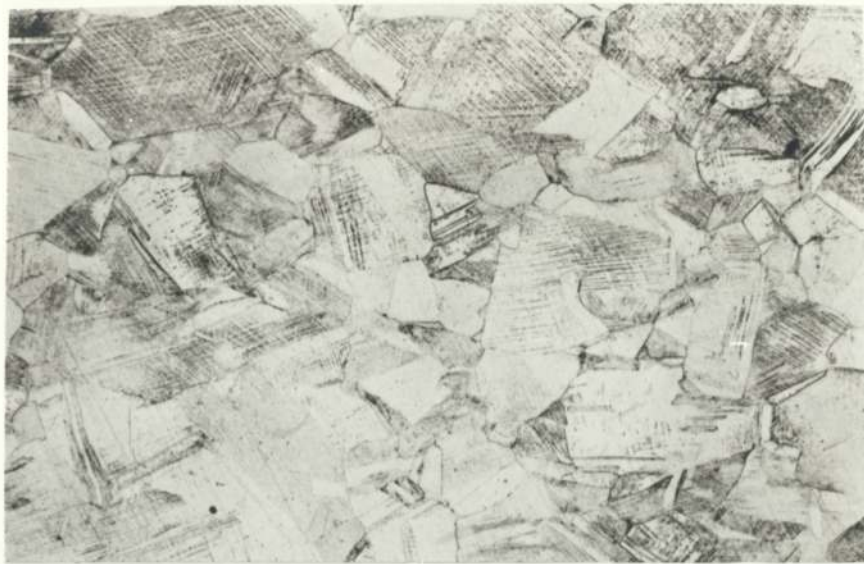
FIG 59 OB U% Co Solution Treated + 12% Cold Work x304
