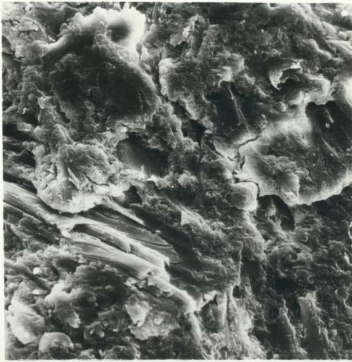
FIG 140 OB Sea Water Rest Potential \dot{\epsilon} 1 \times 10^{-7} / s x240
