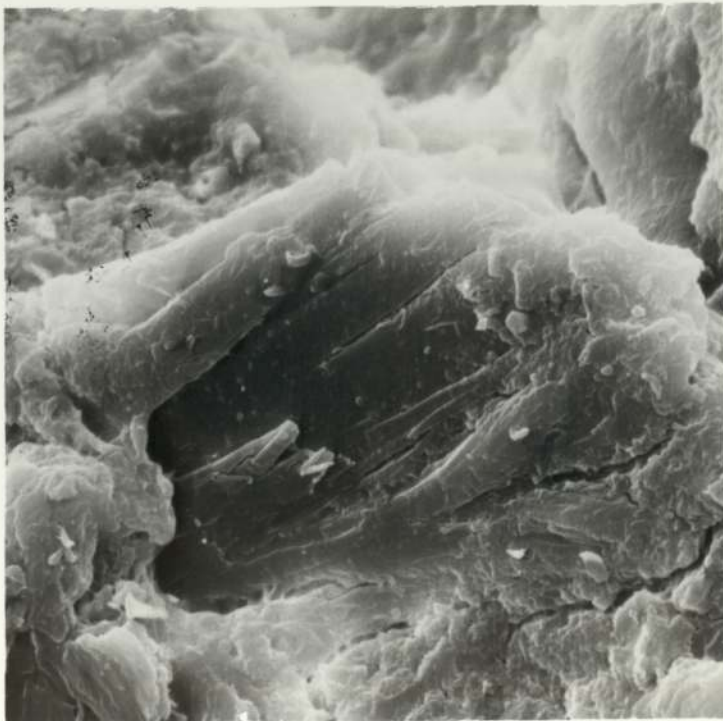
FIG 141 OB Sea Water Rest Potential \dot{\epsilon} 1 \times 10^{-7} / s x800
