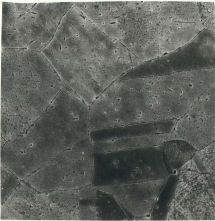
FIG 83 7A 0.7% Co Solution Treated x2200
