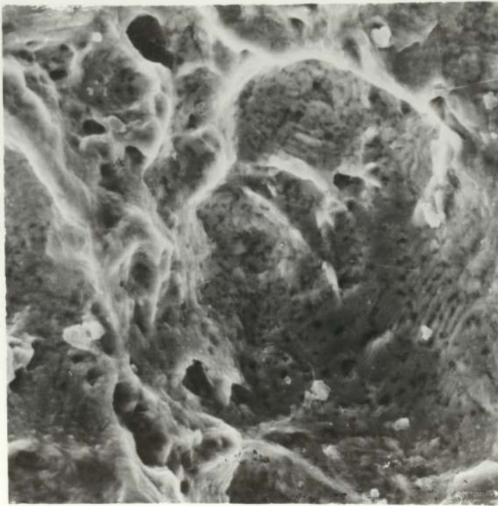
FIG 143 OB Sea Water -200 mV \dot{\epsilon} 1 \times 10^{-7}/s x900
