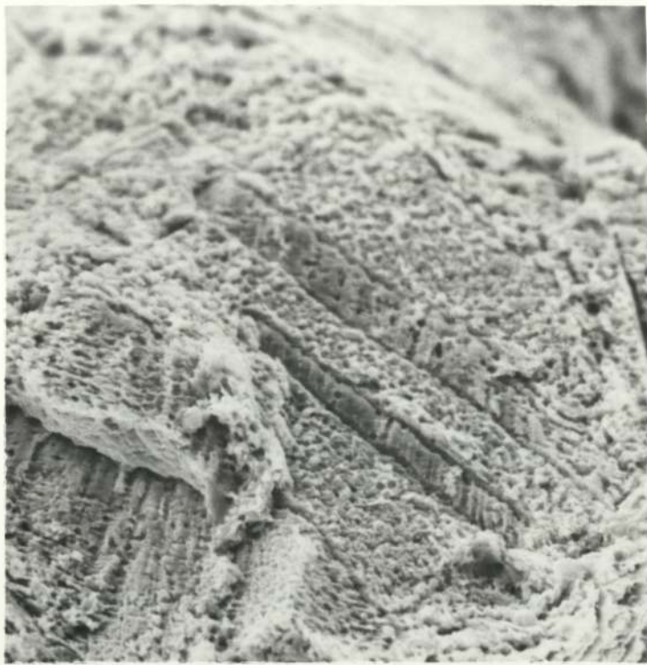
FIG 162 1B54 Sea Water Rest Potential \dot{\epsilon} 1 \times 10^{-6} / s x1000
