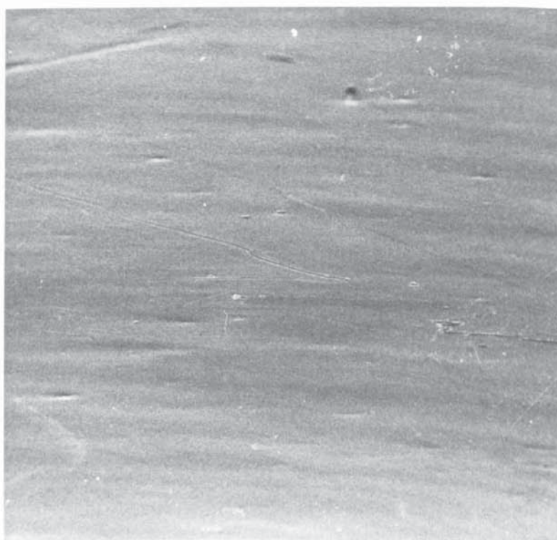
Fig.5.I6. A typical Scanning Electron Micrograph of stainless steel electropolished in the 'gas evolution' region of the anodic dissolution curves of Figs.5.9.-I2. X 550.
