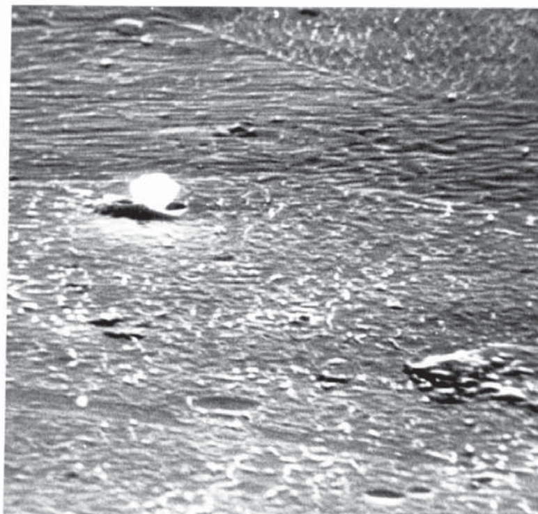
Fig.4.33. Scanning Electron Micrograph of 99.5% Al. Chemically polished in solution K for 180 seconds, with the deposited copper removed. X 5000.
