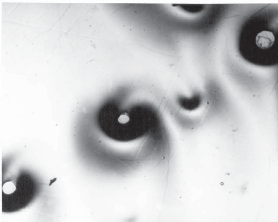
Fig.5.3. Optical Micrograph of 99.99% aluminium immersed live at 4V and electropolished for 10 minutes. X 160.
