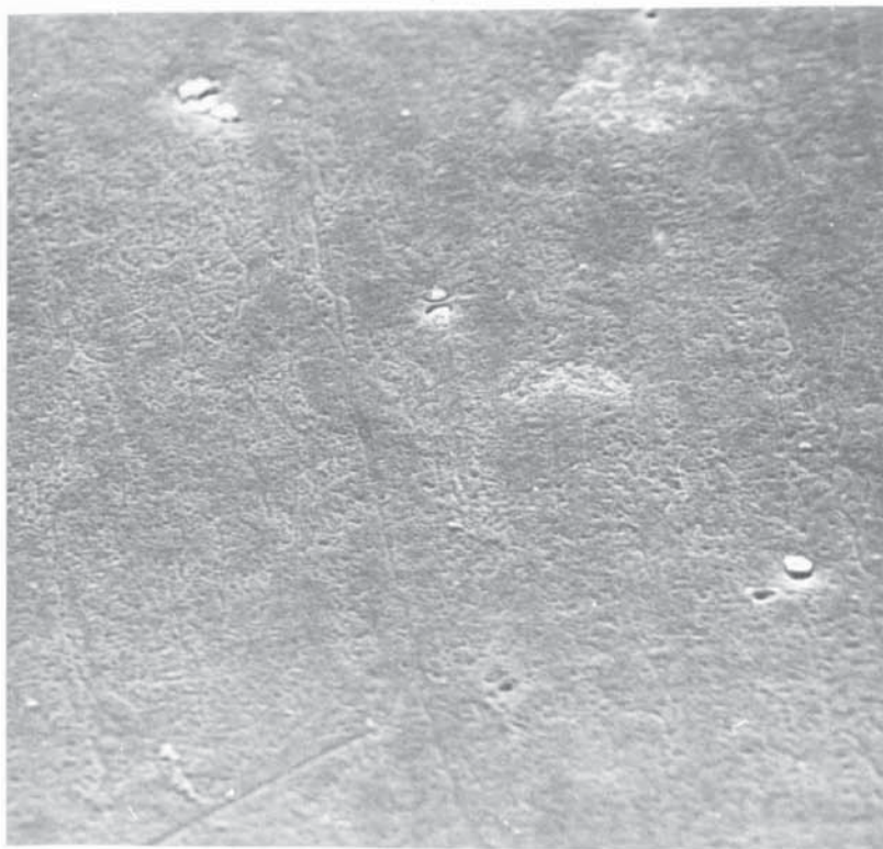
Fig.3.59. Scanning Electron Micrograph of 99.5% Al. Chemically polished in solution D (no nitric acid & 1g/l Cu) for 5 seconds. X 1000.
