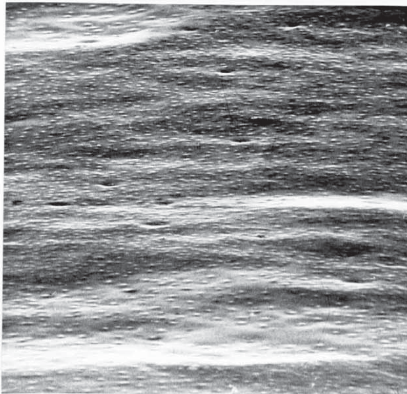
Fig.3.I4. Scanning Electron Micrograph of 99.99% Al. Chemically polished in solution A (no Nitric acid) for 120 seconds. X 1000.
