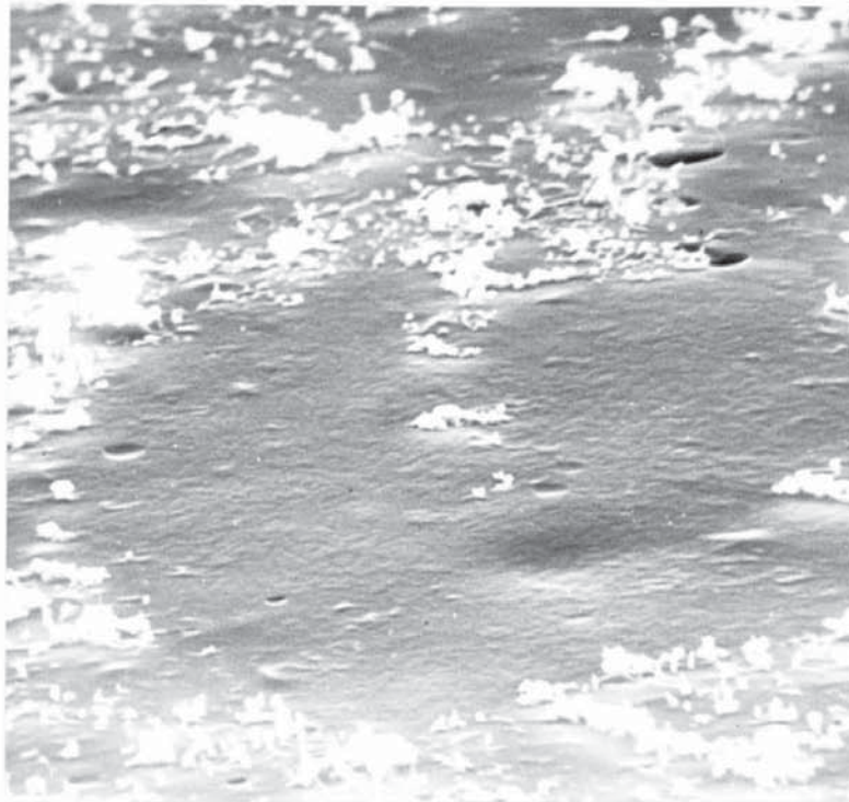
Fig.4.25. Scanning Electron Micrograph of 99.5% Al. Chemically polished in solution J for 180 seconds. X 2000.
