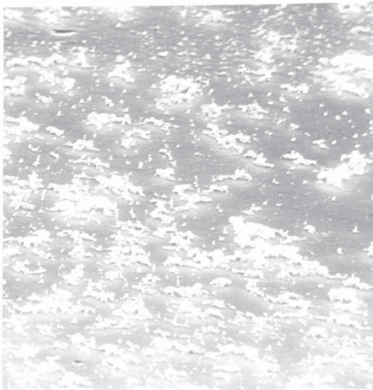
Fig.4.IO. Scanning Electron Micrograph of 99.99% Al. Chemically polished in solution G for 120 seconds. X2000.
