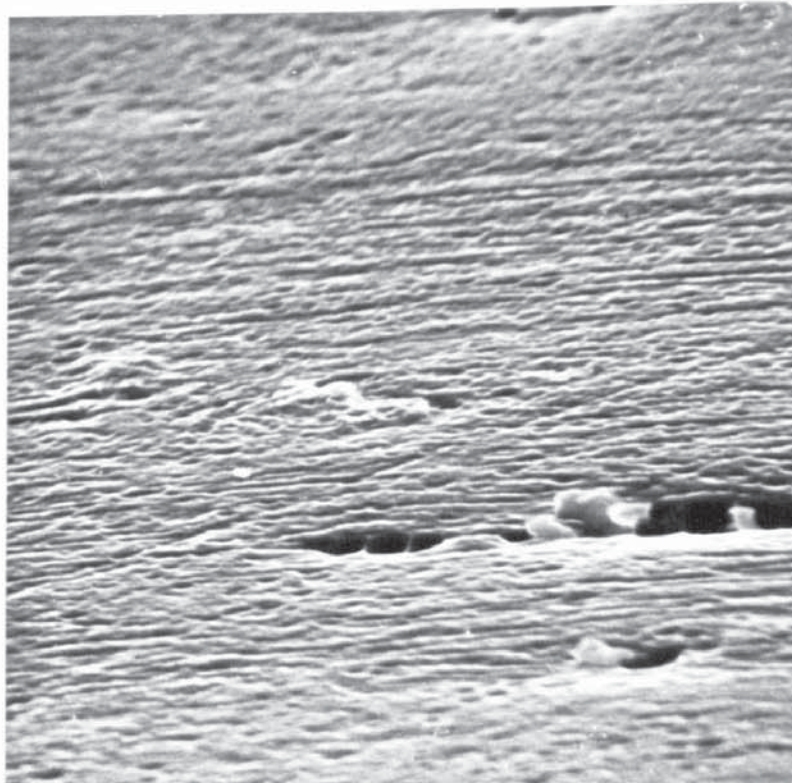
Fig.3.I7. Scanning Electron Micrograph of 99.5% Al. Chemically polished in solution A (no Nitric acid) for 5 seconds. X 2,400.
