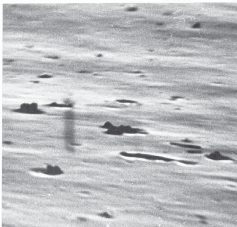
Fig.4.I5. Scanning Electron Micrograph of 99.99% Al. Chemically polished in solution H for 180 seconds, and after immersion in a 50%(by Vol.) nitric acid solution. X 10,000.
