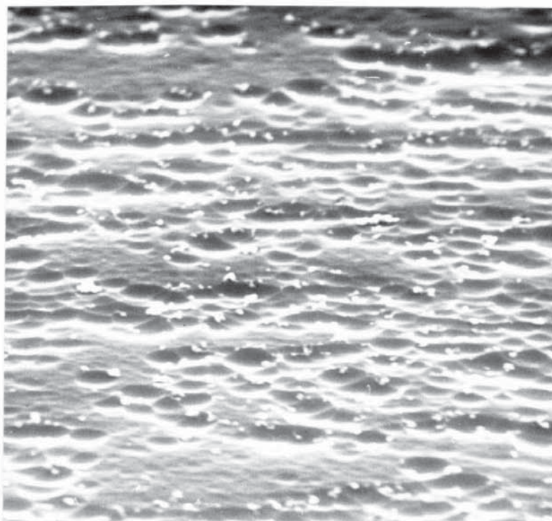
Fig.3.53. Scanning Electron Micrograph of 99.99% Al. Chemically polished in solution D (no nitric acid & Ig/l Cu) for 10 seconds. X 2,400.
