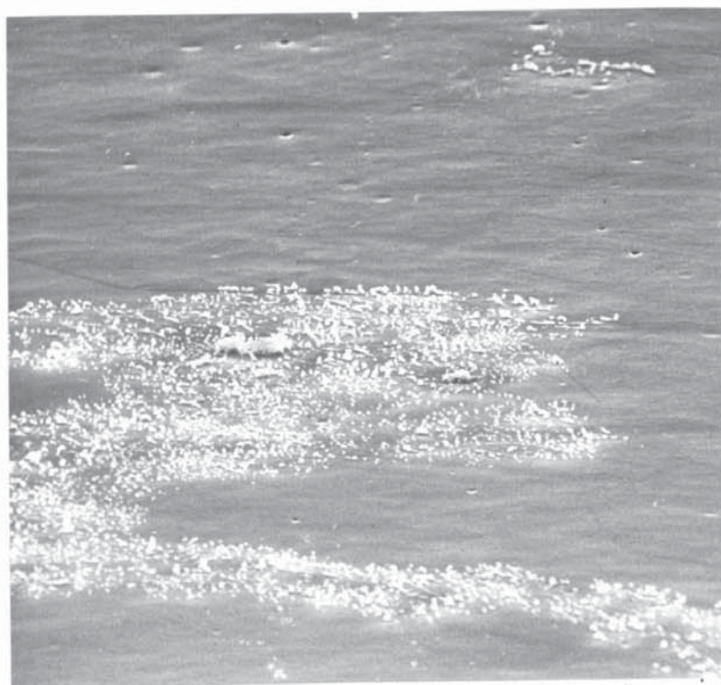
Fig.4.I7. Scanning Electron Micrograph of 99.99% Al. Chemically polished in solution J for 180 seconds. X 1000.
