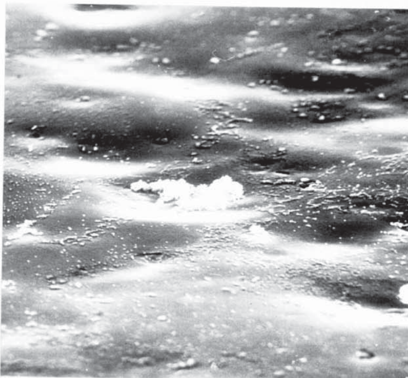
Fig.3.62. Scanning Electron Micrograph of 99.5% Al. Chemically polished in solution D (no nitric acid & 1g/l Cu) for 180 seconds. X 2000.
