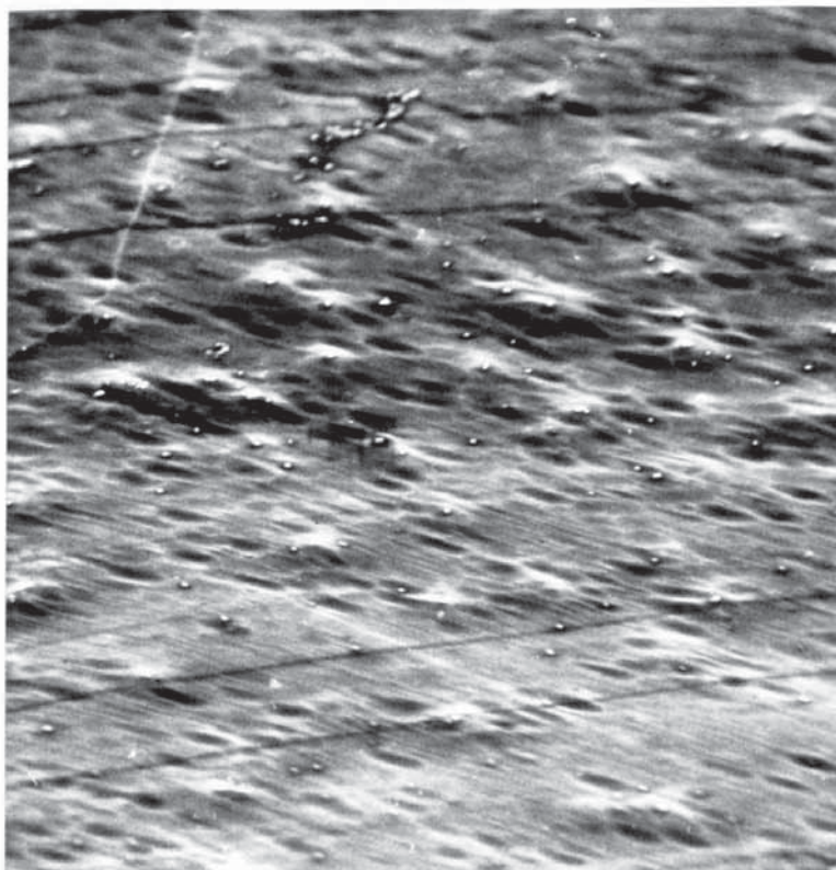
Fig.3.82 Scanning Electron Micrograph of 99.99% Al. Chemically polished in solution F (20% Nitric acid & 1g/l Cu) for 40 seconds. X 2000.
