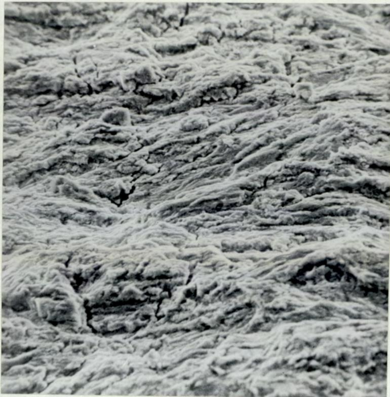
Fig.47. General Transgranular Fracture in QT-B Steel.
