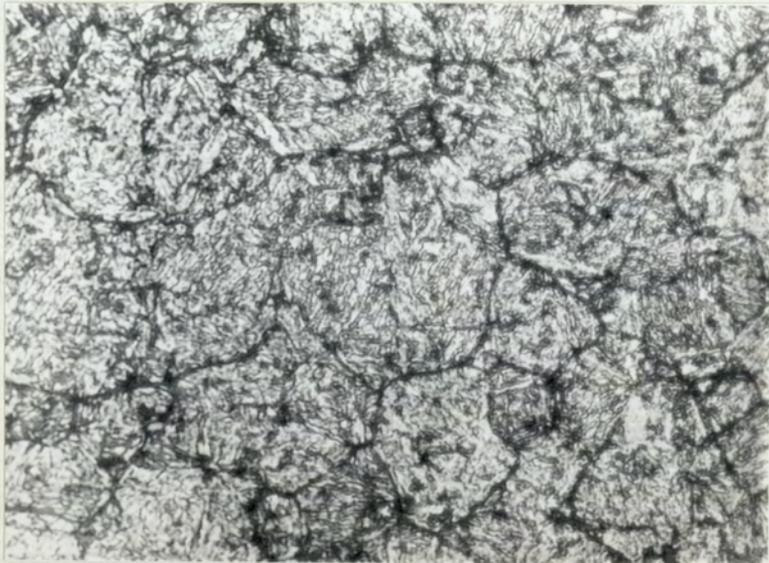
Fig.17. Typical Micro-structure of QT-B Steel.
