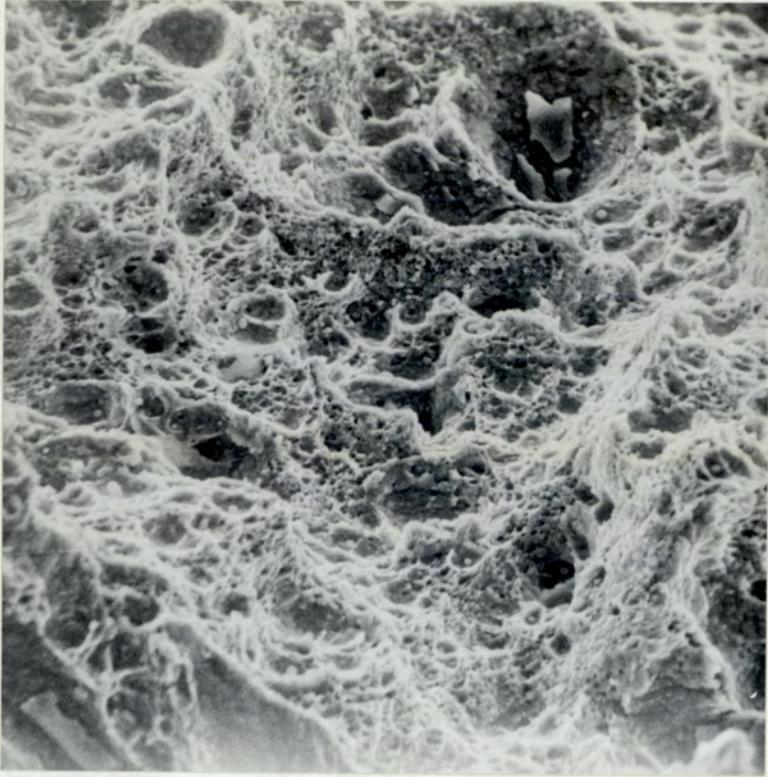
Fig.59. Static Fracture Surface of QT-B Steel.
