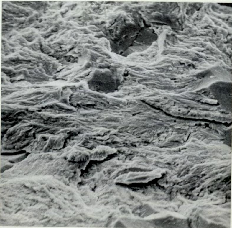
Fig.46. Region of Transgranular Fracture in QT-A Steel.
