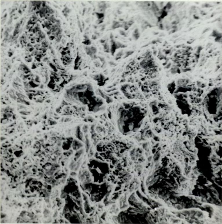
Fig.60. Static Fracture Surface of IS Steel.
