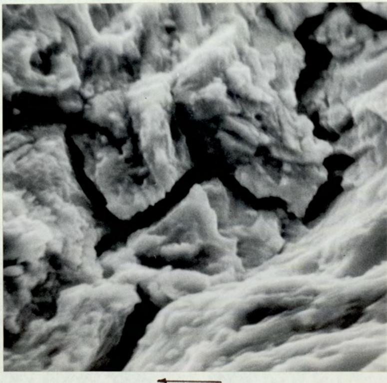
Fig.50. Transgranular Branch Crack in IS Steel. (x 7000)
