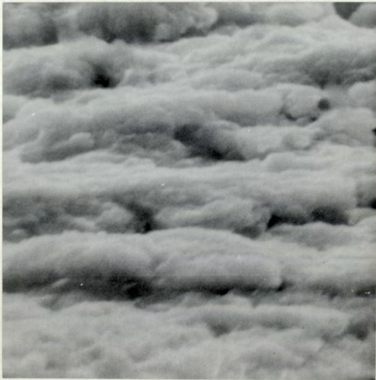
Fig.48. Furrows Running Parallel to Crack Growth Direction in QT-B Steel. (x 13,000)
