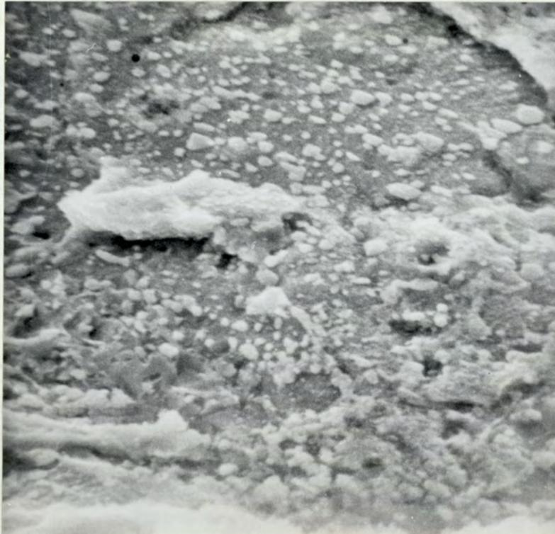
(b) Etched Fracture Surface. (x 6500 )
