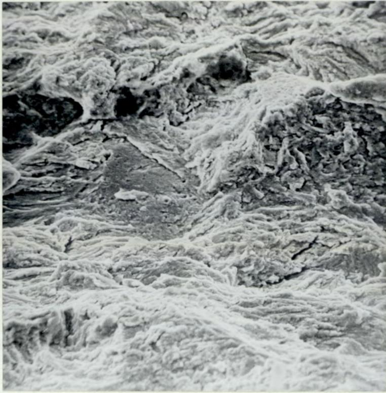
(a) Un-etched Fracture Surface. (x 1300 )
