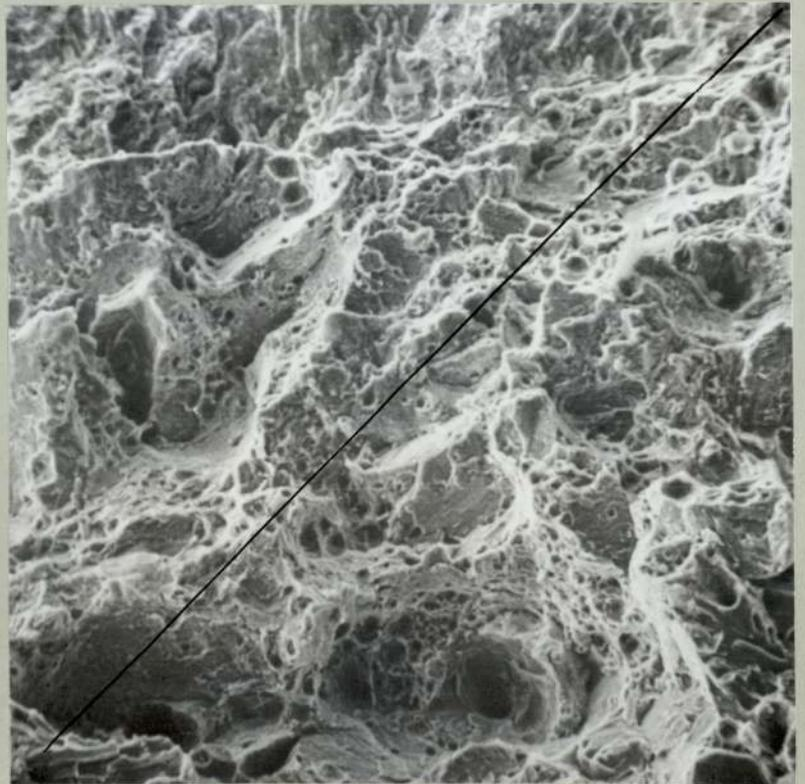
Sample 1B5L. Tested at 200°C. x 300
