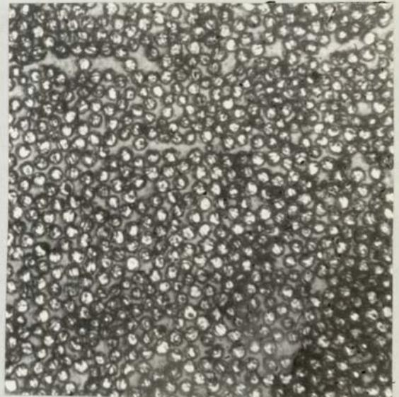
Figure 67 High volume fraction packing in carbon composite. X 250
