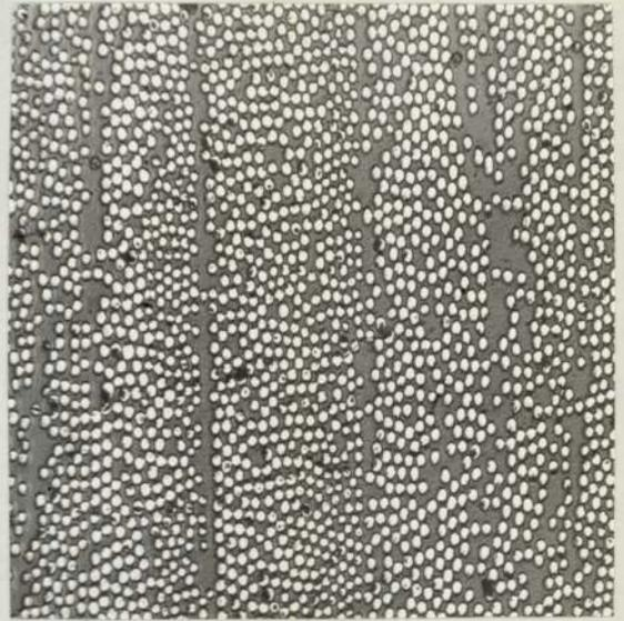
Figure 65 Inter-ply resin rich area in carbon composite. X 120
