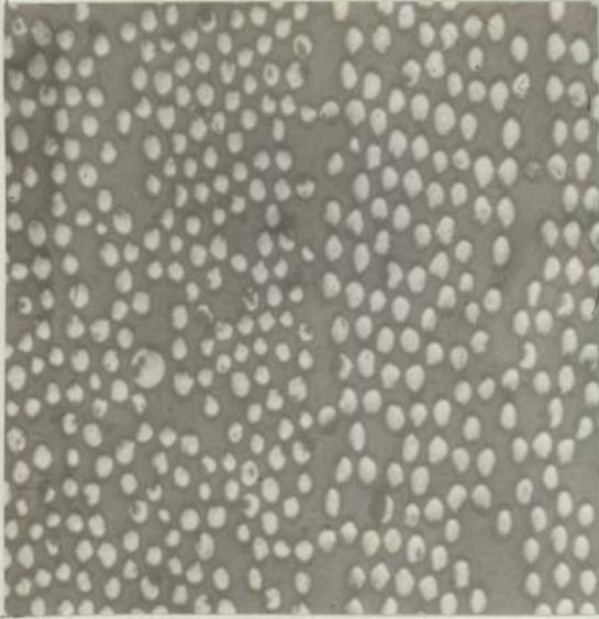
Figure 64 Inhomogeneous glass fibre distribution. X 30
