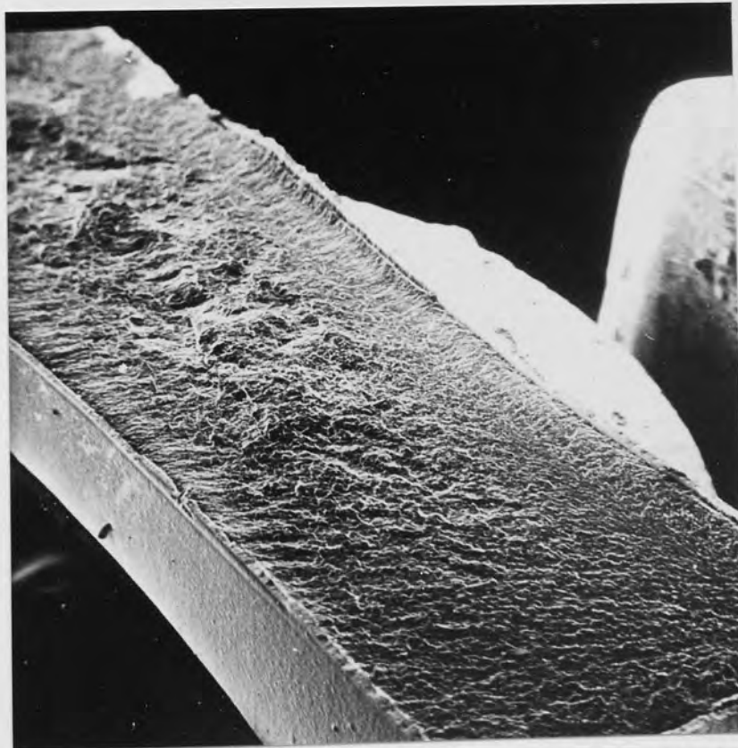
Fig.28b. Scanning electronmicrographs of fractured face of polypropylene grade P after tensile testing; specimen plated with 20 \mu\text{m} copper + 6 \mu\text{m} bright nickel + 0.25 \mu\text{m} microporous chromium. Magnification x 20.
