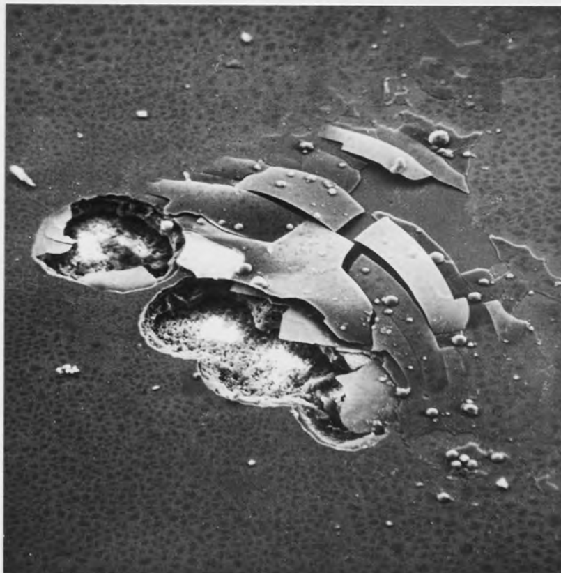
Fig.12. Severe corrosion site produced by CASS testing. Copper had been preferentially corroded and chromium was flaking off. Plastics grade X, process sequence B, coating system No.2. 16 hr. CASS test. Magnification x 300.
