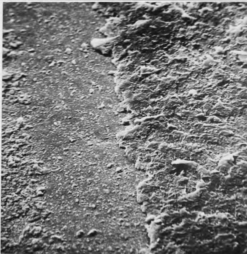
Fig.10. Edge of "corrosion circle" on the underside of the metal foil, after peeling from substrate. A thin layer of plastics was present in the region unaffected by corrosion. Foil stripped from plastics grade X, process sequence B, coating system No.4., 16 hr CASS test. Magnification x 1300.
