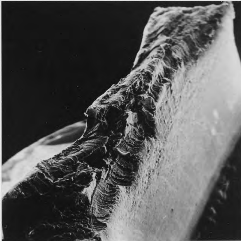
Fig.28a. Scanning electronmicrographs of fractured face of polypropylene grade P after tensile test; specimen in the etched condition. Magnification x 20.
