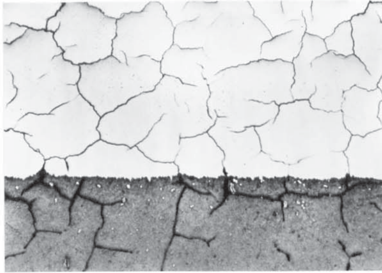
a) Cracking in central plateau region.
