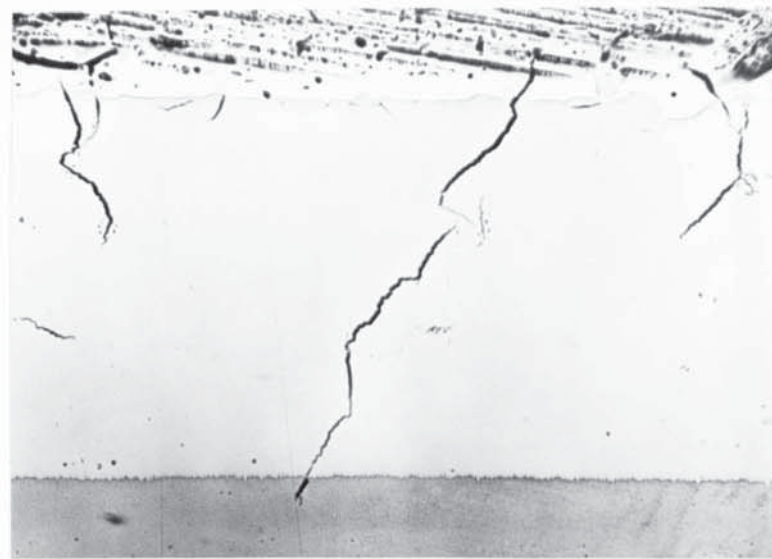
Fig.82. Taper sections of 'composite' chromium/cobalt-nickel coatings showing cracks propagating through cobalt-nickel layer into the die steel.
