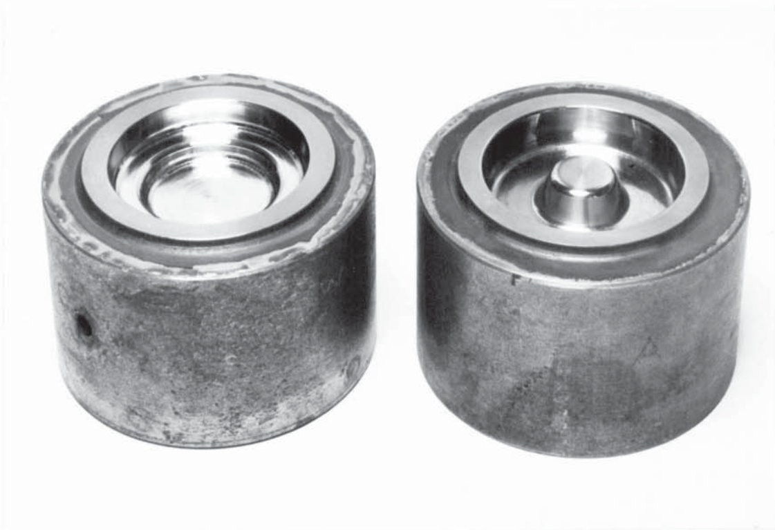
Fig.18. Photograph showing large shaped dies. Approximately three-quarters actual size.
