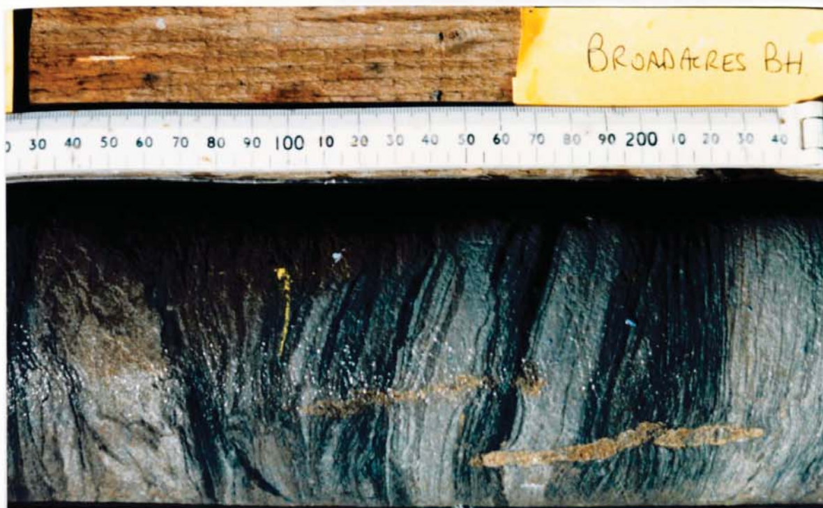
Plate 5.32 Lithofacies 9.1 subseatearth grey. Location: Broadacres Borehole. Age: Westphalian A. The original lithofacies Sandstone wavy stratified is clearly visible together with vertical sideritised root casts which resemble burrows.
