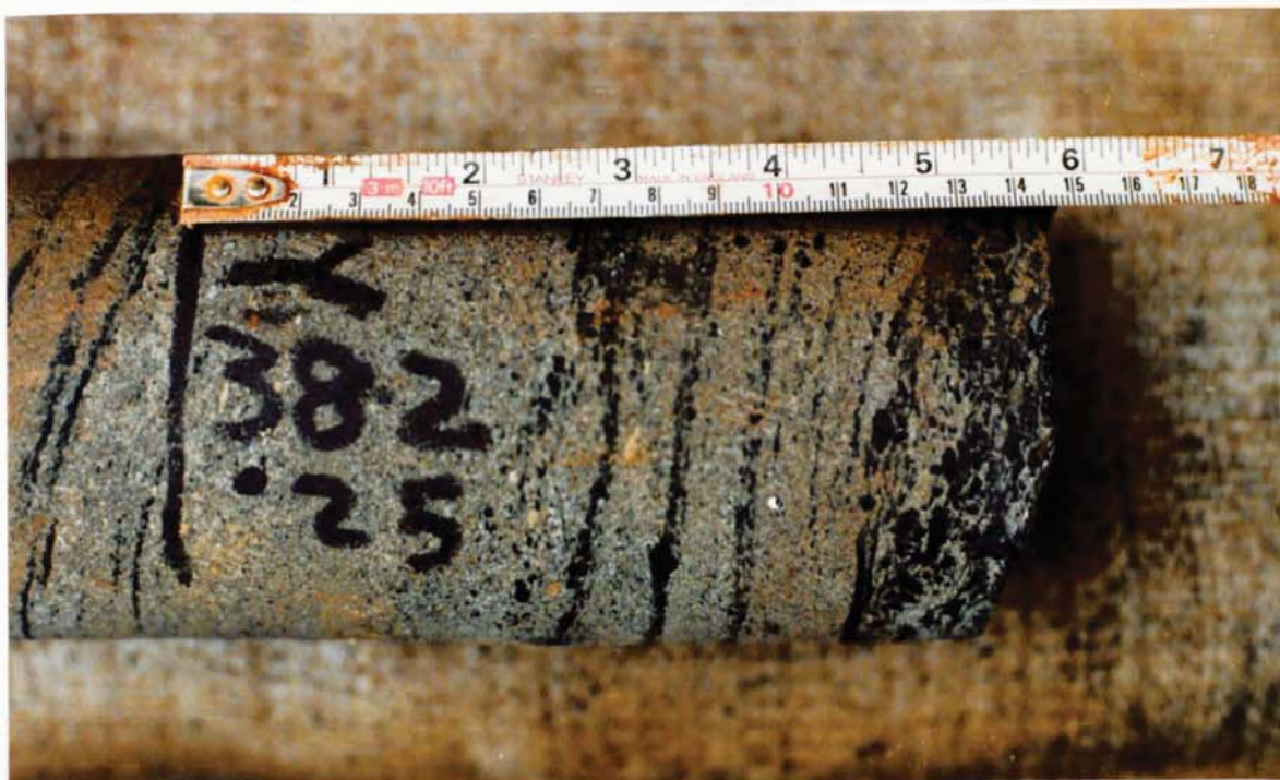
Plate 5.24 Lithofacies 6.1 Conglomerate, intraformational Location : Solomons Temple Borehole. Age : lower Westphalian D. Granule and pebble size coal clasts in a coarse grained sandstone matrix.
