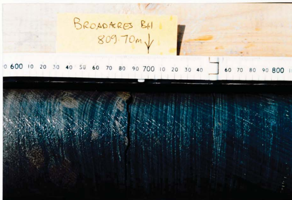
Plate 5.5 Lithofacies 3.3 Siltstone parallel stratified with sandstone. Location: Broadacres borehole. Age: mid Westphalian A
