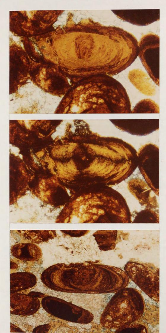
Plate 2.28a Slivers of goethite occur within the yellow-brown chamosite of ooid centres. Stained section, PPL, x125.
