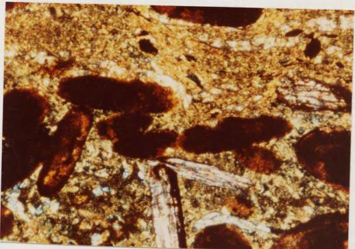
Plate 2.35 Ferroan calcite (blue) and rare siderite (white, greenish white) polygons, dominantly equilateral and isosceles triangles, set in authigenic chamosite. Stained sections, PPL, x200, x125.
