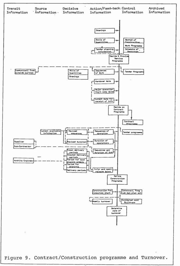
Preliminary preparations to placing the orders and nomination of sub-contractors and suppliers include assessment of plant, material and sub-contractor requisition, available internal resources and their costs.
