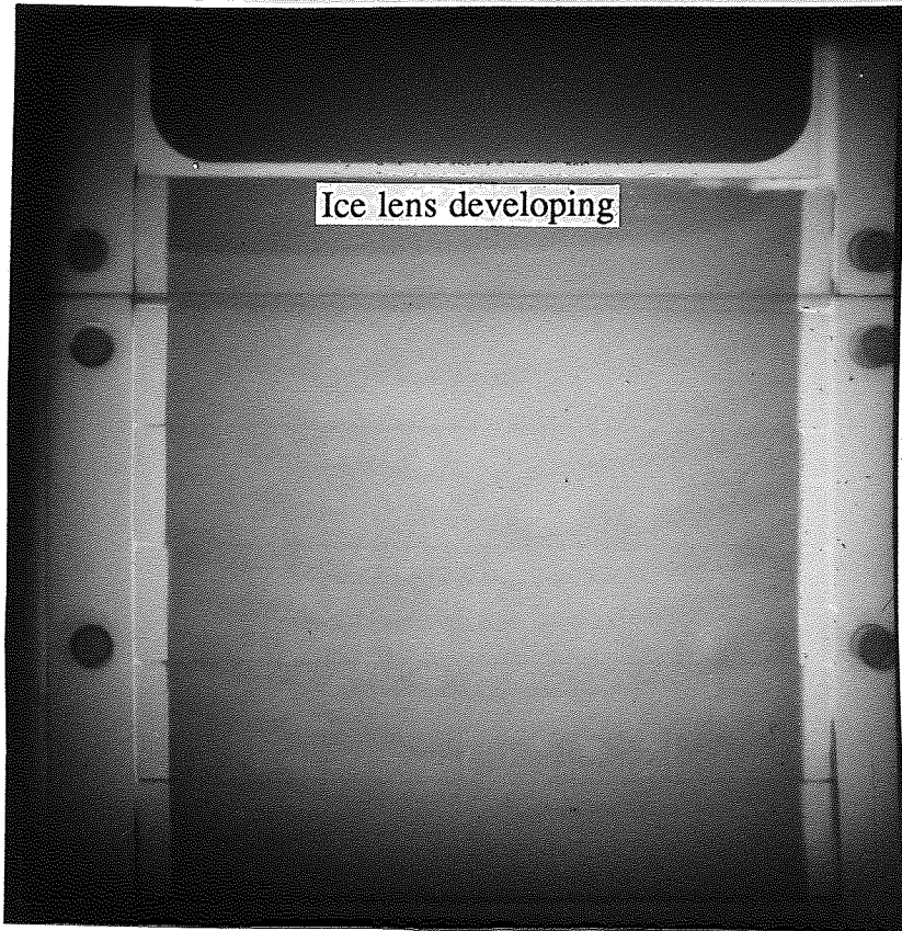
Plate 11 – Standardised Test (Time: 60 min., Heave: 0 mm, Temp.: -2.5 degrees C)
