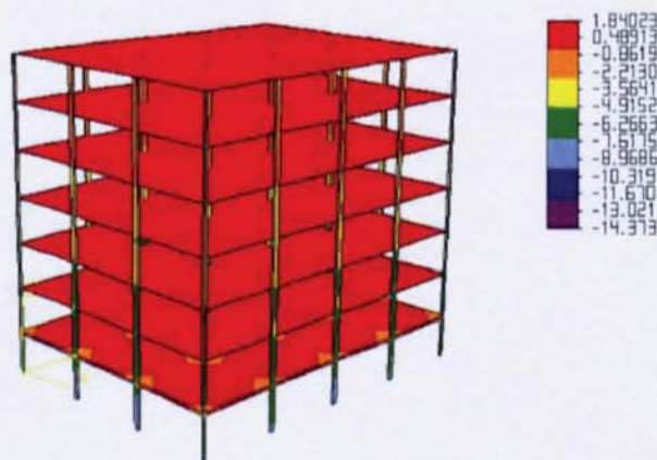
Figure 6.9 Distribution of the stress in z-direction (MPa)
