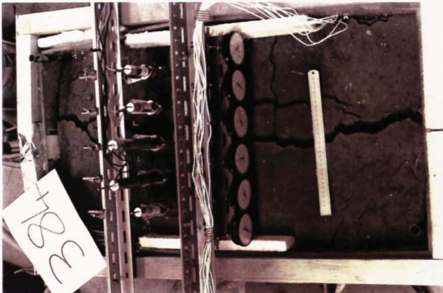
PLATE 8.7 Photograph Showing the Extent of Ground Cracking After 384 hours During the Tatsfield Test.
