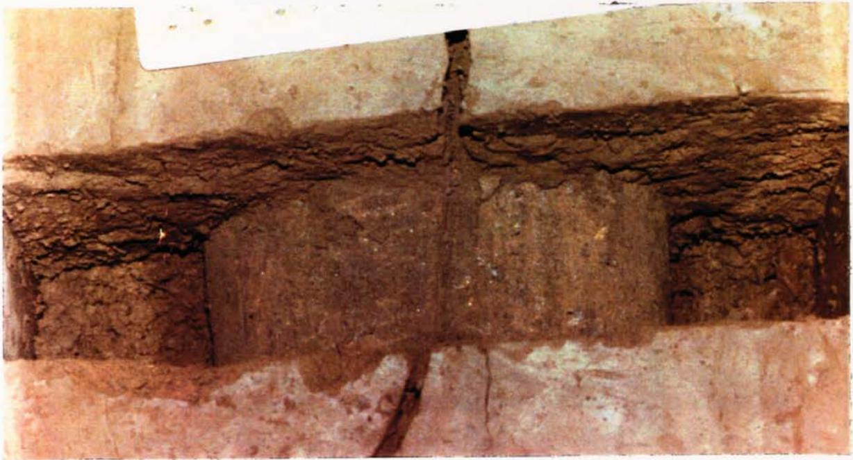
PLATE 8.2 Photograph Showing the Shape Frozen Annulus above the Pipe and the Ground Crack Above the Annulus at the end of the Final Validation Test.
