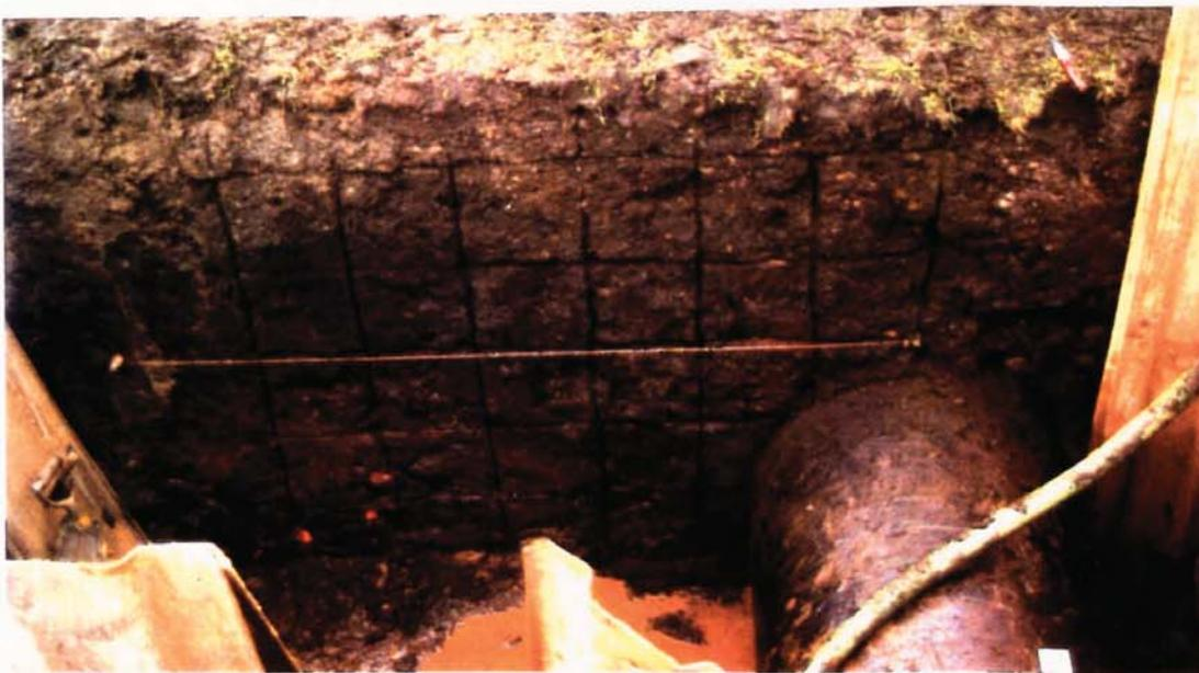
PLATE 7.2 300 x 300 mm Grid Marked on Trench Wall at Site C.
