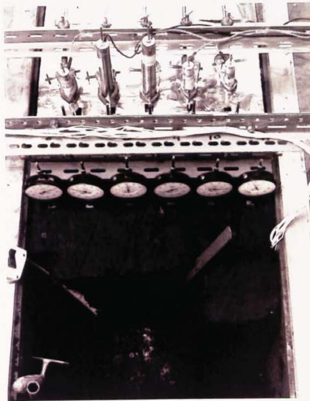
PLATE 8.14 Photograph of Soil Failure Pattern 200 mm from the End of the Tank Closest to the Normal Camera Position (Figure 8.8).
