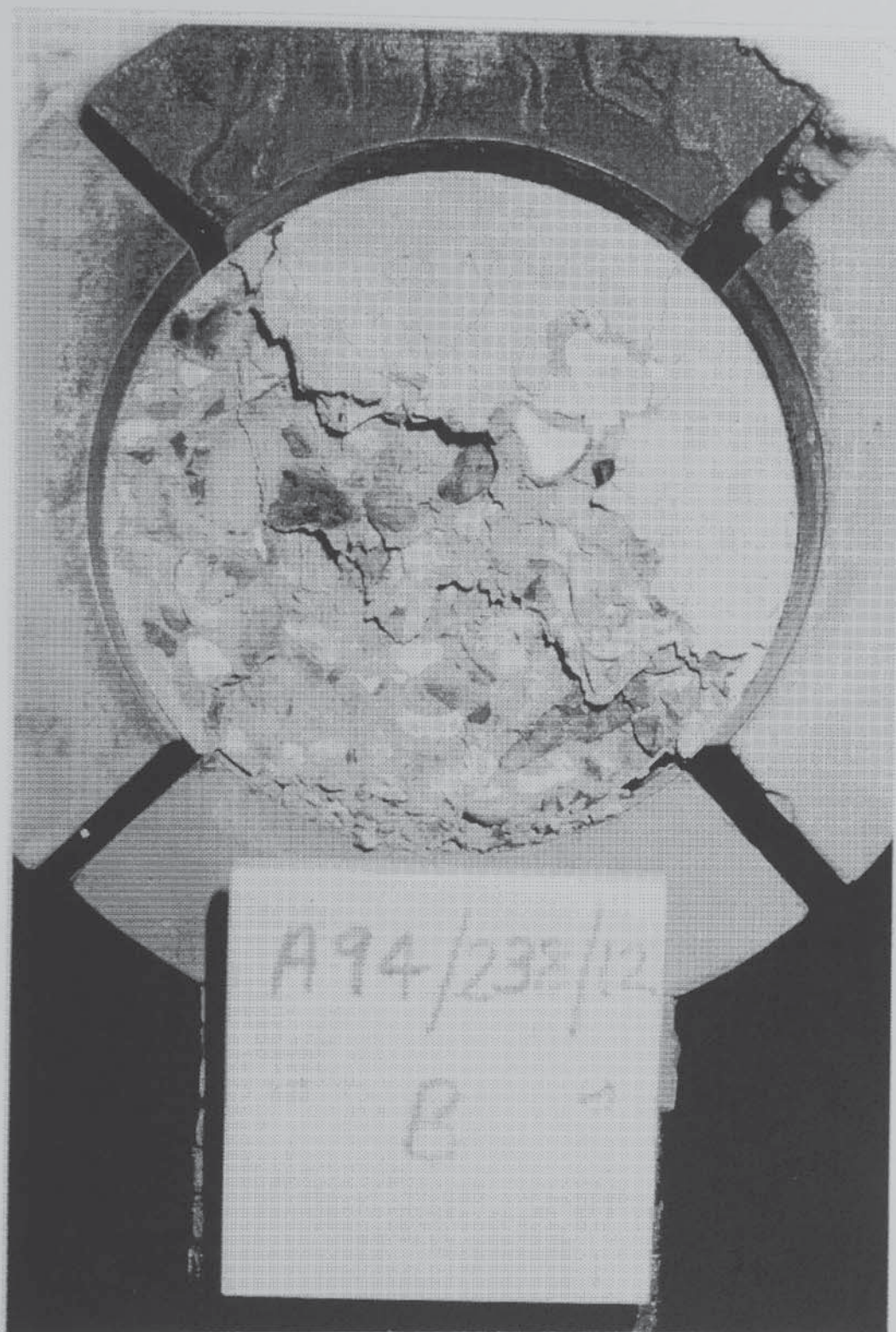
Plate 6.6 Partial explosive spalling
