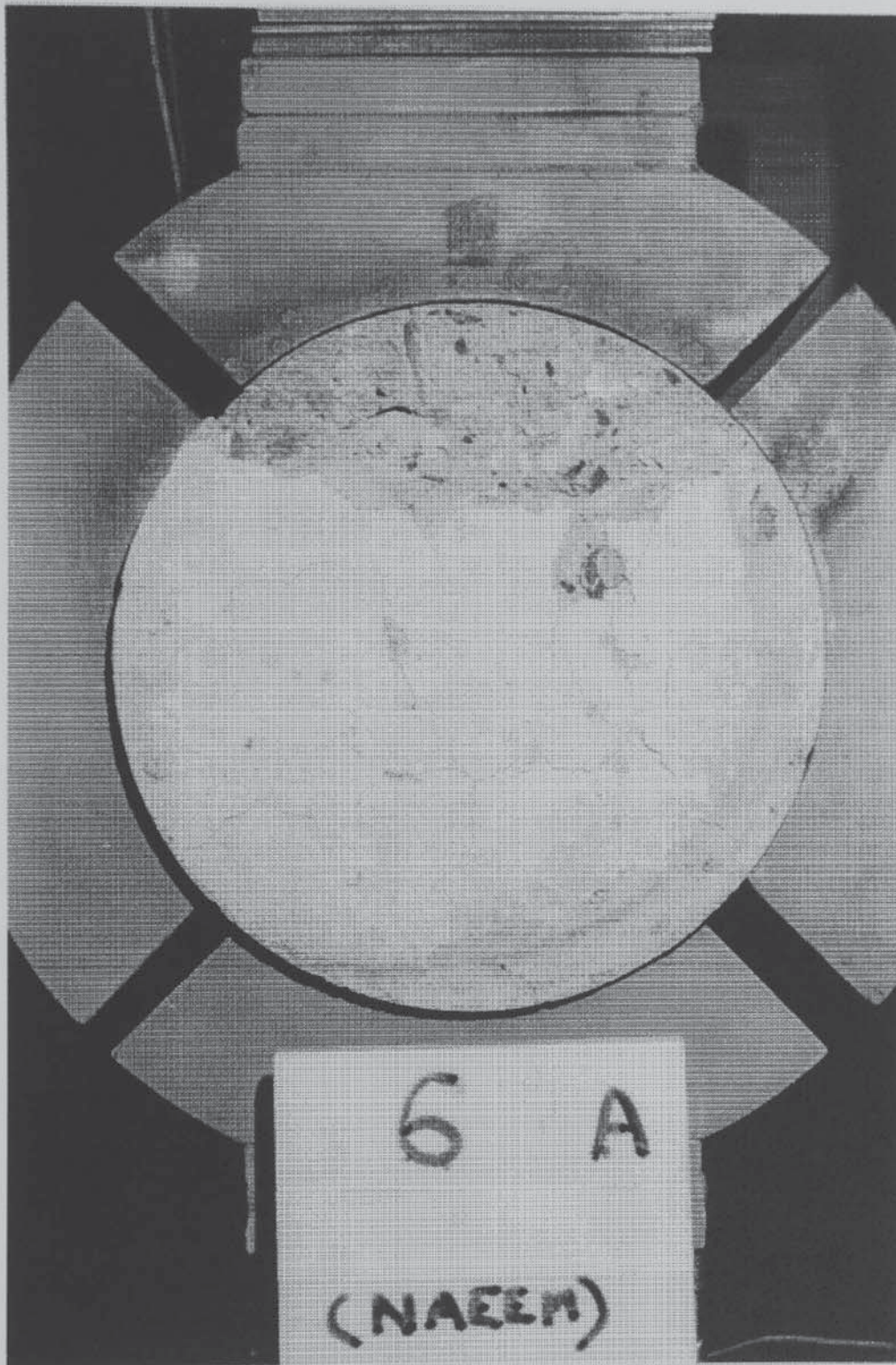
Plate 6.5 An example of surface spalling
