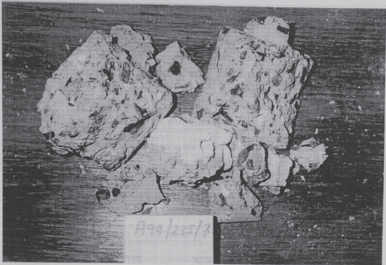
Plate 6.10 Complete destruction of concrete specimens by explosive spalling
