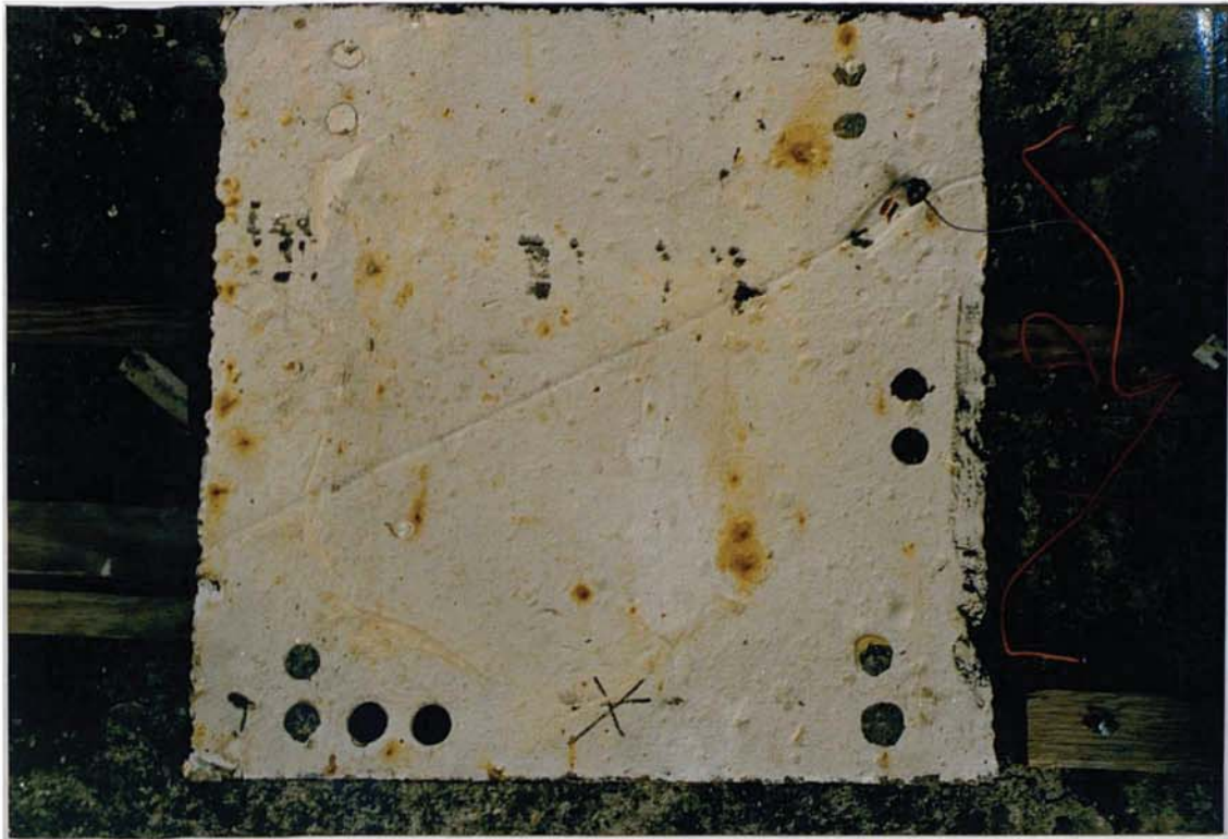
Plate 6.5 Specimen P:2:50:1, 8 months: Heavy rust spotting, bleaching, few micro and macro bubble sites.
