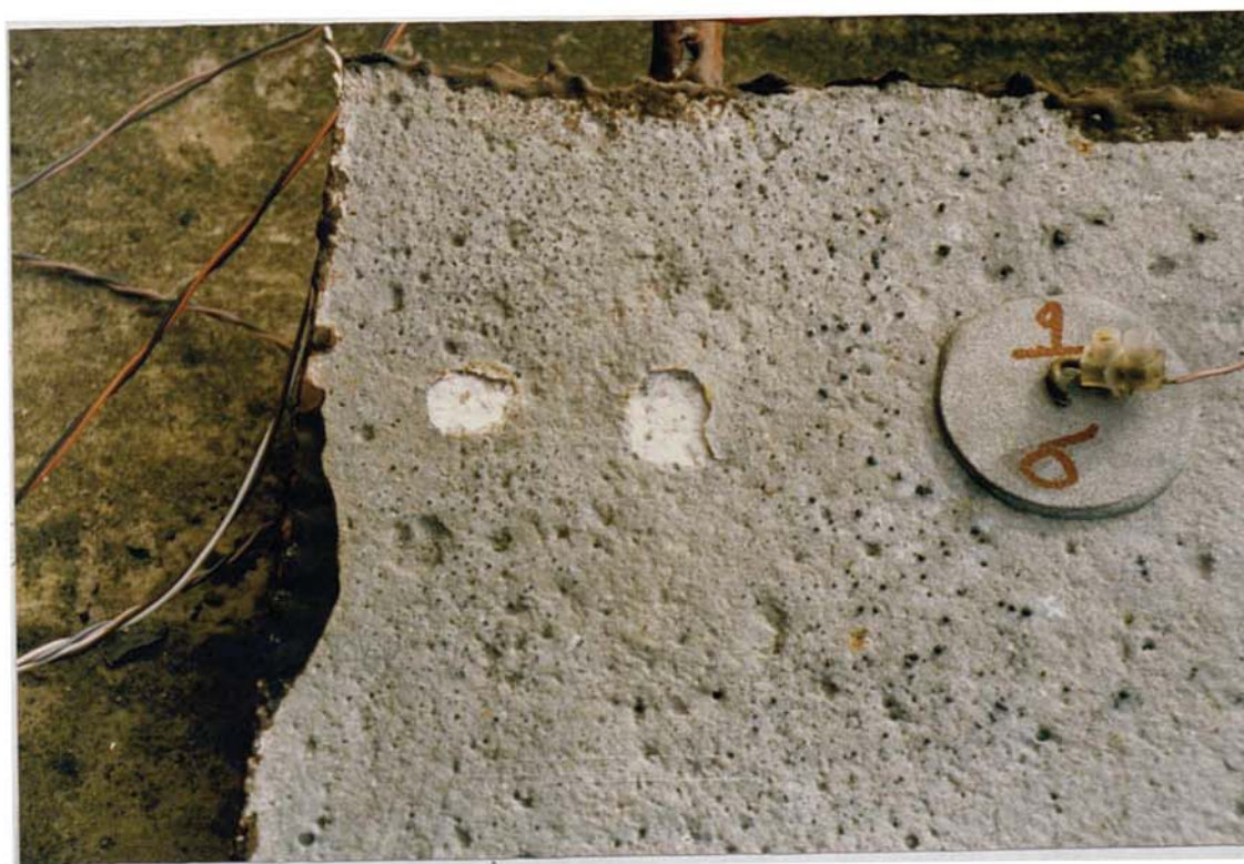
Plate 6.16 Specimen Z:2:50:1, 8 months: Surface "warts" and "white rust" formation over zinc pull-off sites.
