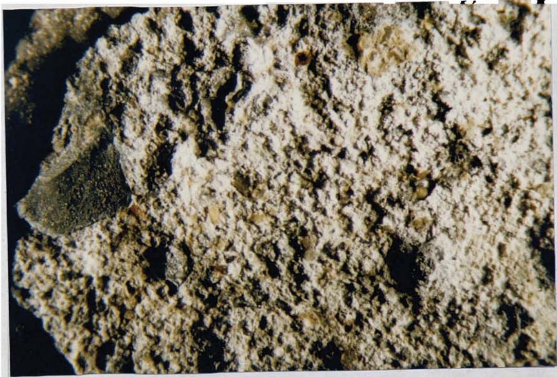
Plate 6.22 Specimen Z:2:50:1, 4 months: Type 5 failure. (10 mm = 1.07 mm)
