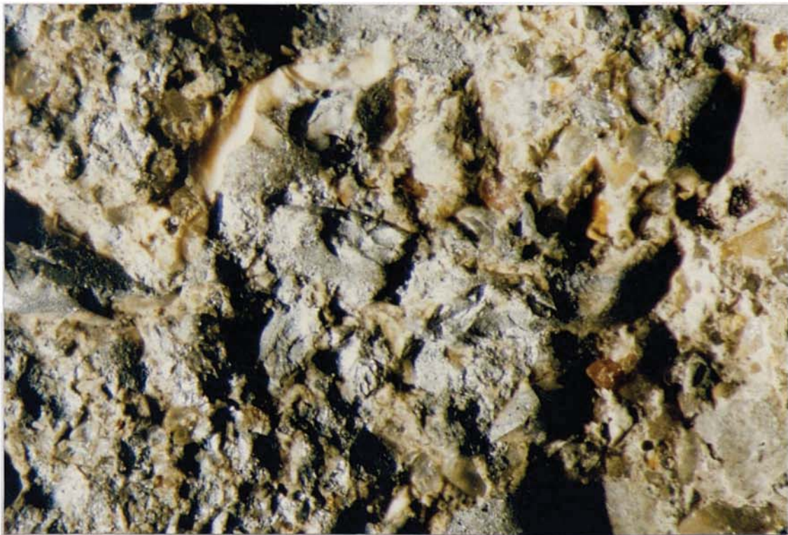
Plate 6.20 Specimen Z:2:0:1, 4 months: Type 2 failure: zero degradation case. (10 mm = 1.07 mm)
