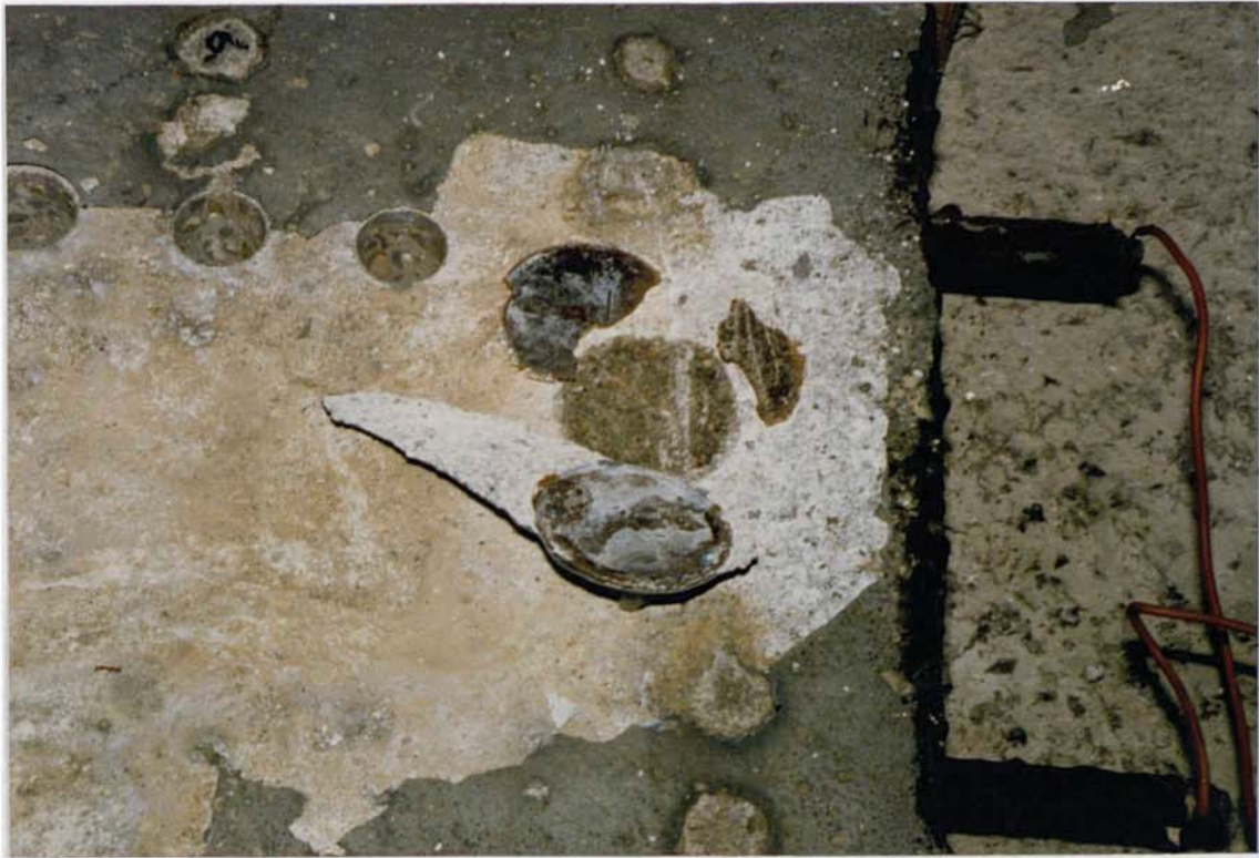
Plate 6.19 Specimen Z:2:50:1, 18 months: Central area has debonded, good primary anode/epoxy resin/substrate bond. Brown dust from previous coring.
