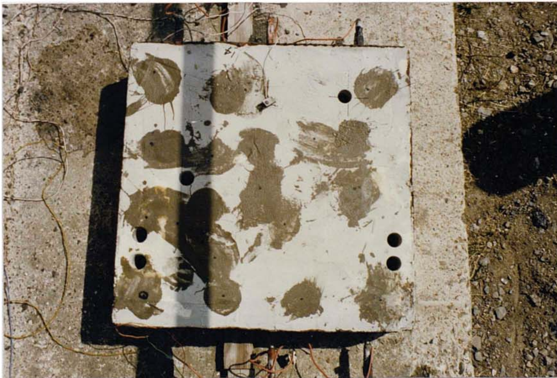
Plate 6.2 Specimen E:2:50:2: location of USPV (Pundit) measurements using flat transducer heads.
