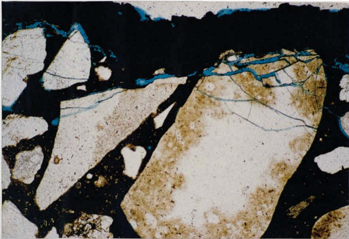
Plate 8.7 Specimen Z:2:50:1, 3 months, shattered surface aggregate, zinc thickness \approx 340 \mu\text{m} . (scale 10 mm = 171 \mu\text{m} )
