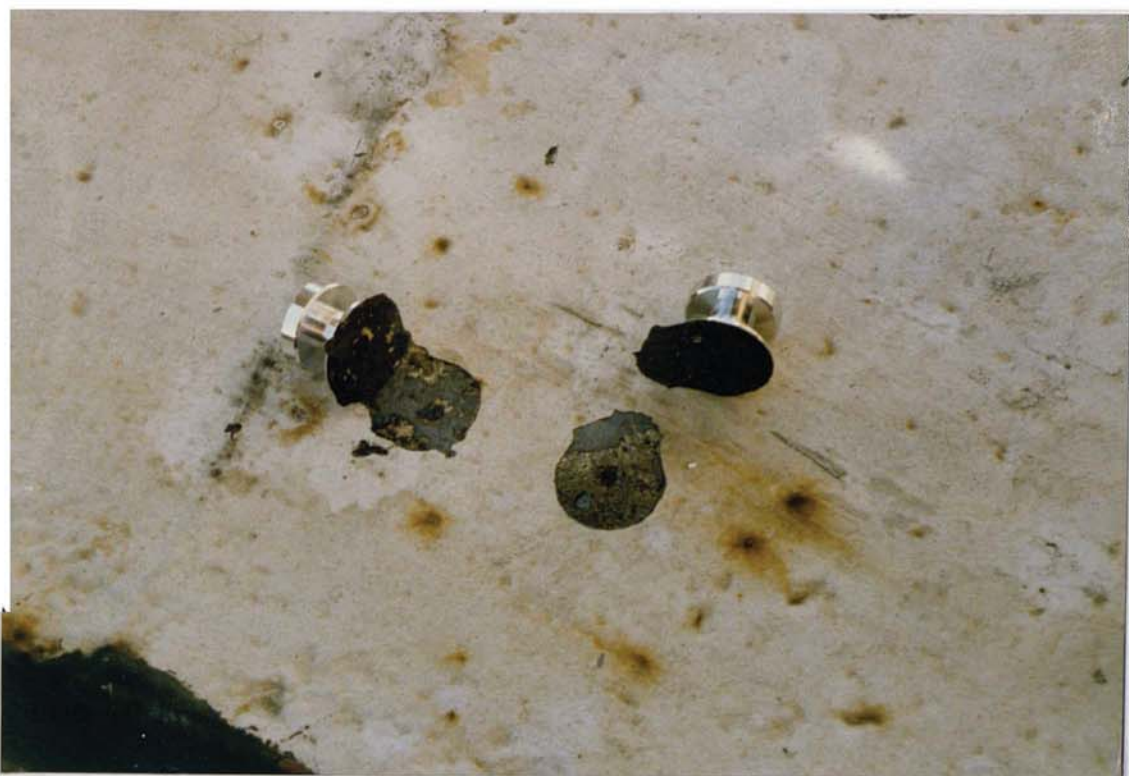
Plate 6.7 Specimen P:0.4:20:1, 18 months: Anode P, type 4 failure.
