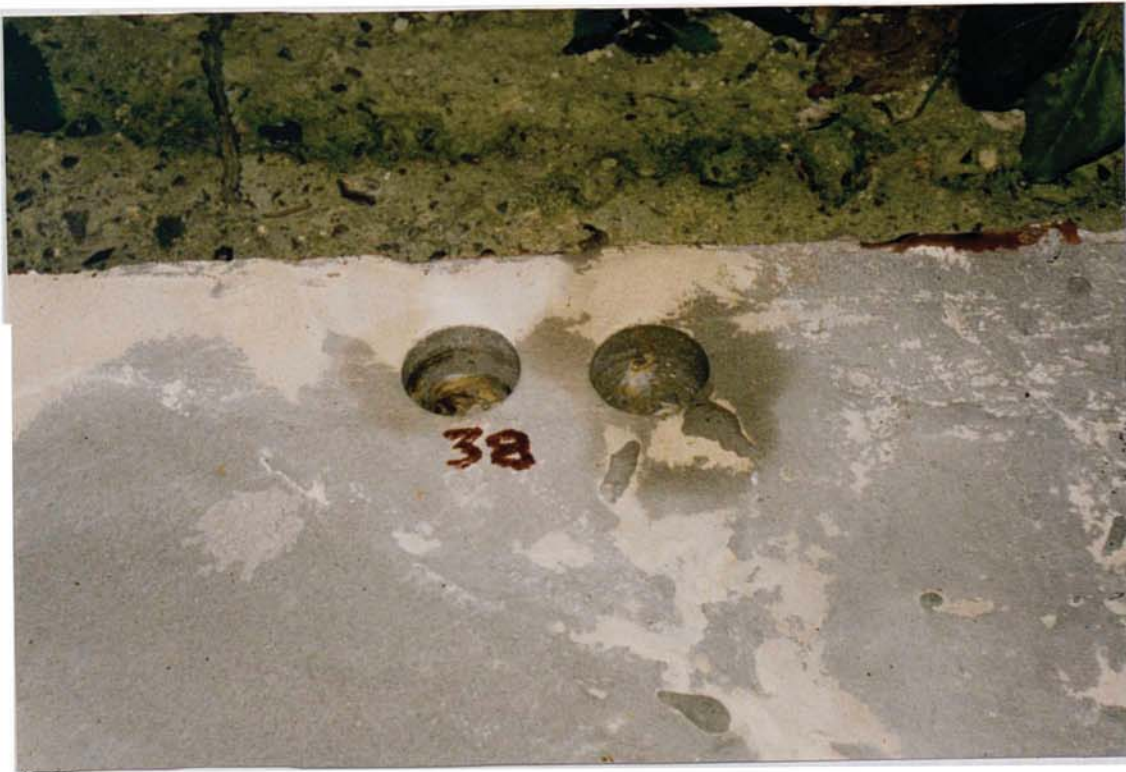
Plate 6.34 Specimen E:0.4:20:2, 8 months. Corrosion products surrounding an anode strand.
