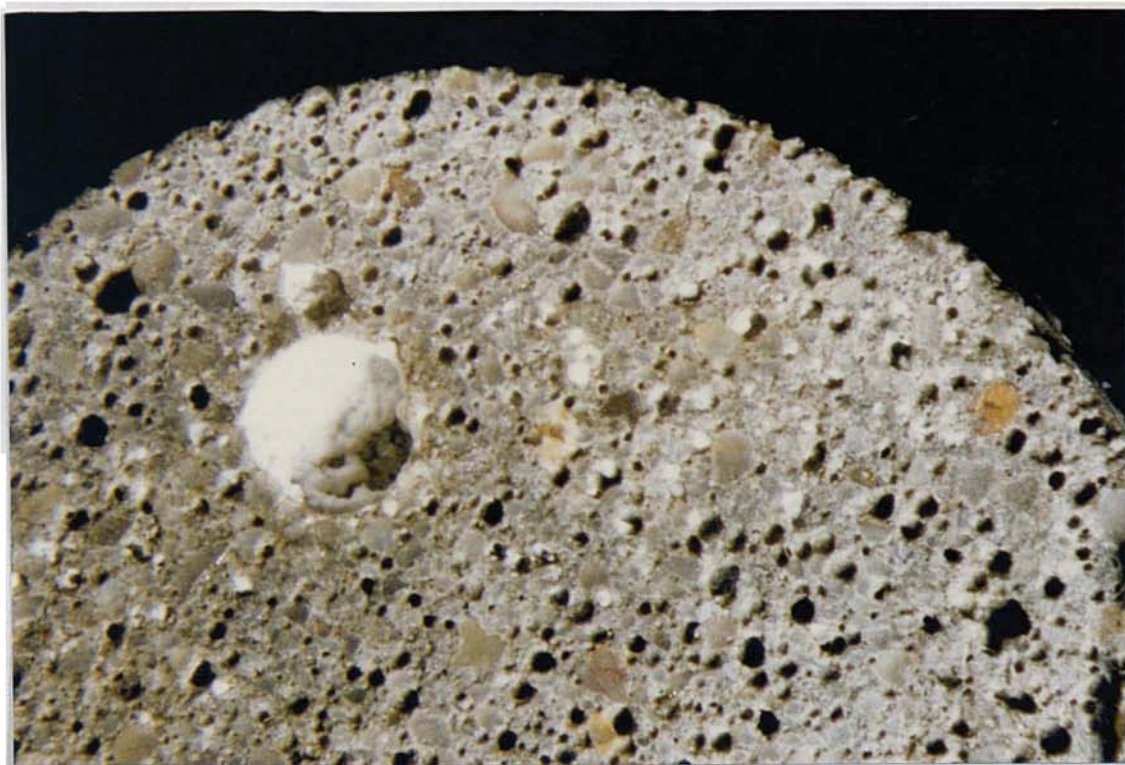
Plate 6.40 Specimen T:2:50:1, 12 months. White crystalline product which precipitated along line of anode strand and within macro void. (10 mm = 1.07 mm)
