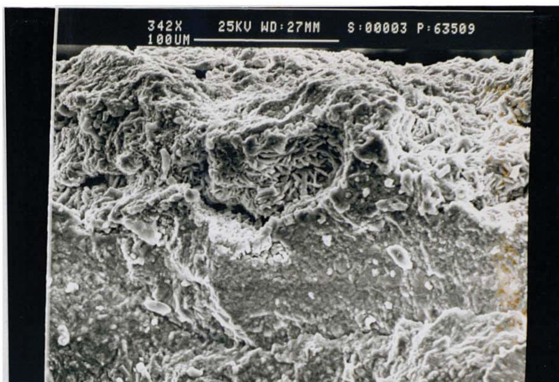
Plate 6.31 SEM micrograph of zinc fracture surface, specimen Z:2:50:1.
