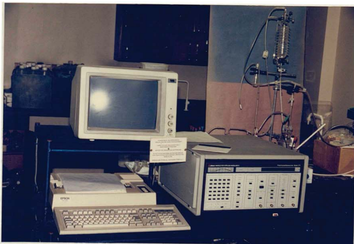
Plate 4.2 Potentiostat during an experiment; Nylox deoxygenator in the background.
