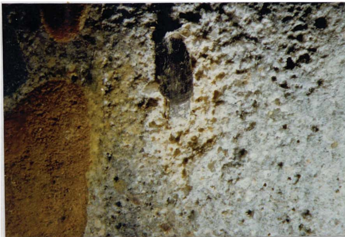
Plate 6.37 Specimen T:2:50:1, 9 months. Type 4/5 degradation, rust staining of paste on left associated with aggregate. (10 mm = 1.07 mm)
