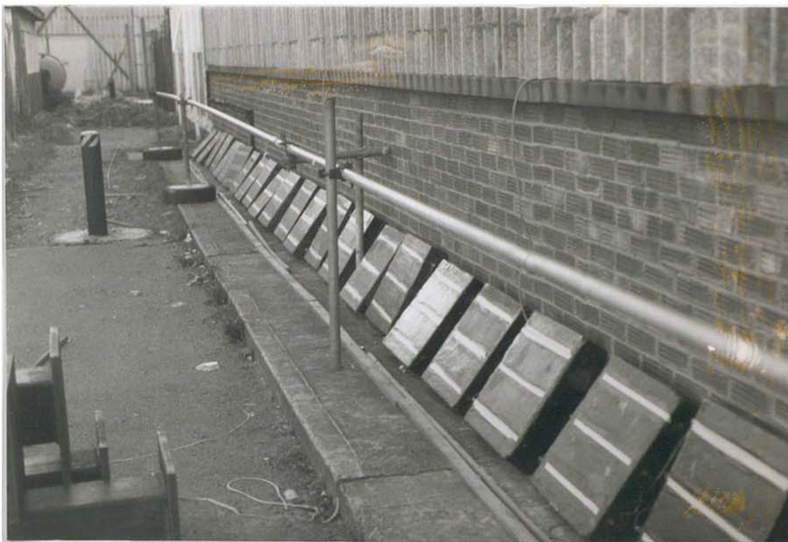
Plate 7.1 Arrangement of slabs during cathode potential measurements.
