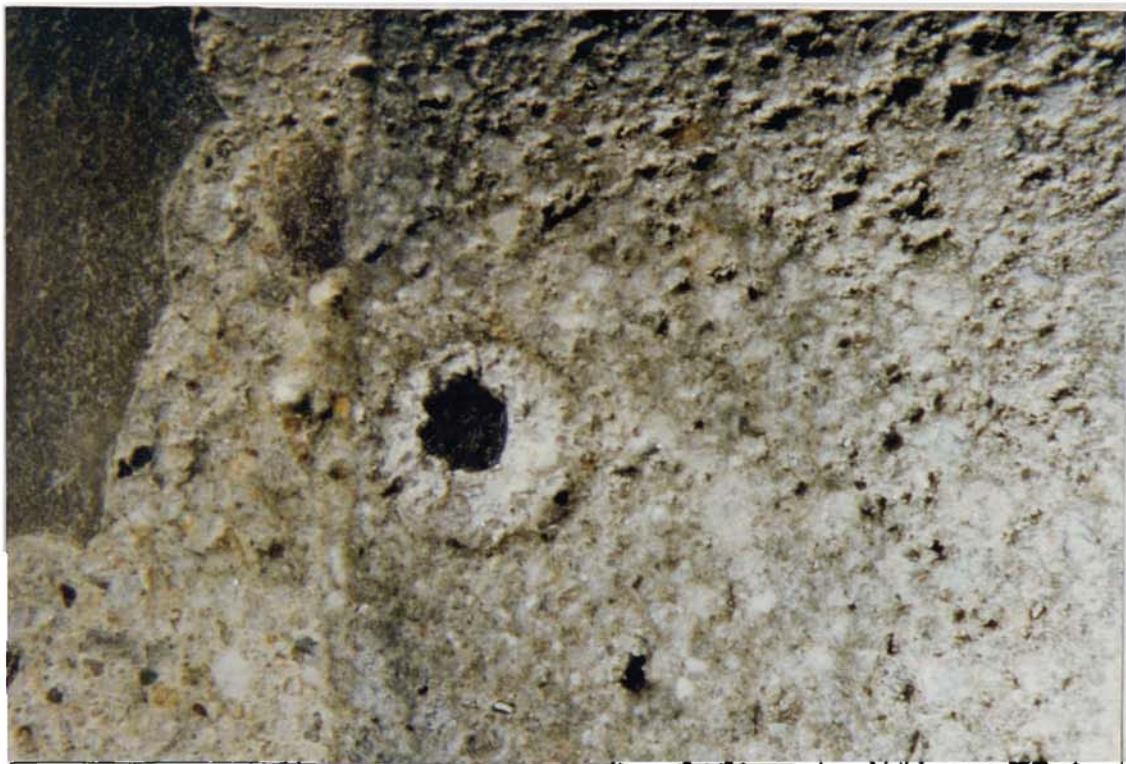
Plate 6.36 Specimen E:4:20:1, 9 months. Type 2/3 degradation, reduced porosity in anode strand region. (10 mm = 1.07 mm)
