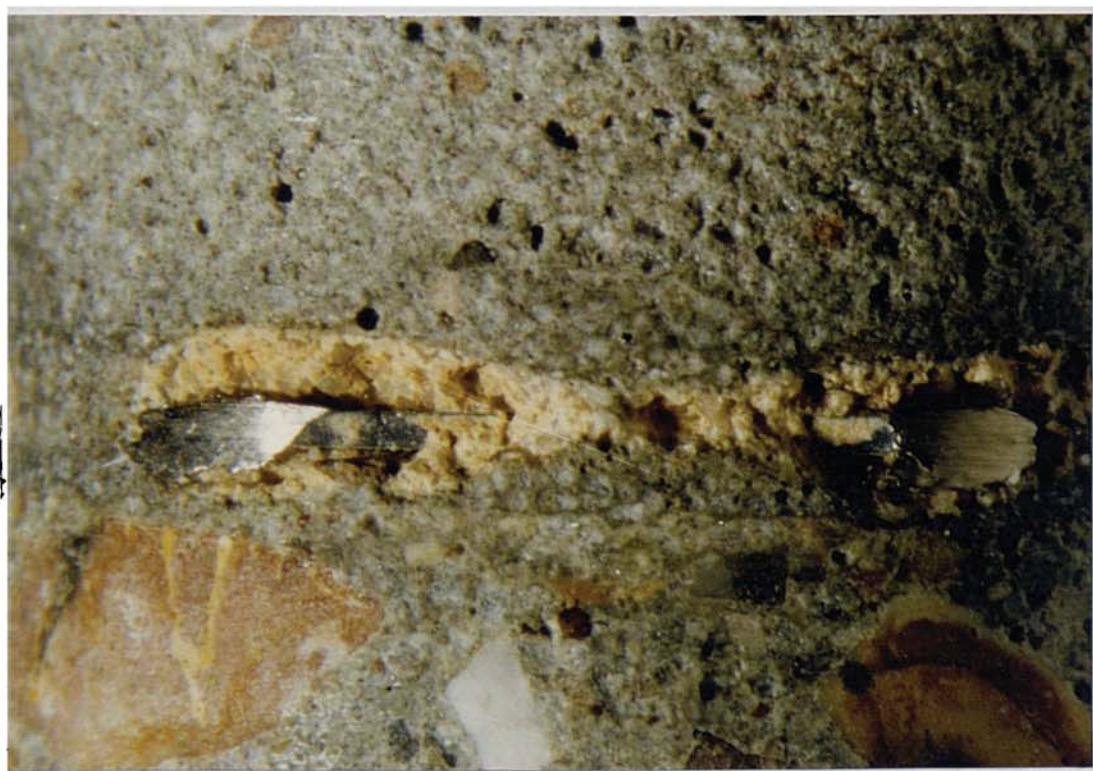
Plate 6.38 Specimen E:2:50:1, 9 months. Type 5 degradation in cored specimen. (10 mm = 1.07 mm)
