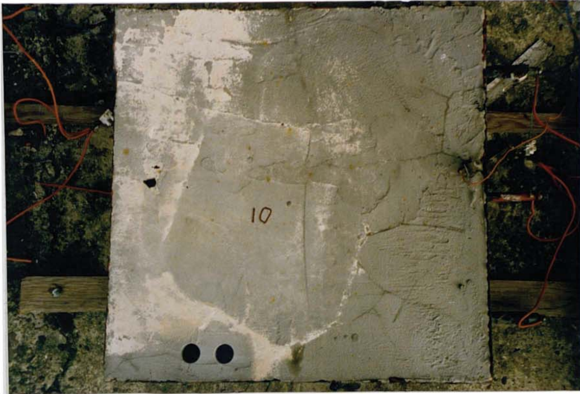
Plate 6.33 Specimen E:2:50:1, 8 months. Drying shrinkage cracking of cementitious overlay and light rust spotting.
