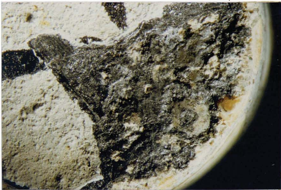
Plate 6.12 Specimen P:2:50:1, 9 months: View of a cored bubble site, with bubble removed. (scale 10 mm = 1.07 mm)
