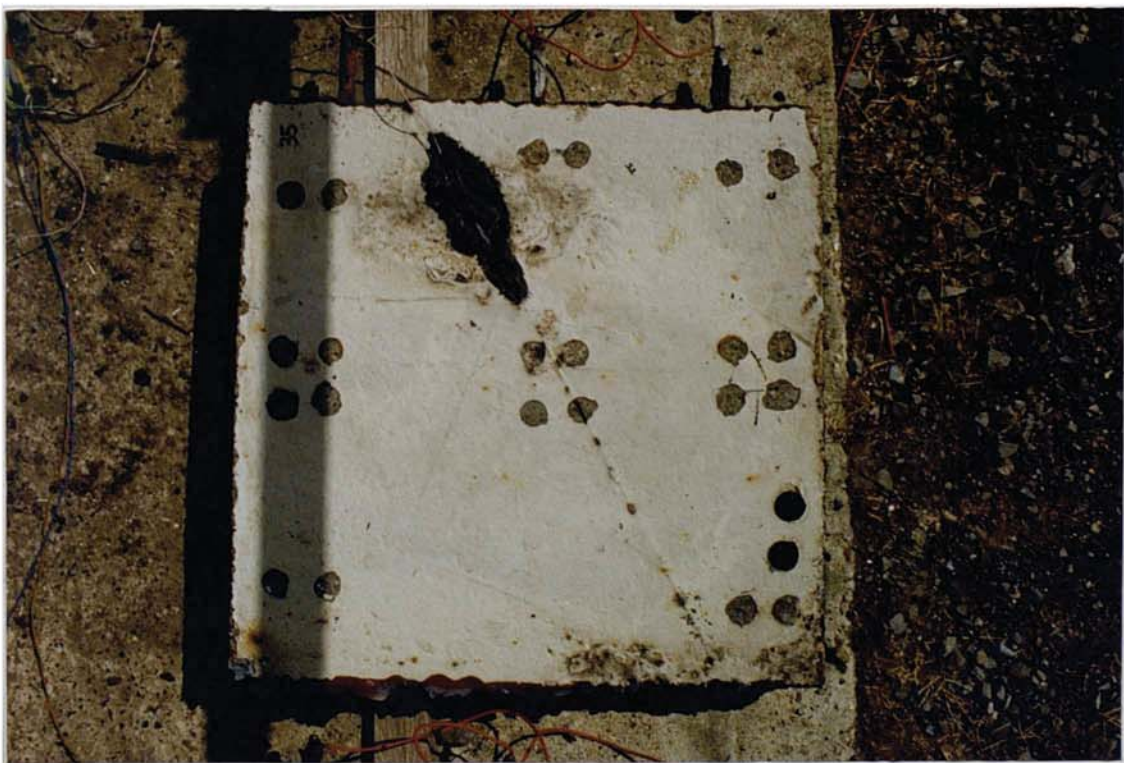
Plate 6.4 Specimen P:0.4:50:1, 18 months: Repaired anode region, degradation has spread further. Majority of the surface is unaffected. Low rust spotting.
