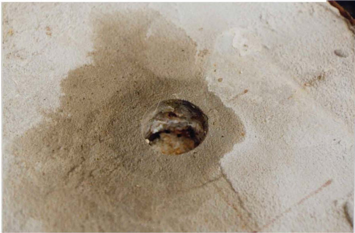
Plate 6.35 Specimen E:2:50:2, 22 months. Carbonate precipitation within cored hole.
