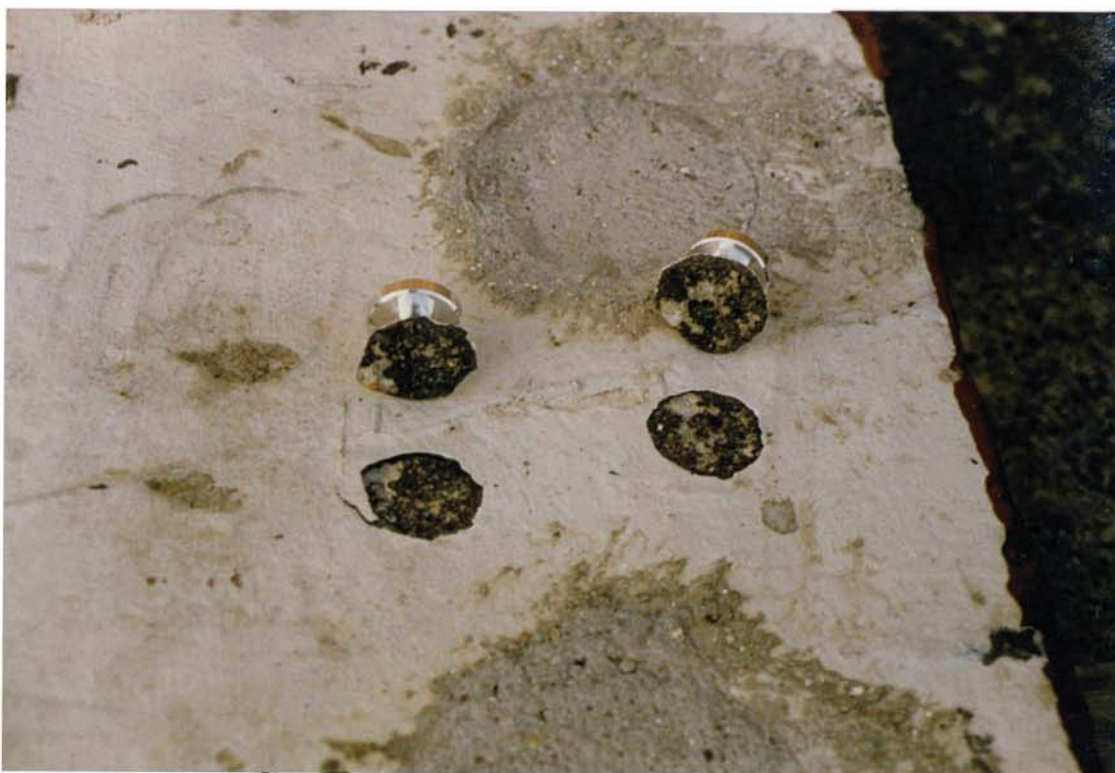
Plate 6.9 Specimen P:0.4:0:1, 18 months: Anode P, type 2 failure.
