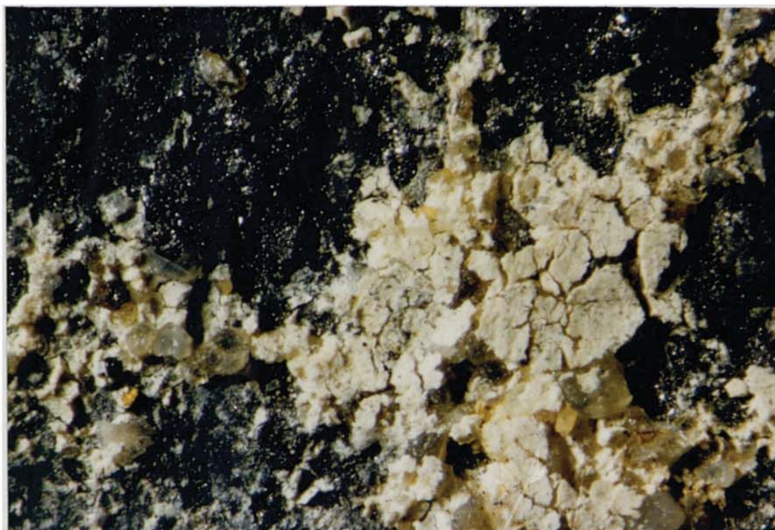
Plate 6.13 Specimen P:2:50:1, 9 months: View of acidified cement paste adhering to disbonded coating. (scale 10 mm = 1.07 mm)
