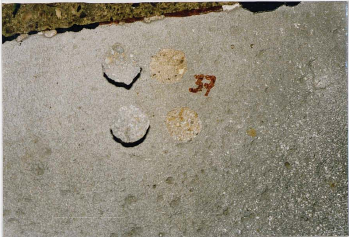
Plate 6.21 Specimen Z:0.4:20:2, 8 months: Type 3 failure (upper dolly) and type 4 failure (lower dolly).
