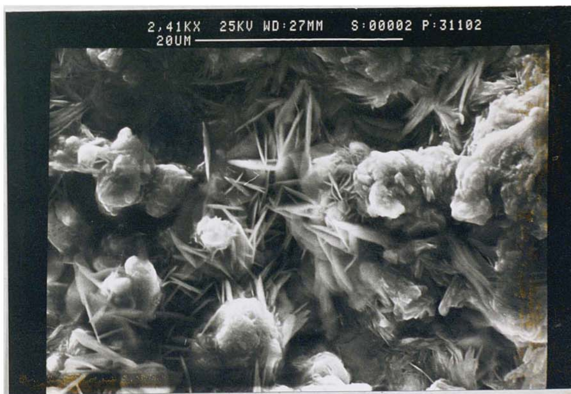
Plate 6.26 SEM micrograph of zinc wart corrosion product, inner surface.
