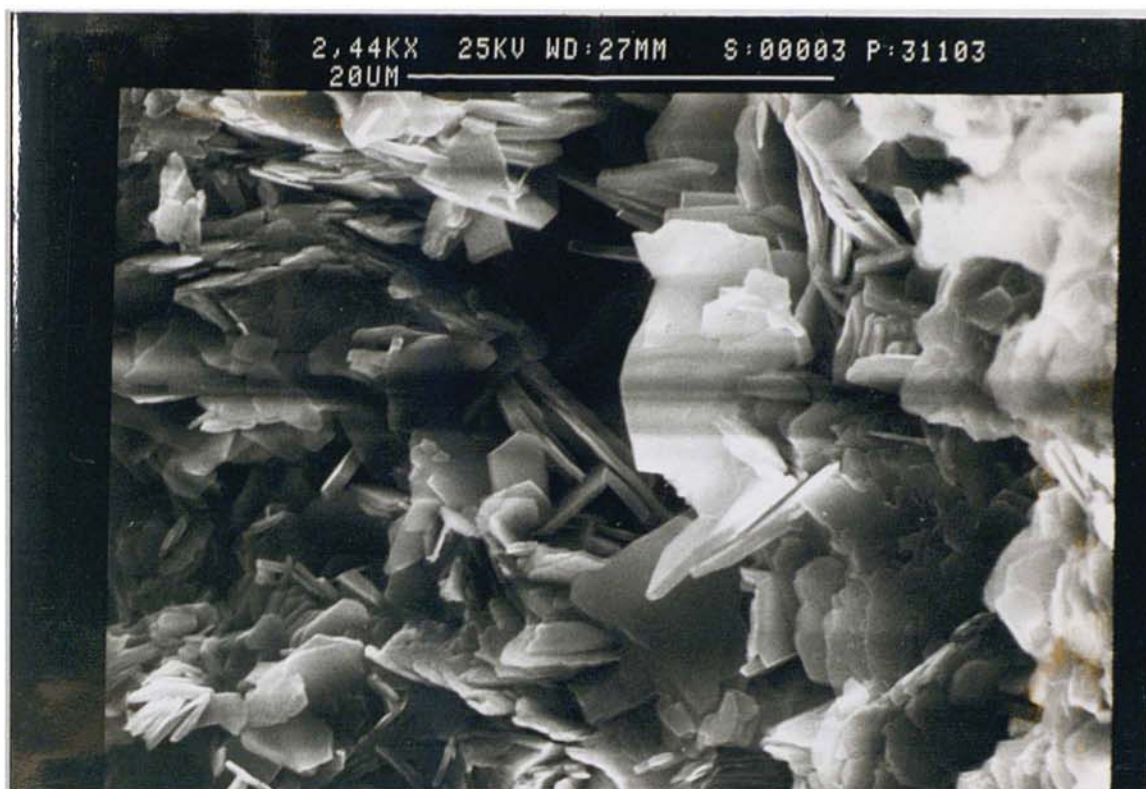
Plate 6.27 SEM micrograph of zinc wart corrosion product, inner surface.
