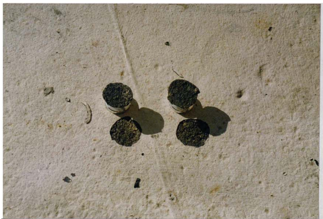
Plate 6.8 Specimen P:2:20:1, 18 months: Anode P, type 3 failure.
