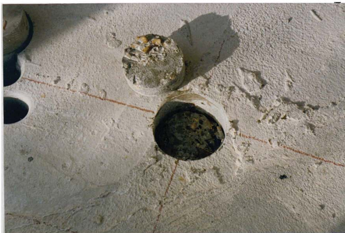
Plate 6.42 Specimen E:2:50:1, 18 months. Overlay adhesion test (Limpit), failure at the overlay/substrate interface.
