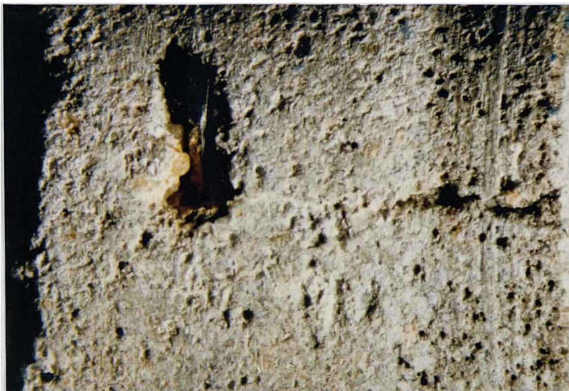
Plate 6.39 Specimen E:2:50:1, 12 months. Type 6 degradation, crack extending from anode to surface is partially filled by a precipitate. (10 mm = 1.07 mm)
