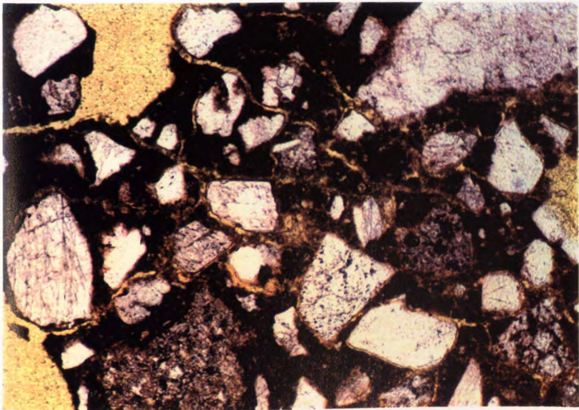
Plate 4.6 - Petrographic Image of Cracking in the Interior of Poned Slabs (Potassium Acetate) x 100 Mag.
