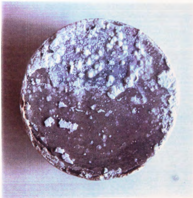
Plate 4.10 - Deposits Precipitated on Diffusion Specimens (Calcium and Magnesium Acetate) x 1.8 Mag.
