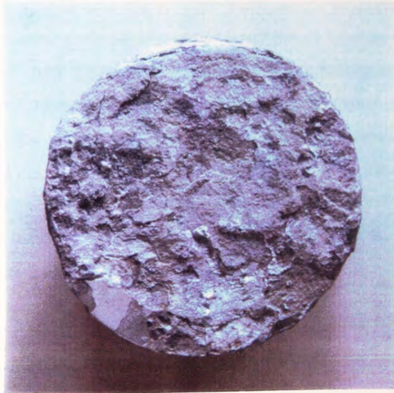
Plate 4.8 - Scaling Damage to Bottom Surface of Partial Immersion Sample (Potassium Acetate) x 1.6 Mag.
