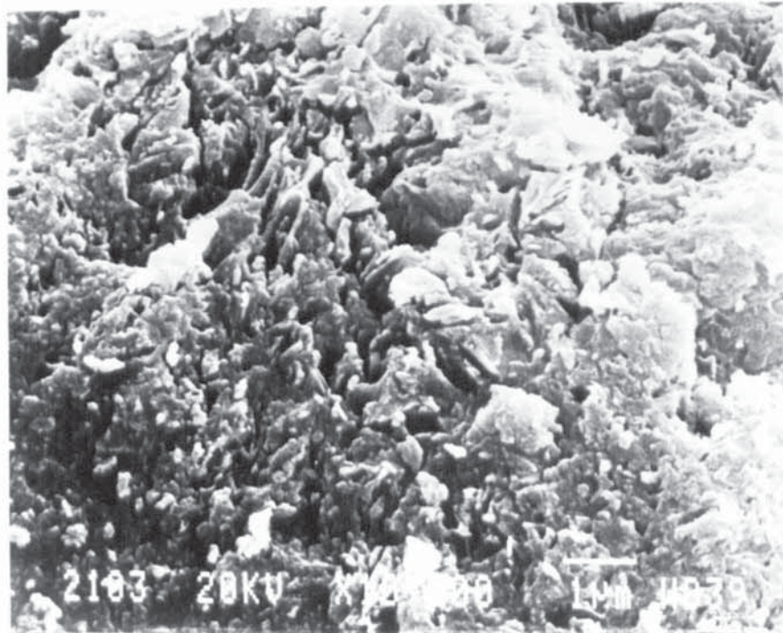
Figure 5.26: Scanning electron micrograph of the uncarbonated portion of silica fume cement mortar specimen contaminated with Cl+SO 4
