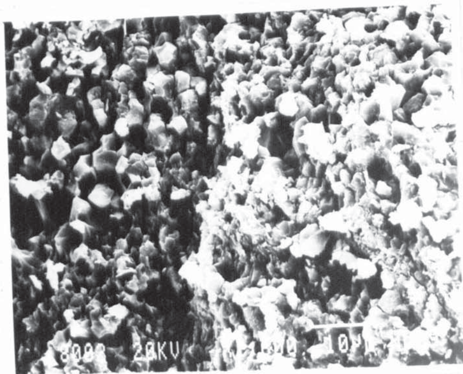
Figure 5.30: Scanning electron micrograph of the uncarbonated portion of BFS cement mortar specimen contaminated with Cl+SO 4
