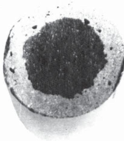
OPC-A ( \text{C}_3\text{A} : 8.5%) MORTAR SPECIMEN CONTAMINATED WITH \text{Cl}^- + \text{SO}_4^{2-} EXPOSURE - 51 WEEKS
