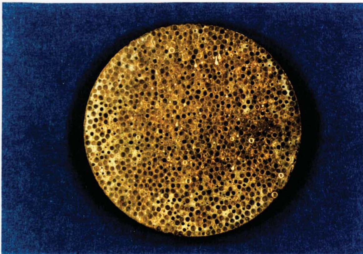
Plate 7.3: Random distribution of glass beads in OPC mortar constituting approximately 48% volume fraction of beads
