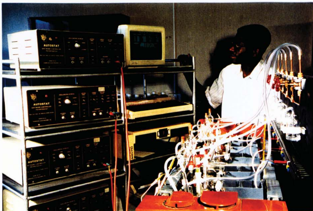
Figure 3.2: Set-up of oxygen diffusion experiment
