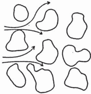
(a) Tortuous diffusion in a porous solid
