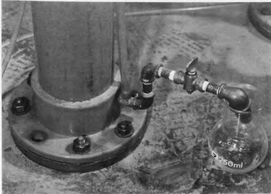
Fig 6.6 Collection of Drainage Water from Soil Columns.
