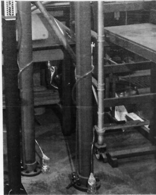
(a) Arrangement for Maintaining a Constant Head.
