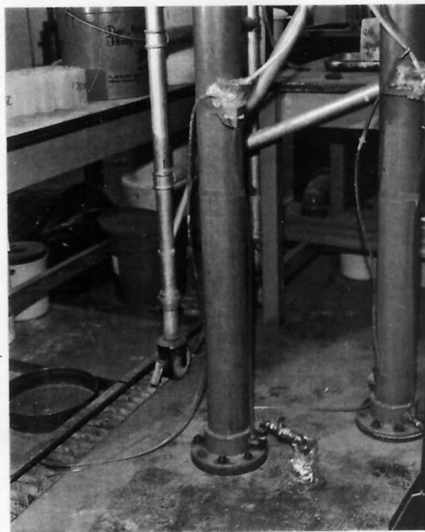
(b) Device for Raising the Column Water Table Level.
