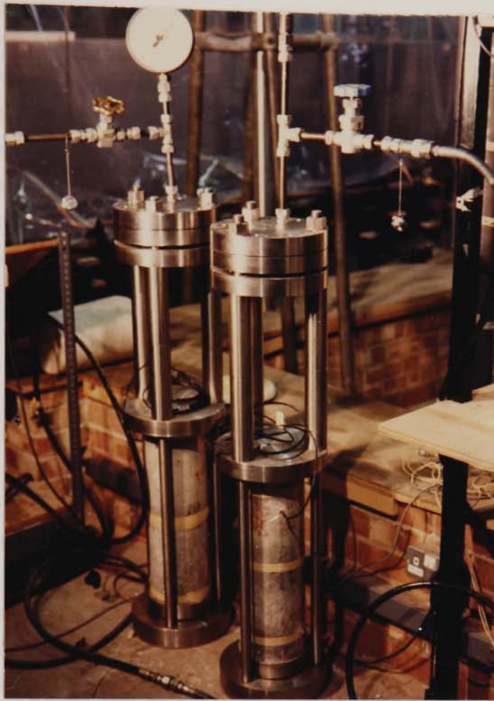
PLATE 6.1. Cylindrical specimens located in the hydraulic loading rigs prior to installation into the cryogenic cabinet.
