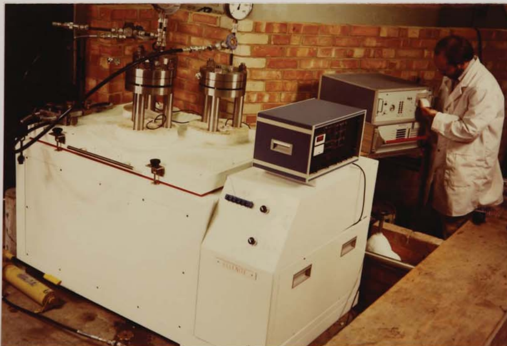
PLATE 6.2. Three loading rigs installed in the cryogenic test rig prior to testing.
