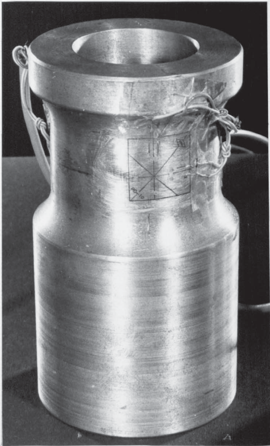
PLATE A2.1 THE DYNAMOMETER WITH THE GAUGE CONFIGURATION
