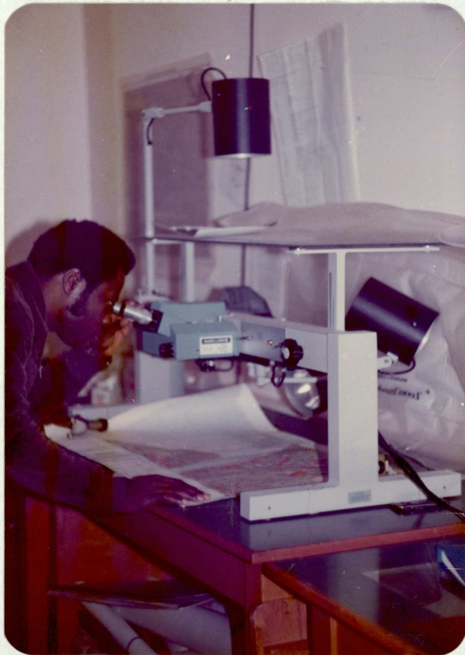
Plate 5.4 The Zoom Transferscope (ZT4-H)
