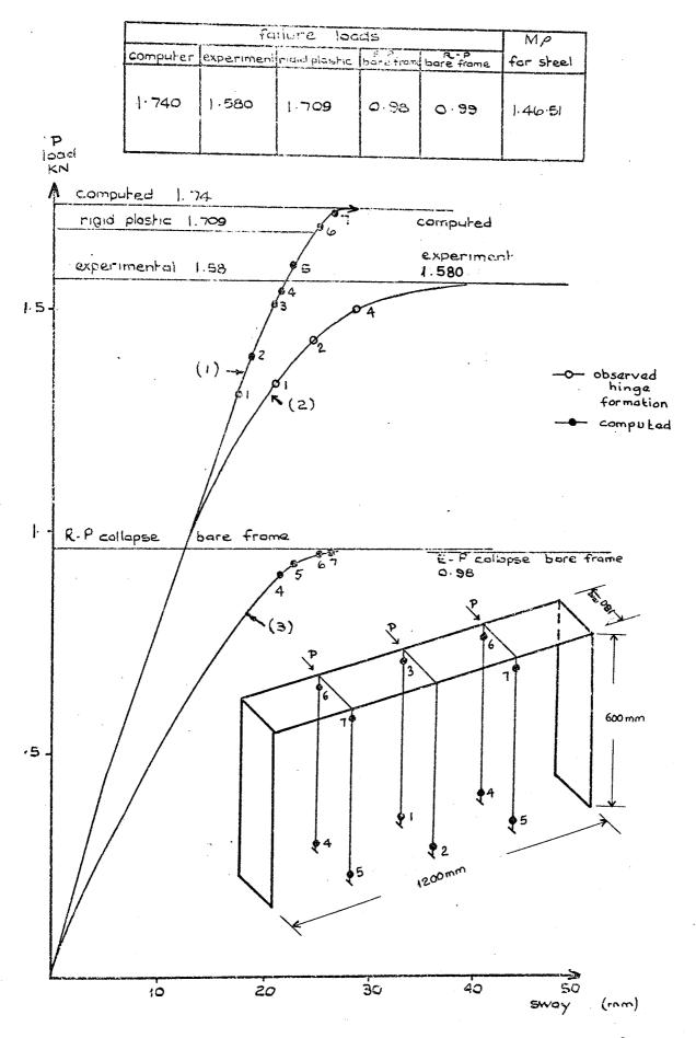
Fig. 5.1 Load - deflexion diagram for structure 2
