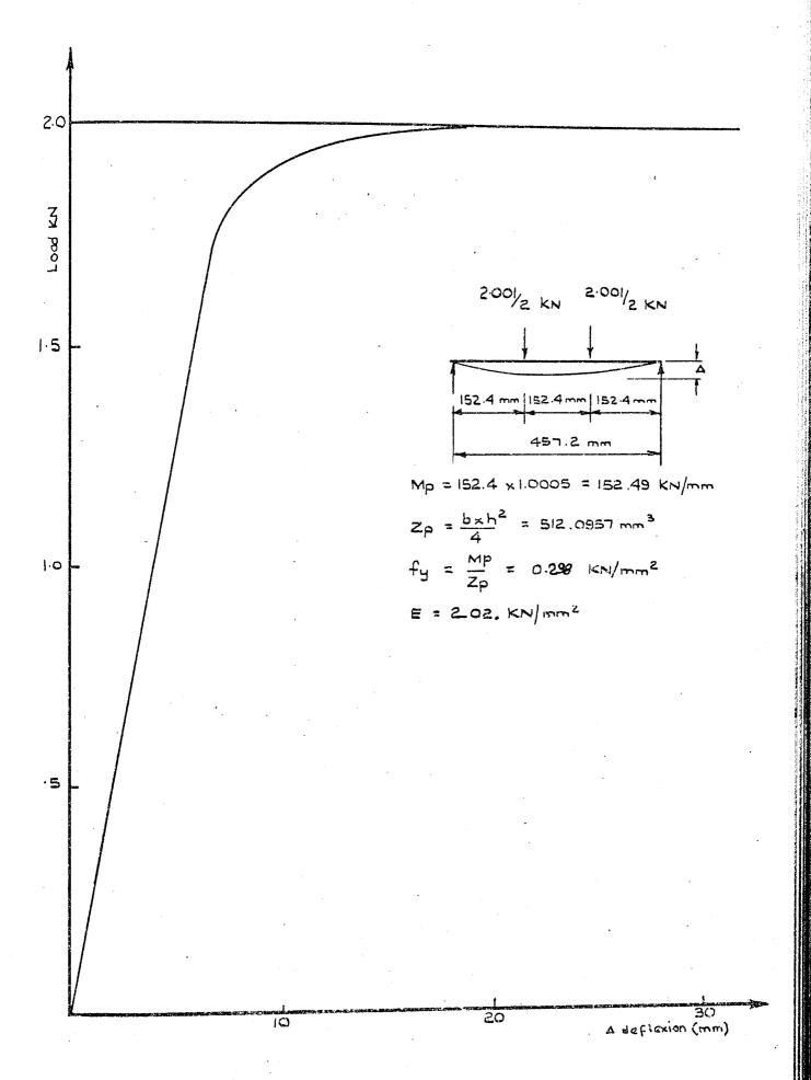
Fig. 4.5 Control test on 12.7 mm x 12.7 mm
