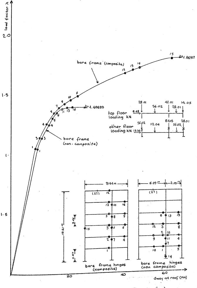
Fig. 6.5 Six storey frame (combined loading)
