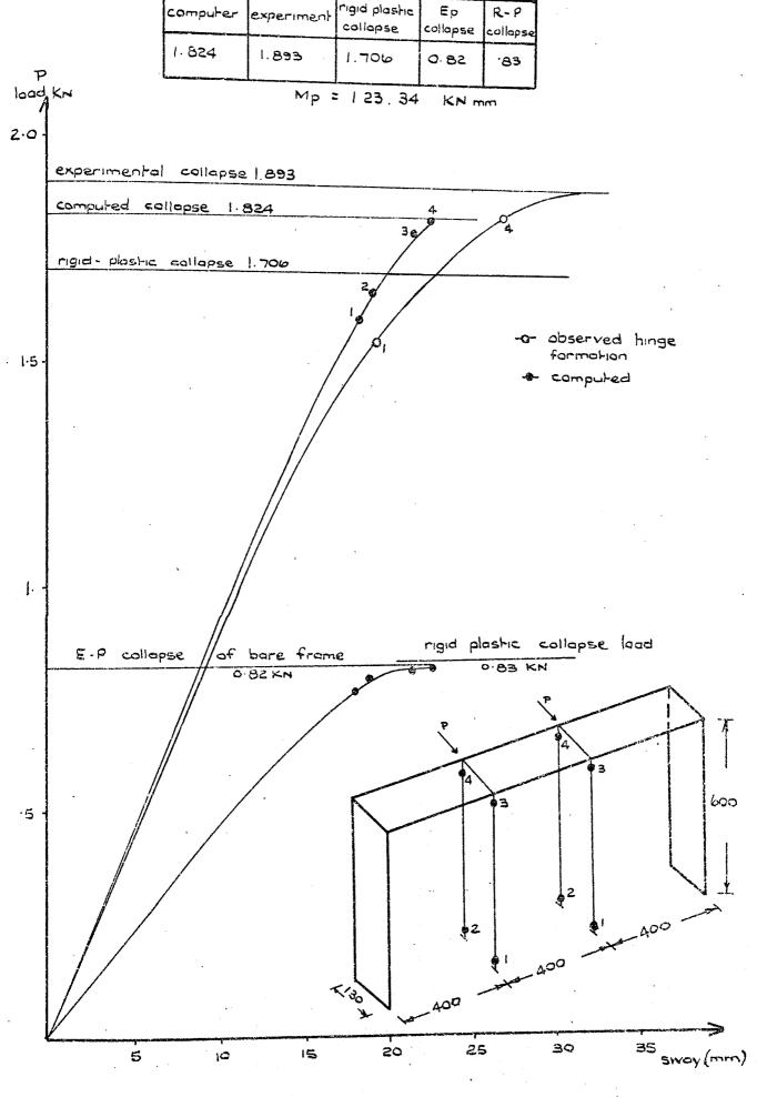
Fig 5.3. Load deflexion diagram for structure 4B
