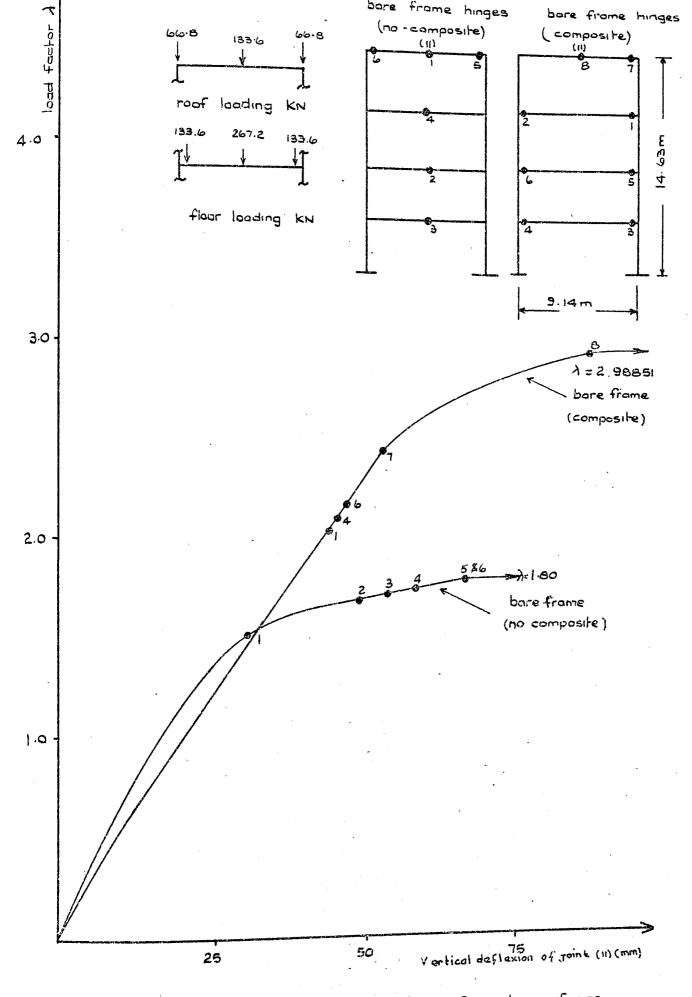
Fig. 6.2. Load deflexion graphs for a four storey frame (under vertical loading)
