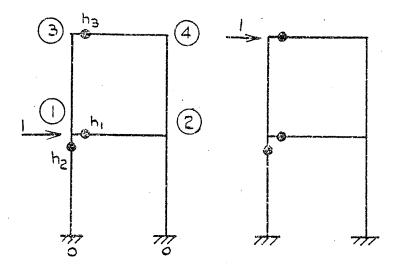
Fig. 2.4. Unit loads acting at alternative floor levels
