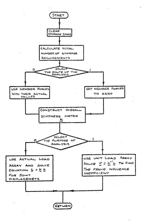
Fig. 3.2. Flow diagram for subroutine stiffmath
