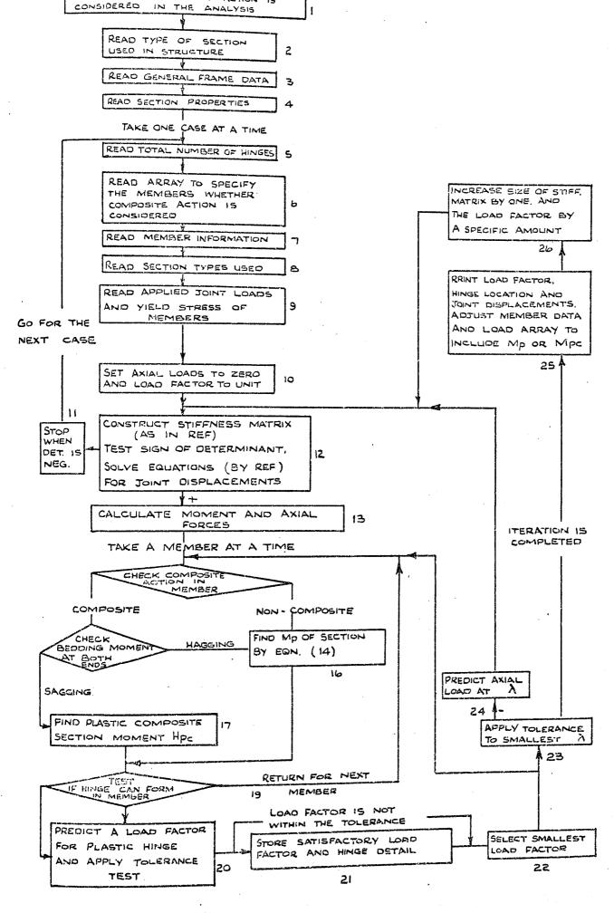
Fig. 6.1. Flow diagram for the composite action analysis programme.
