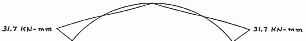
TWISTING MOMENT DIAGRAM FOR FIXED BOW GIRDER WITH VARIABLE CROSS SECTION UNDER 60.0 kgf. LOAD AT MID-POINT
