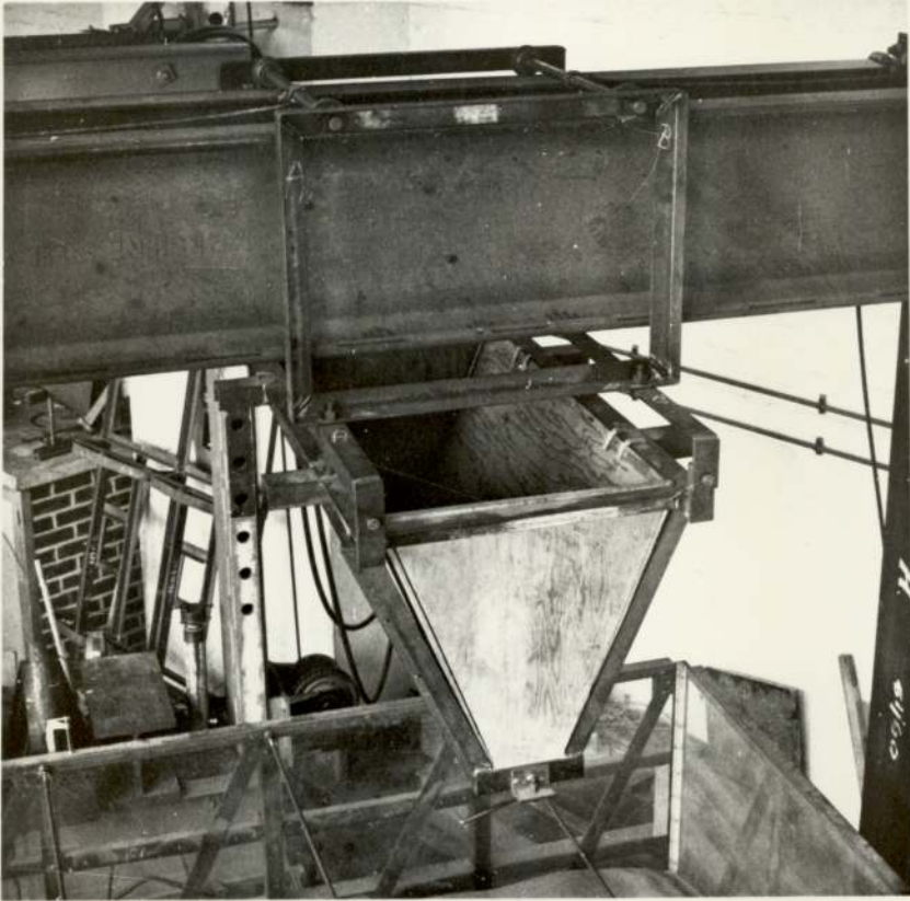
PLATE (5.2c) THE HOPPER MOUNTED ON THE TROLLEY
