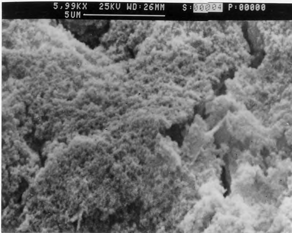
Fig.5.14 SEM picture of etched fracture surface of OPC I paste, 90 days with w/c=0.5
