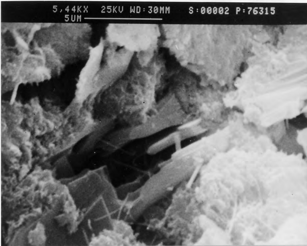
Fig.5.10 SEM picture of fracture surface of OPC I paste, 90 days with w/c=0.5
