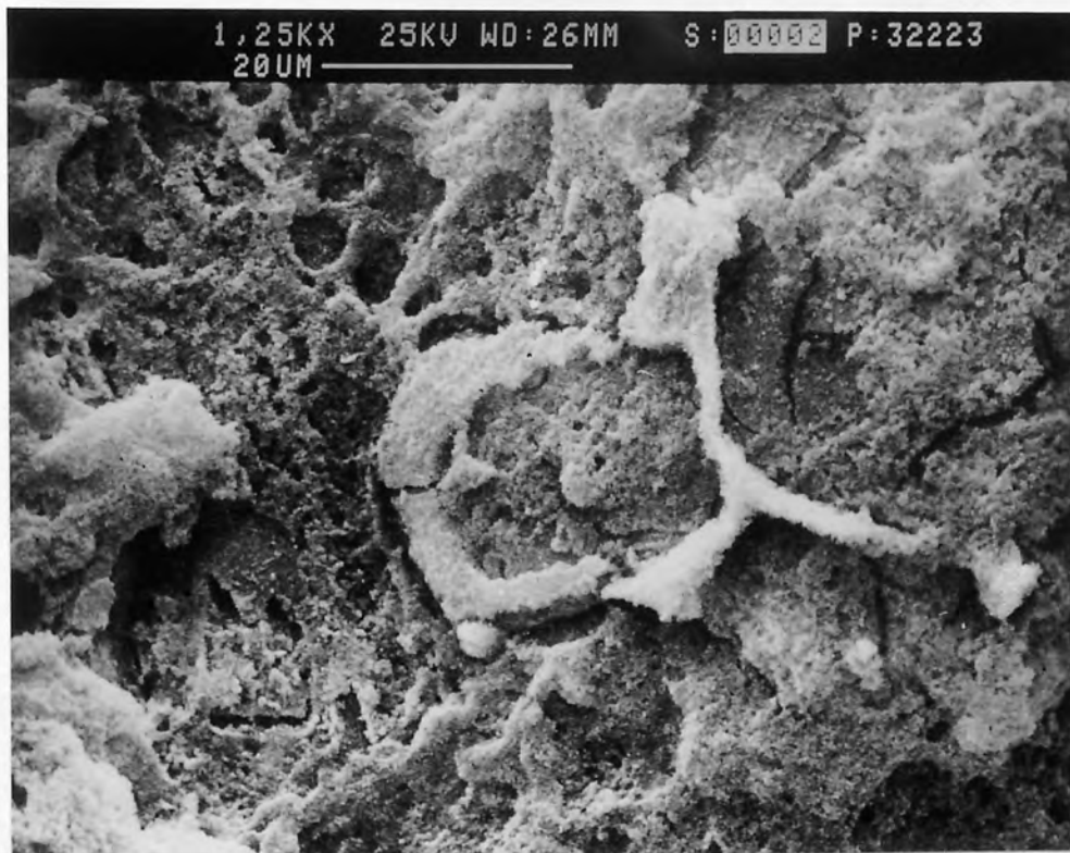
Fig.5.15 SEM picture of etched fracture surface of SBR 1-OPC I paste, 90 days with w/c=0.5
