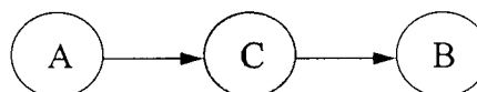
Fig. 4.7 With hard evidence at C, A and B are d-separated and independent
