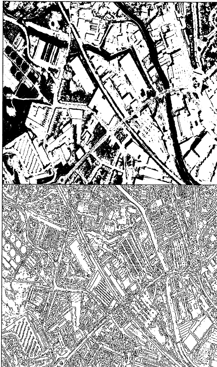
Figure 5.2 The Canny Edge Detector applied to a section of the Dudley Imagery (Band 11)
