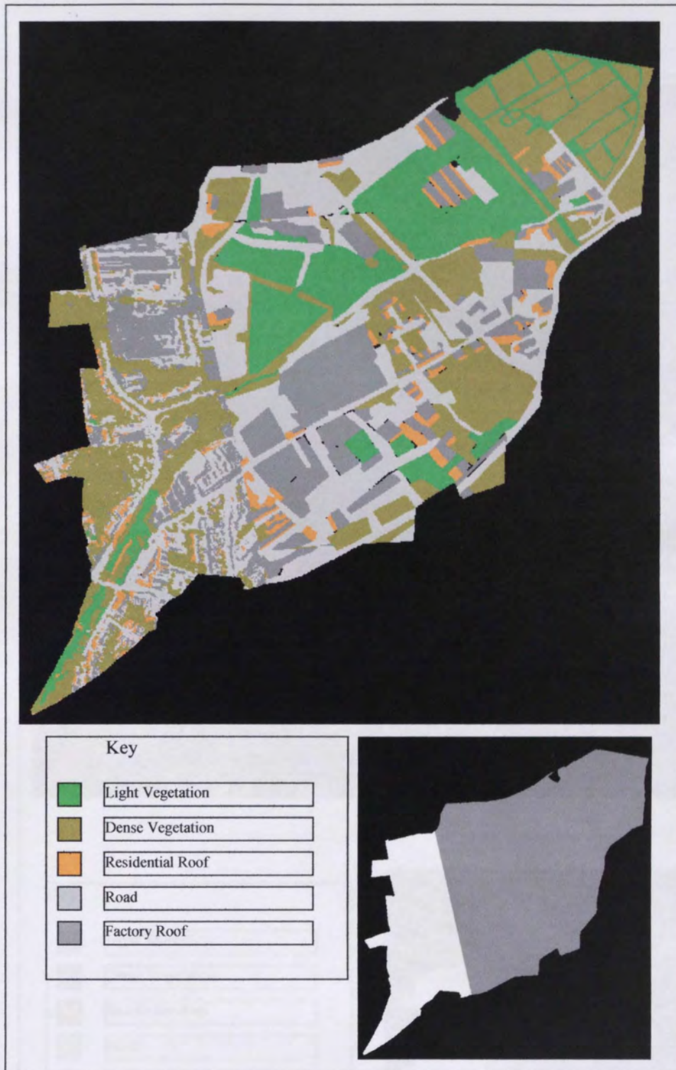
Figure 7.4 The Polygon Classified ATM Imagery overlaid on the manually classified Map of the James Bridge Catchment.
