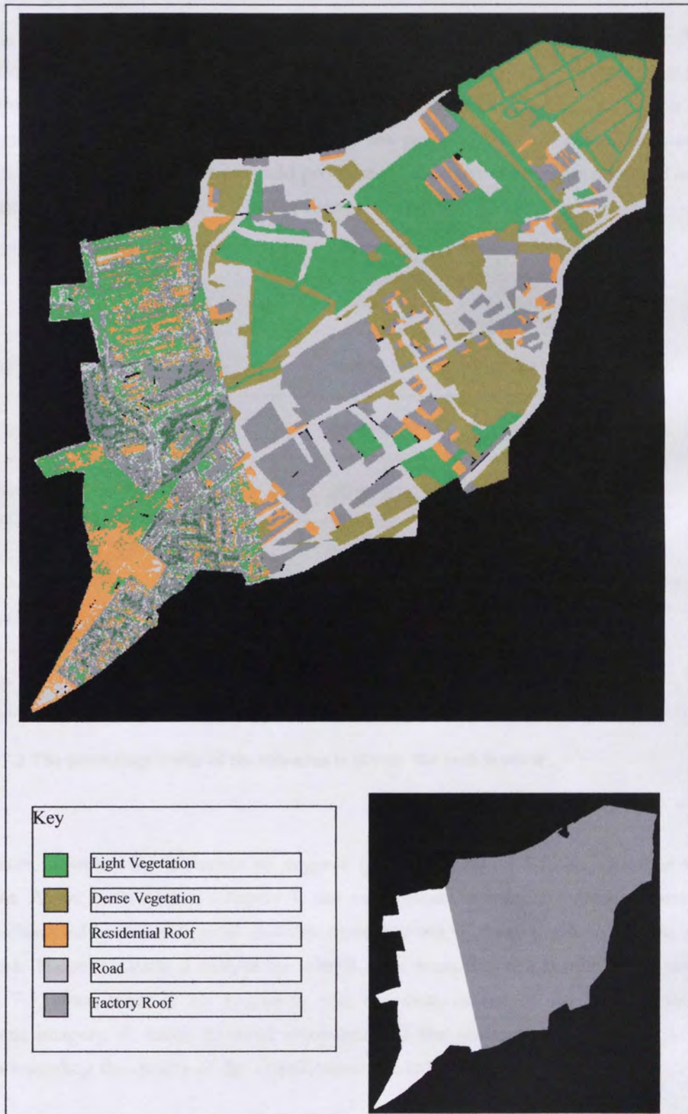
Figure 7.5 The Maximum Likelihood classification of the Vidoegrphy (Blaojovic et al , 1998) overlaid on the manually classified map.
