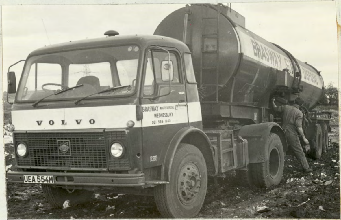
FIGURE 3.4 Articulated 4,500 gallon (20,450 litres) tanker large 14 wheel type with auxiliary engine discharging liquid waste over the face of a tip.
