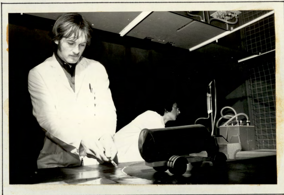
FIGURE 9.4 Detail inside the tunnel. The gas sampling technique is being demonstrated with the flow meter and helium filled bubble generator also visible.
