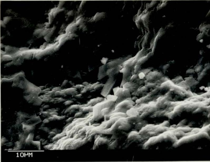
Figure 6.74 The aggregate side of the interface with a converted paste in a 20 year old HAC concrete bridge
