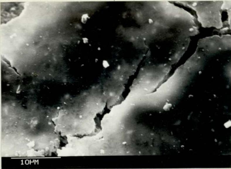
Figure 6.5 A higher magnification of the interfacial film in Figure 6.3
