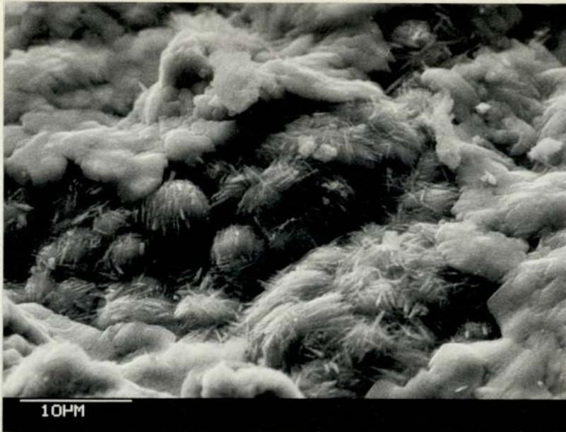
Figure 6.68 The converted paste side of the interface of a specimen from a 20 year old HAC concrete bridge
