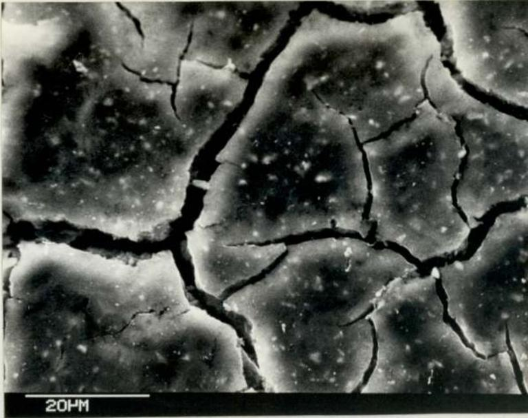
Figure 6.3 The general features of the unconverted paste side of the interface with a glass slide
