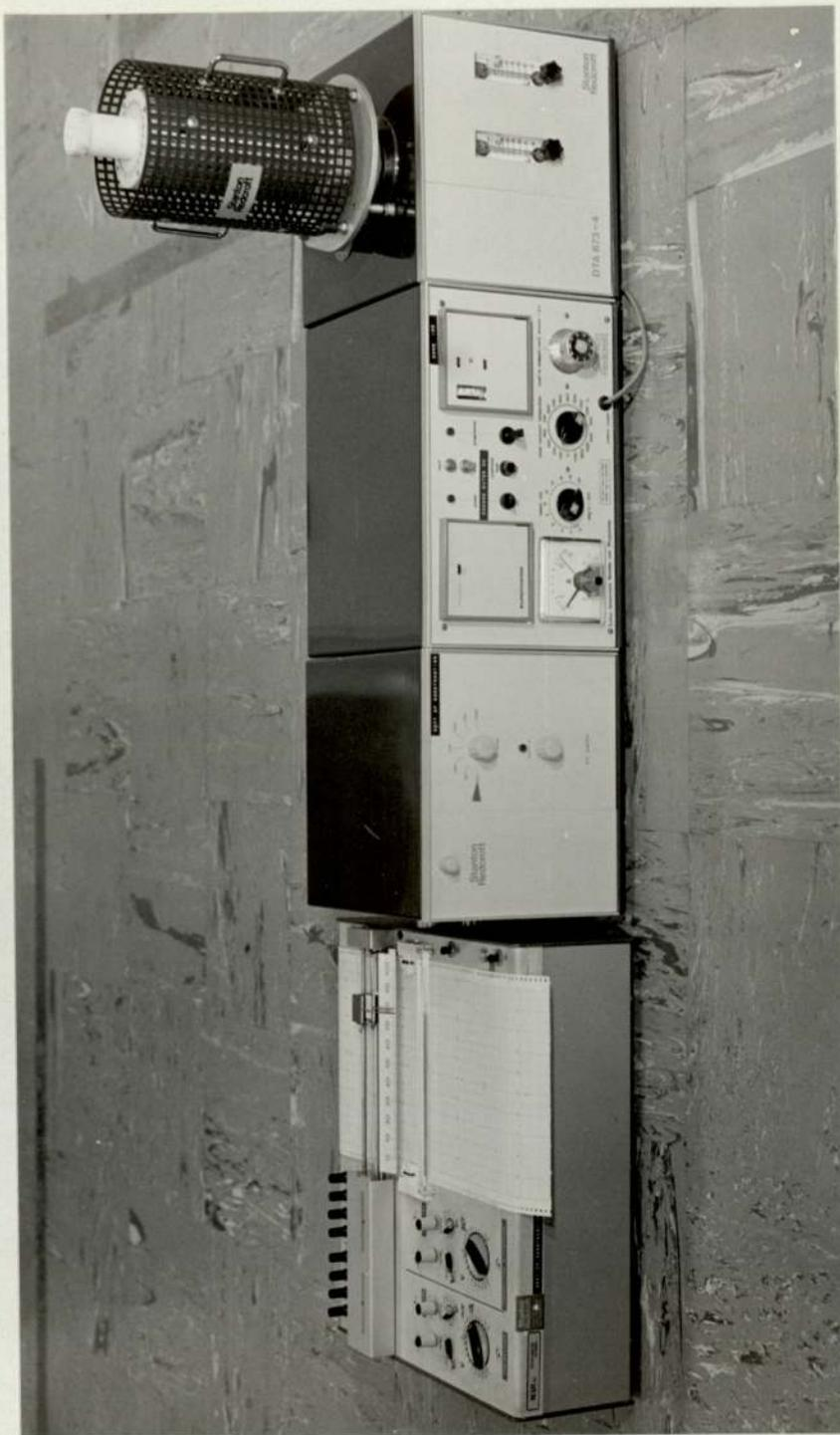
Figure 2.5 A Stanton Redcroft Differential Thermal Analyser Model 673-4
