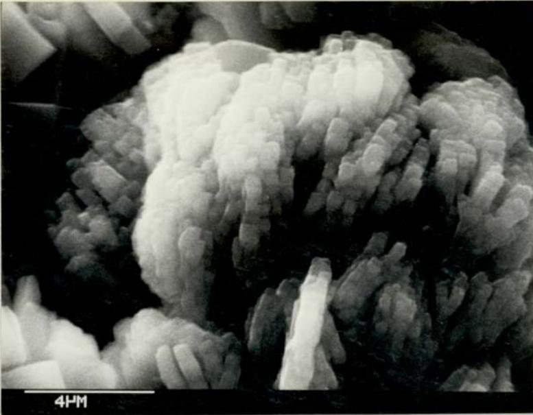
Figure 6.43 One of the shapes of gibbsite crystals on the converted paste side of the interface with Alag aggregate
