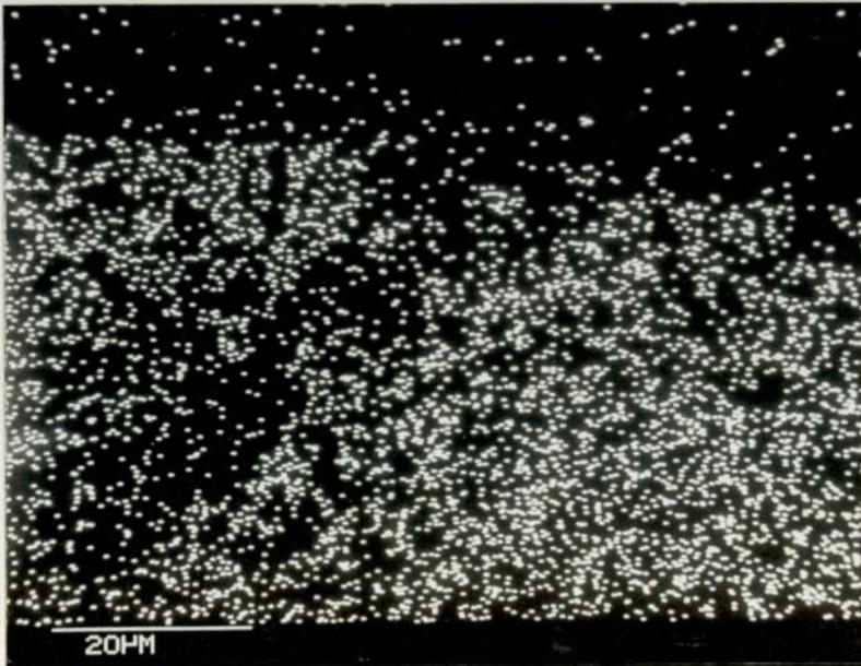
Figure 6.31 The calcium distribution for the fractured surface of Figure 6.29
