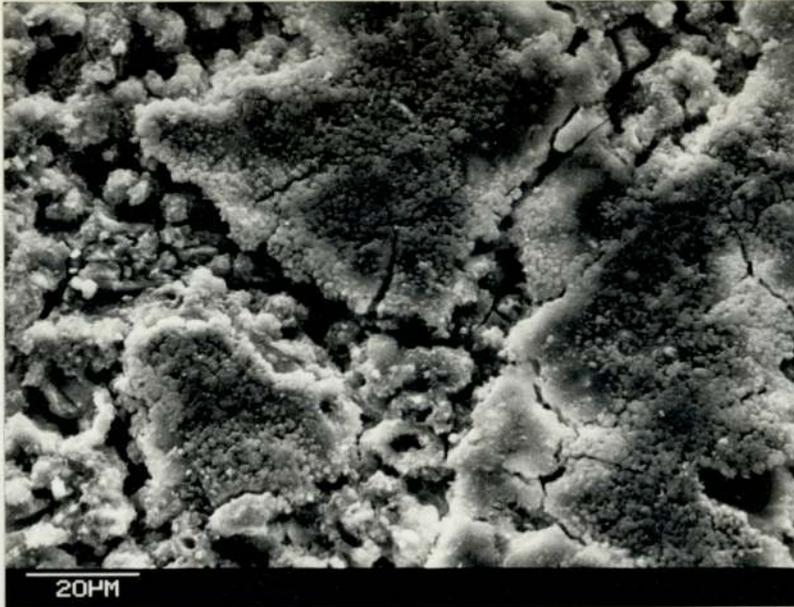
Figure 6.77 The morphology of the paste side of the interface with a glass slide after 2 days of curing at 45°C.
