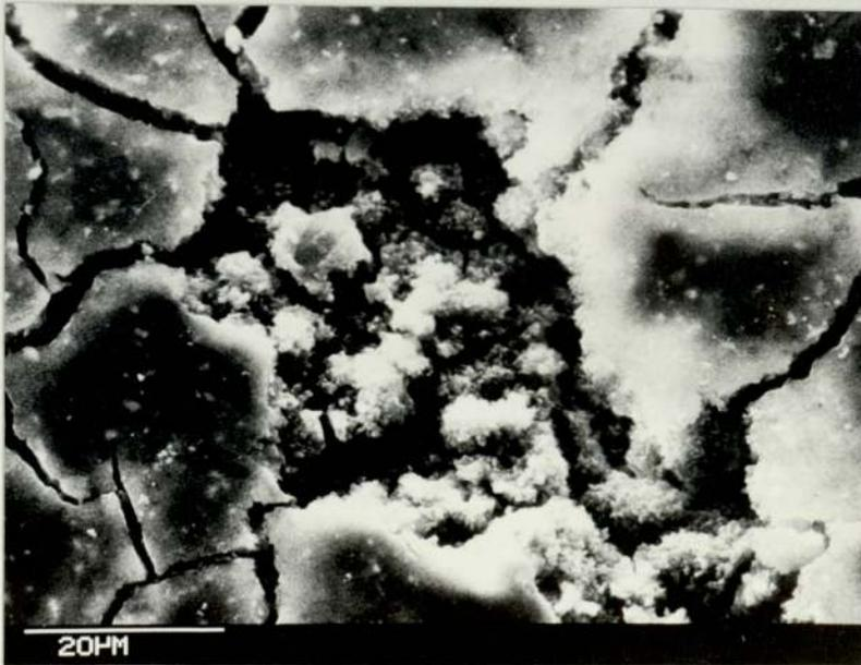
Figure 6.6 The general features of a window observed on the unconverted paste side of the interface with a glass slide
