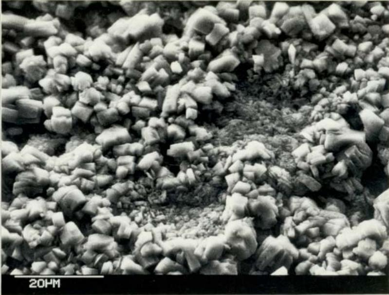
Figure 6.18 The converted paste side of the interface with a glass slide
