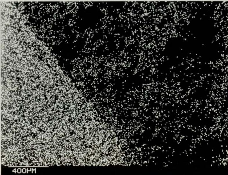
Figure 6.23 The distribution of aluminium on the two surfaces of Figure 6.22
