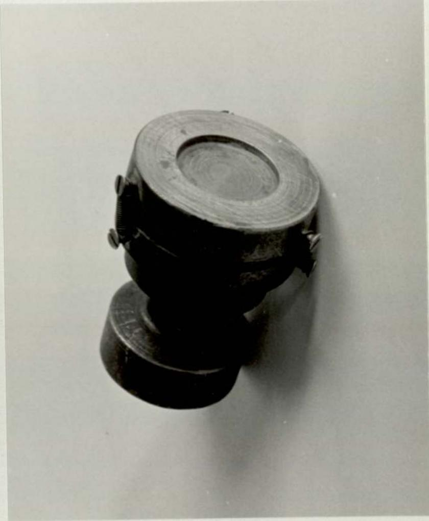
**Figure 2.4** Ball Bearing Mounted Plate for testing small Cylindrical Specimens
