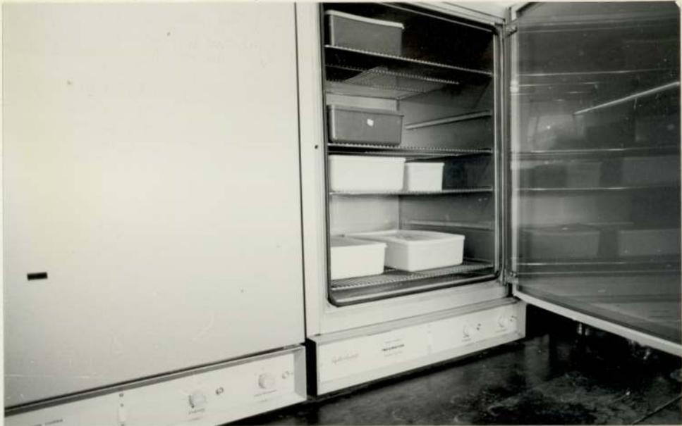
Figure 2.1 Incubator Curing
