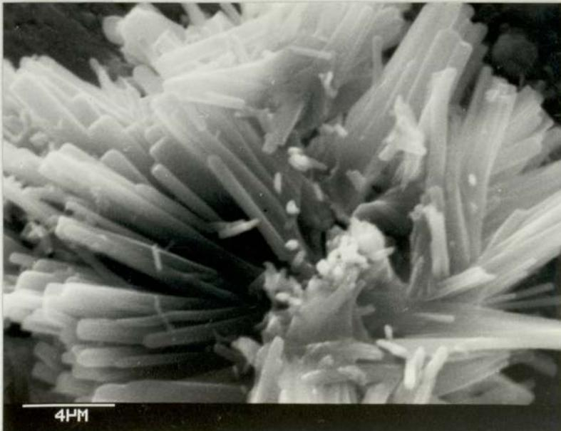
Figure 6.61 A close-up of the ettringite needles on the limestone surface
