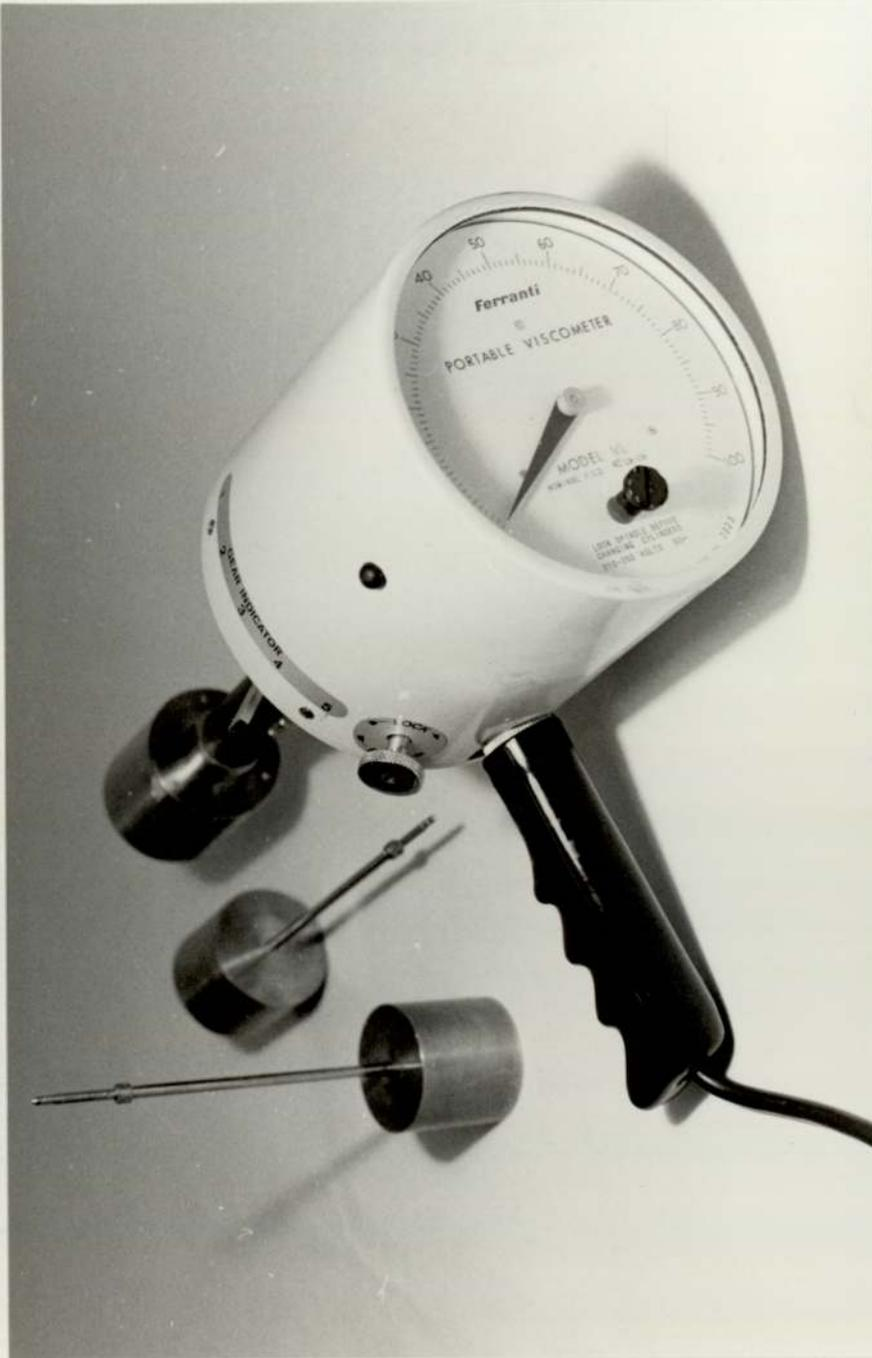
Figure 3.9 A Ferranti portable viscometer
