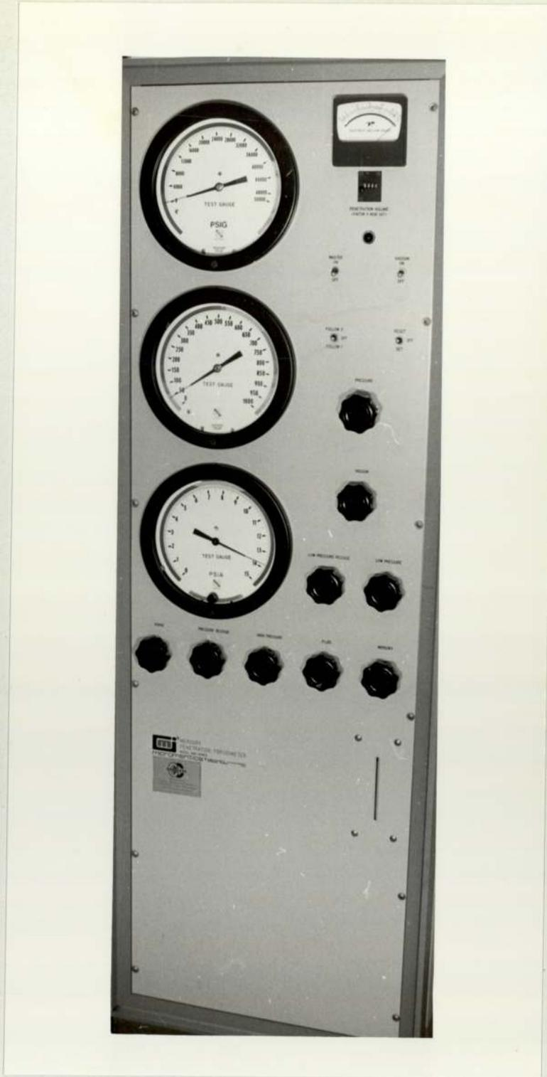
Figure 2.7 A Micromeritics instrument corporation porosimeter, Model 900/910 series
