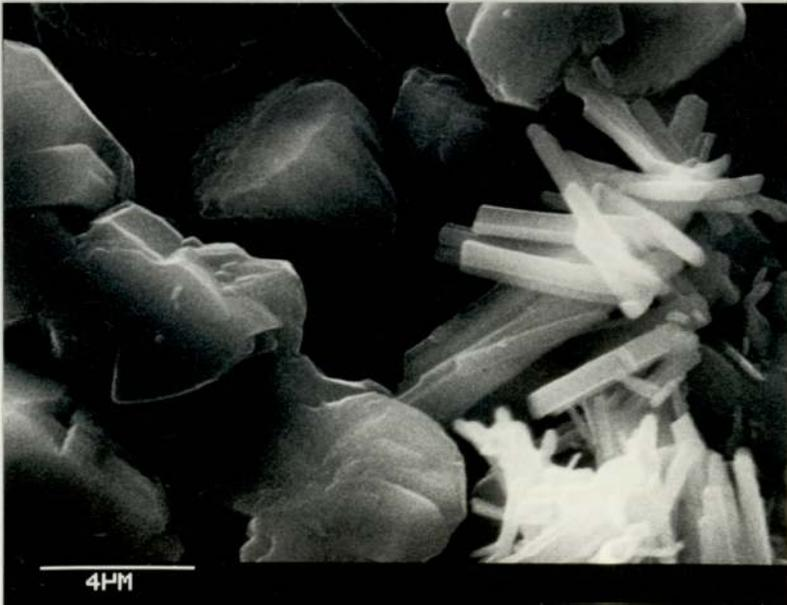
Figure 6.63 Needles of ettringite on the converted paste side of the interface with limestone
