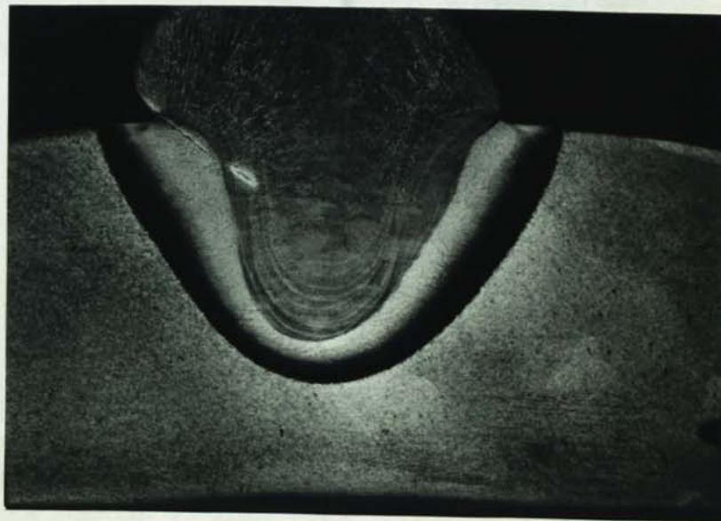
FIGURE 32 Microsection of crack in test weld S2 plate 1013.2
