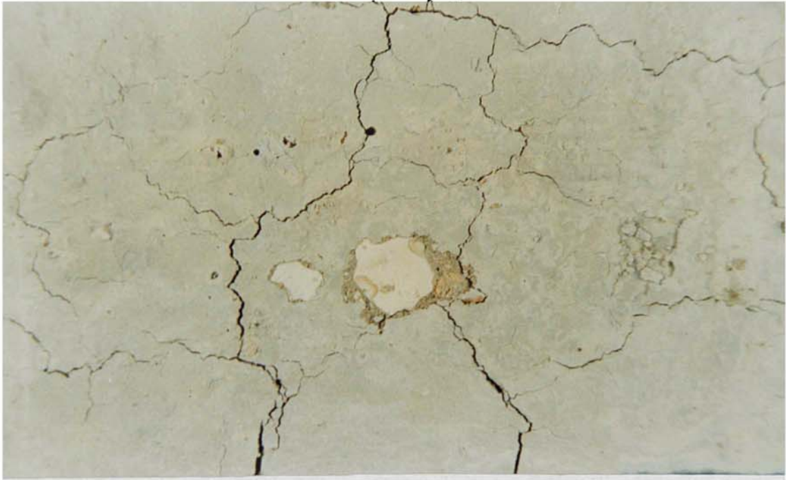
Figure 8.5(c) Photograph to show aggregate spalling on a test beam
