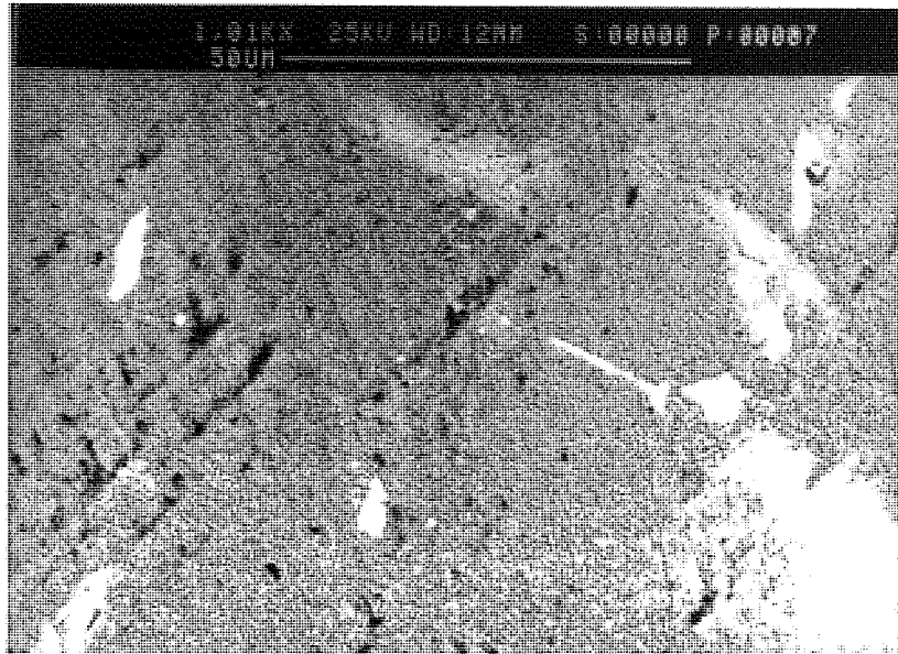
Figure 116. As cast structure of LM25 at high magnification.
