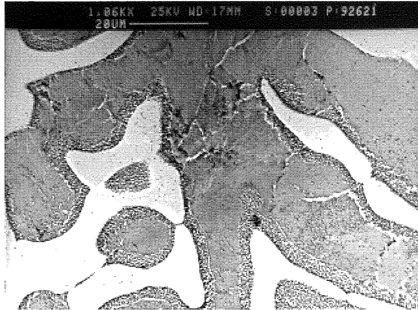
Figure 83. Alloy ZA12 tested at 100MPa and 160°C showing zinc network in \beta at high magnification
