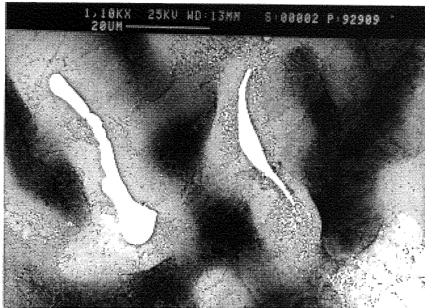
Figure 89. As cast structure of Alloy ZA27 showing the equiaxed structure of dark \alpha dendrites surrounded by lighter decomposed \beta at high magnification.
