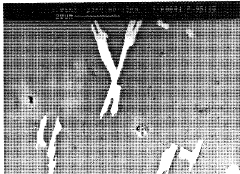
Figure 119. Micrograph of load relaxation sample of LM25 tested at 120°C at high magnification.
