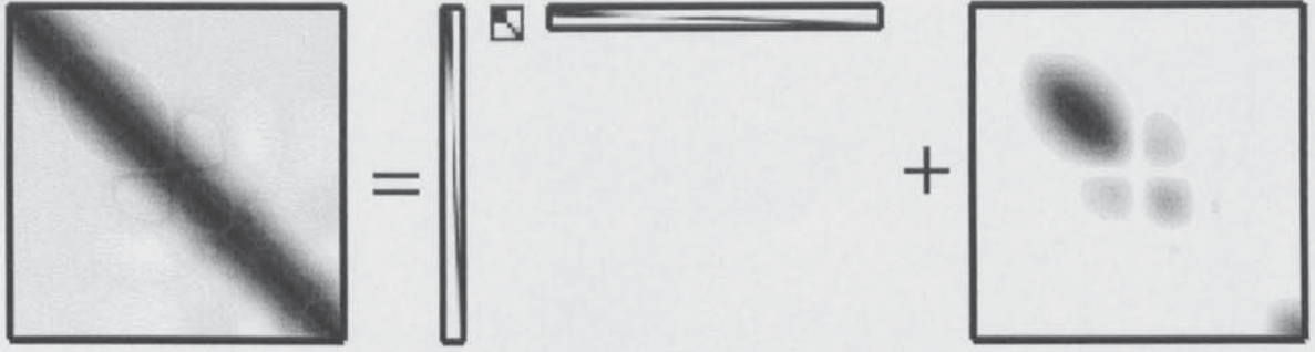
Figure 4.18: Pictorial representation of the construction of the noise free DTC covariance matrix approximation with a low-rank matrix with a space-limited covariance.
