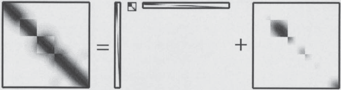
Figure 2.8: Pictorial representation of the construction of the PITS covariance matrix approximation which is identical to the DTC approximation except that an exact block diagonal structure is retained in the matrix. The block diagonal structure has fixed block sizes.
