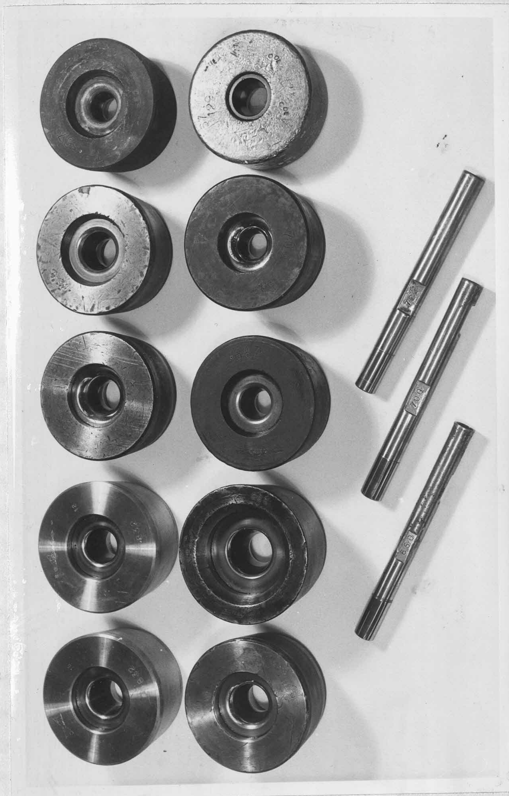
Plate (4.1) Dies and conventional plugs available for tube-drawing
