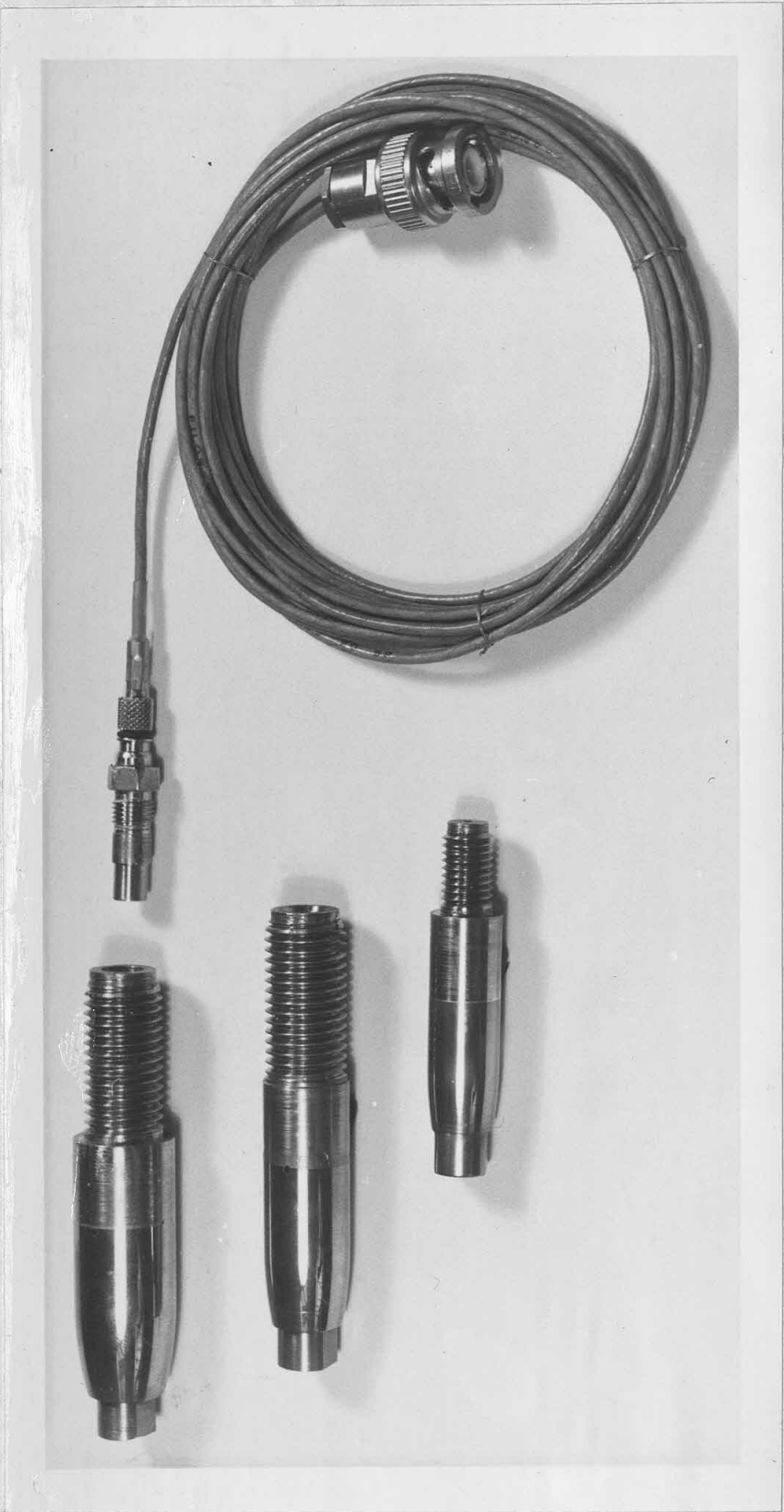
Plate (5.1) Experimental tube-drawing plugs and pressure transducer
