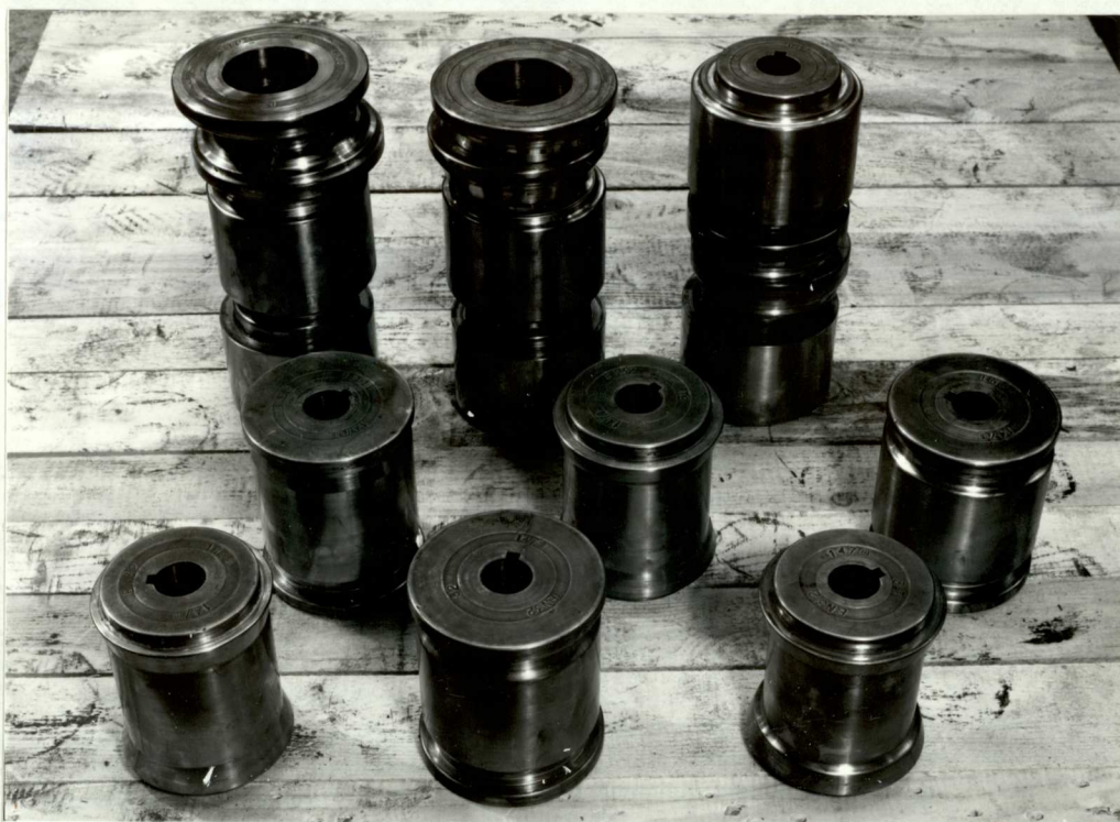
Plate 8.3 A SET OF FORM-ROLLS PRODUCED BY CNC
