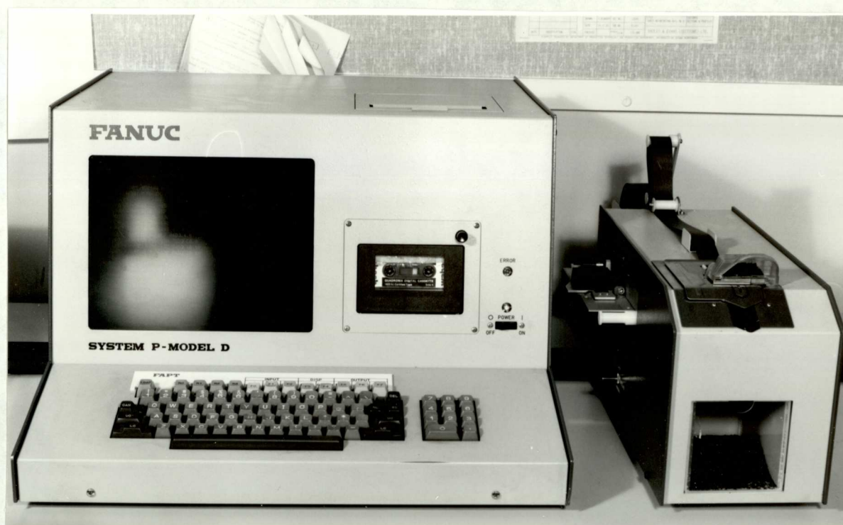
Plate 7.3 FANUC SYSTEM P MICROCOMPUTER FOR FAPT PROGRAMMING
