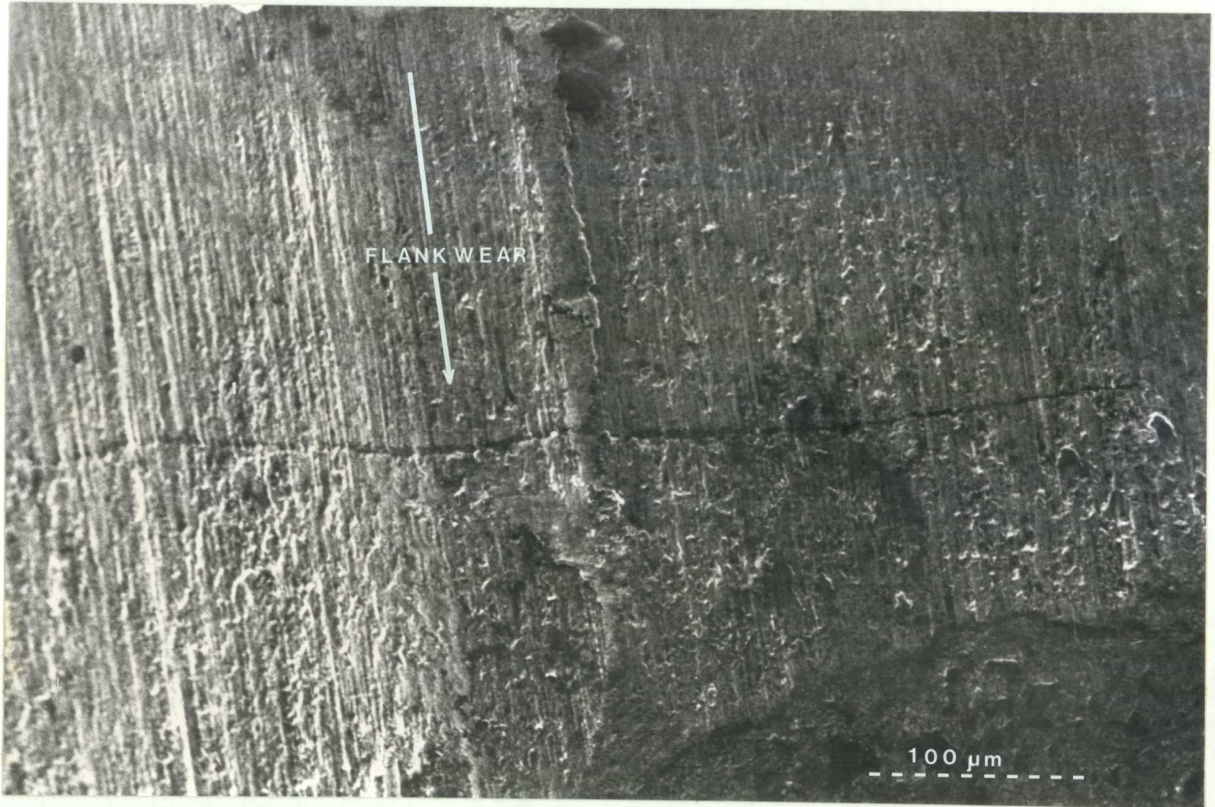
FIG 6.30 CRACK IN FLANKWEAR
