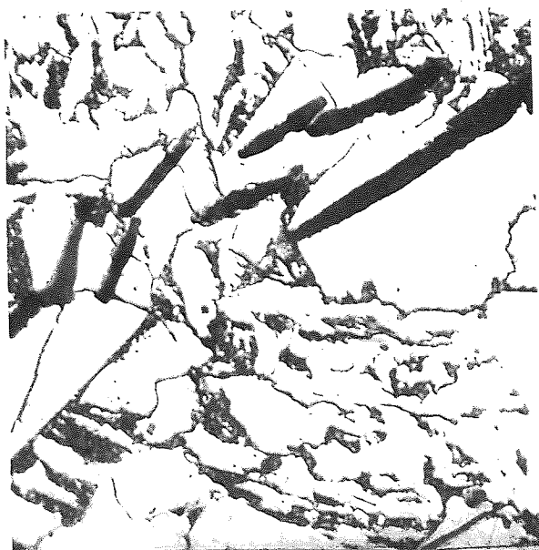
Figure 86 Simulated Sample Heat Input = 14.4KJ/mm Peak Temp. = 1250°C Nital II, X1000, Cleavage cracks cutting across the proeutectoid ferrite and changing direction at the cells boundaries.
