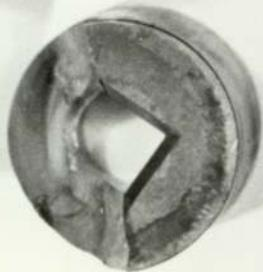
PLATE 8.3. Square section drawing dies (shape 'B')
