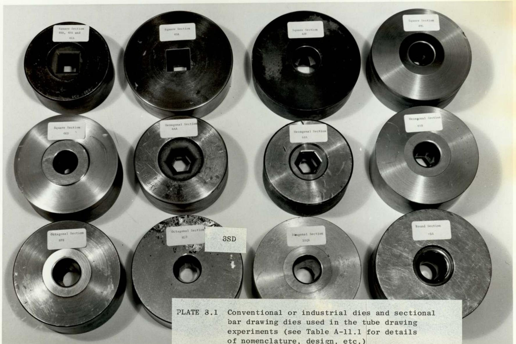
PLATE 3.1 Conventional or industrial dies and sectional bar drawing dies used in the tube drawing experiments (see Table A-11.1 for details of nomenclature, design, etc.)
