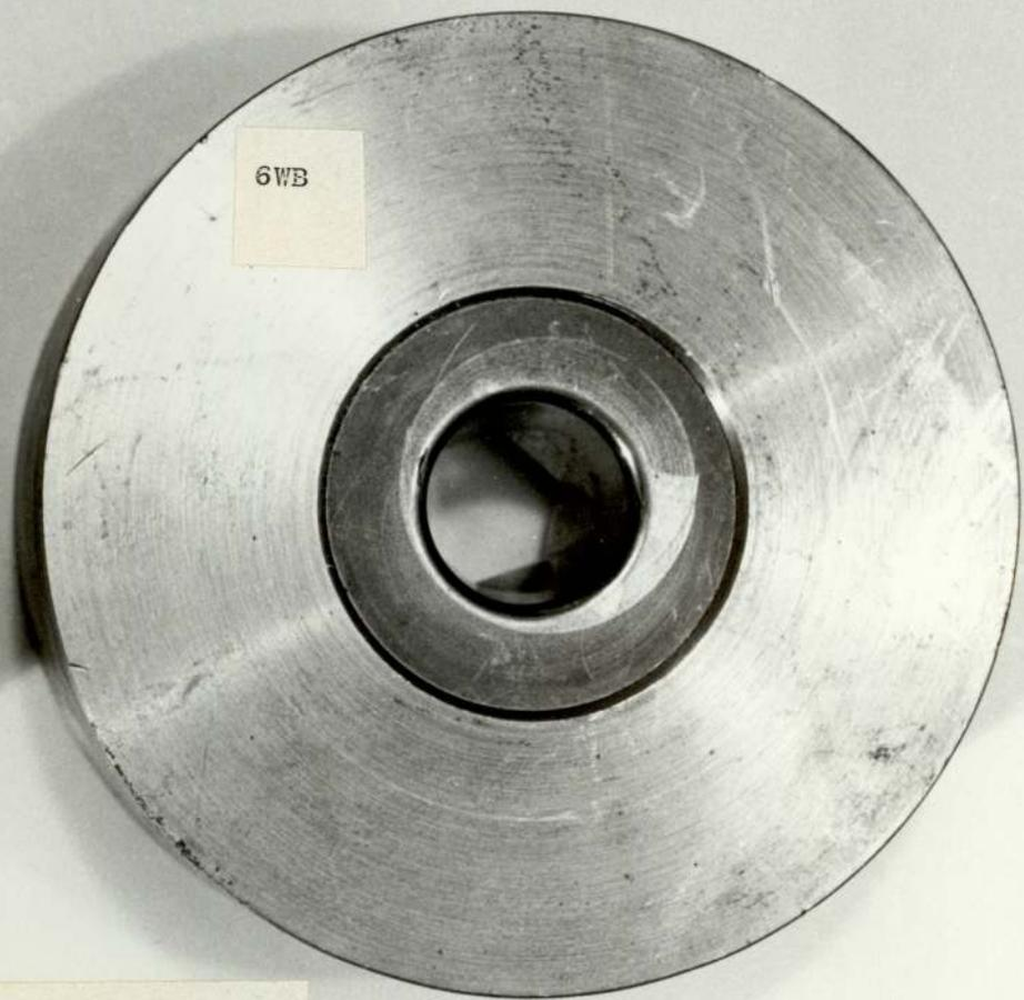
PLATE 8.4 Hexagonal (6WB) and octagonal (8WB) elliptical tube drawing dies
