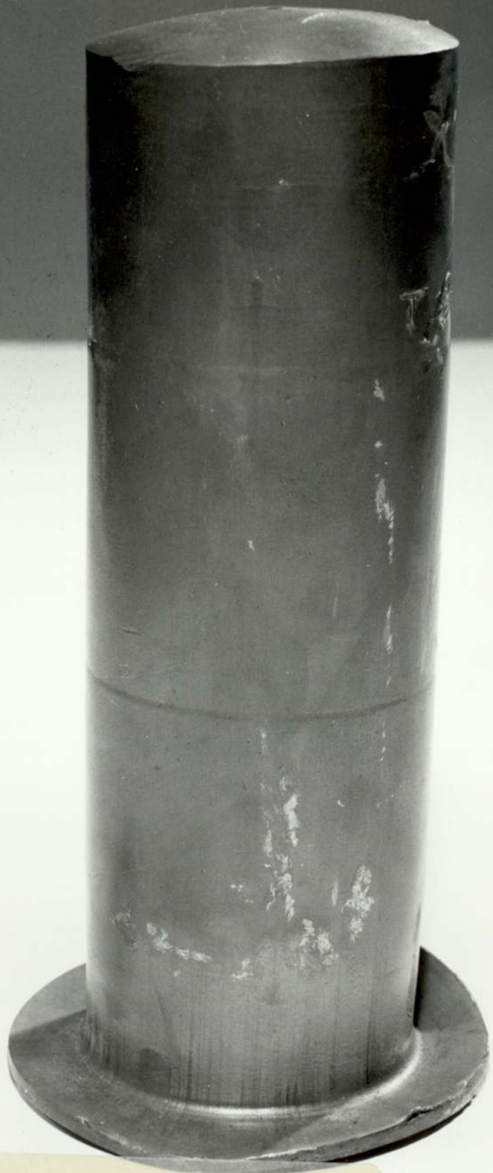
FIG. 5.3. SLOW SPEED EXTRUSION OF LEAD, 75 mm DIAMETER, 75 mm LONG BILLET- 50% REDUCTION OF AREA
