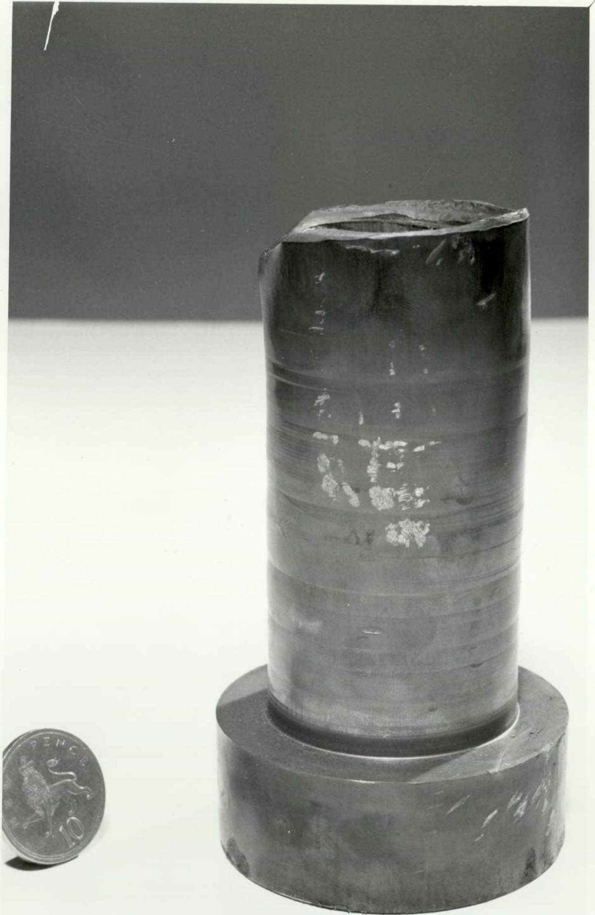
FIG. 5.6. IMPACT EXTRUSION OF LEAD - 75 mm DIAMETER, 75 mm LONG BILLET - 50% REDUCTION OF AREA, TEST 16 to 21
