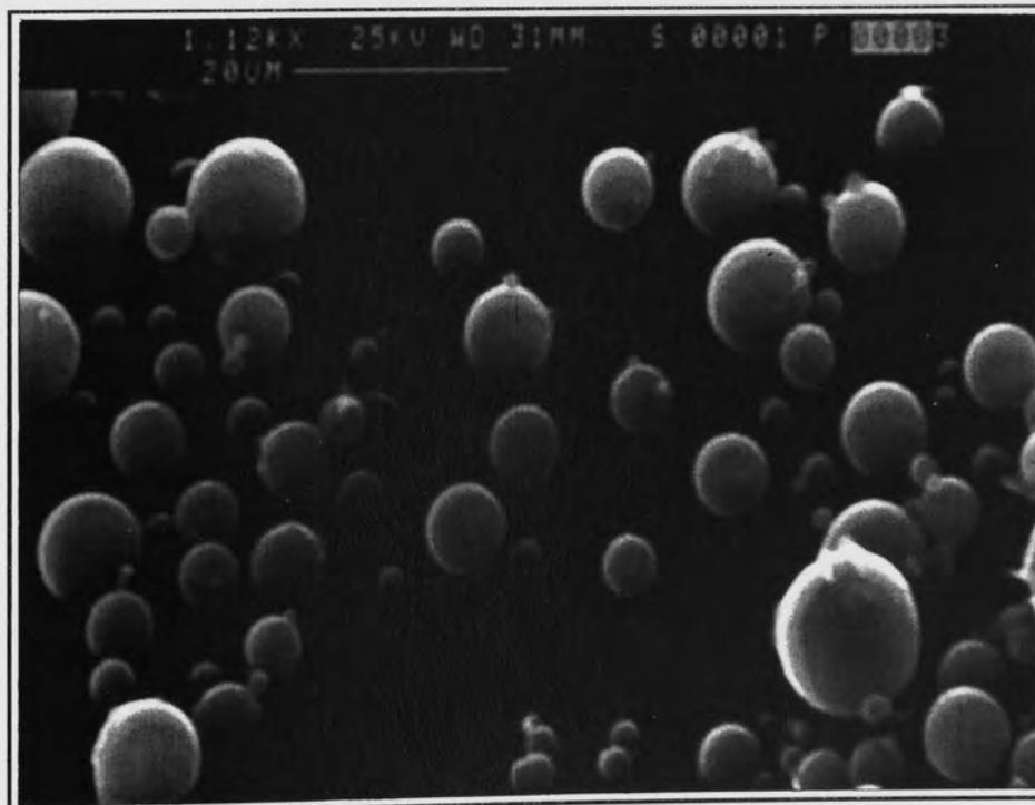
Figure 2.4 - Scanning electron micrograph of PLGA (90:10) microspheres. Mean particle size =  $3.9 \mu\text{m}$ ;  $\sigma_g = 1.7$  ( $n = 97$  particles).
