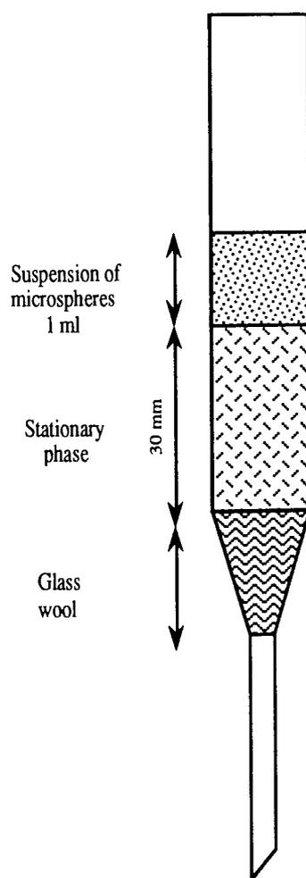
**Figure 4.1** - Diagram of a HIC column prepared using a glass Pasteur pipette as described in the text.
