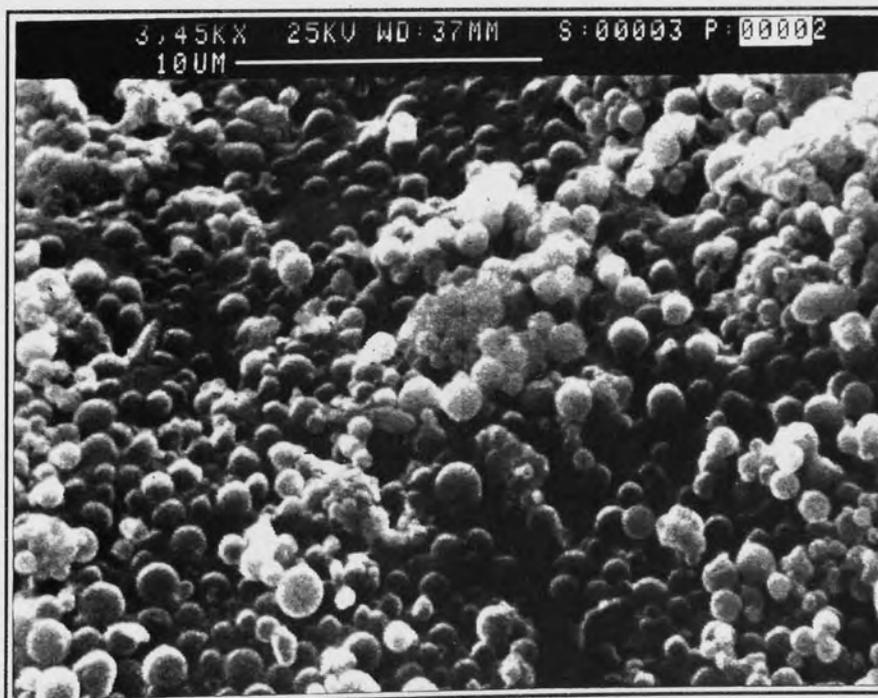
Figure 2.10 - Scanning electron micrograph of a PLA (Mwt 2000 Da) batch of microspheres containing TT microencapsulated.
