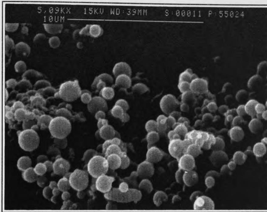
**Figure 2.5** - Scanning electron micrograph of PLA (Mwt 2000 Da) microspheres prepared according to method D, using a high speed homogeniser ( $\geq 10000$  rpm).
