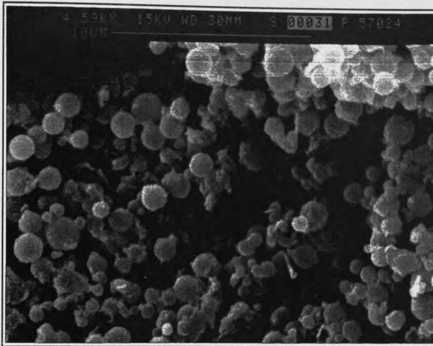
Figure 2.9 - Scanning electron micrograph of a PLA (Mwt 2000 Da) batch of microspheres containing BSA microencapsulated.
