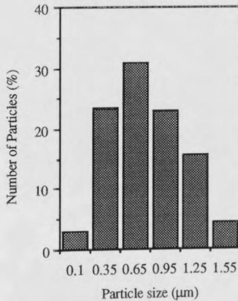
**Figure 2.6** - Particle size distribution of PLA (Mwt 2000 Da) microspheres prepared by method D using a high speed homogeniser ( $\geq 10000$  rpm). Mean particle size =  $0.7 \mu\text{m}$ ;  $\sigma_g = 1.8$  ( $n = 231$  particles).
