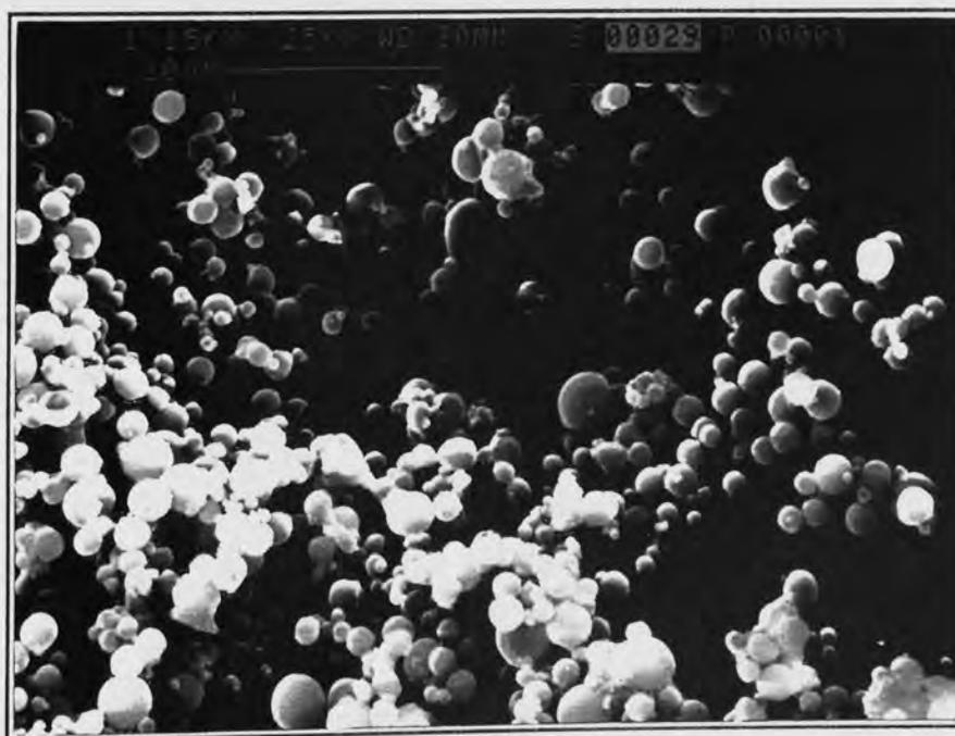
**Figure 2.7** - Scanning electron micrograph of PLA (Mwt 50000 Da) microspheres prepared according to method D.
